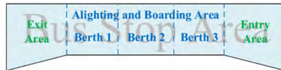
FIGURE 3. Structure of bus stop
