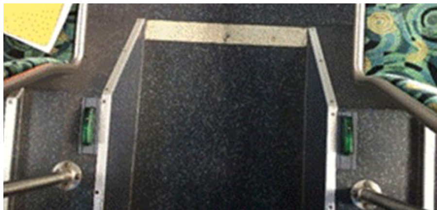
FIGURE 4. Accelerometer placement on longitudinal axis of bus
