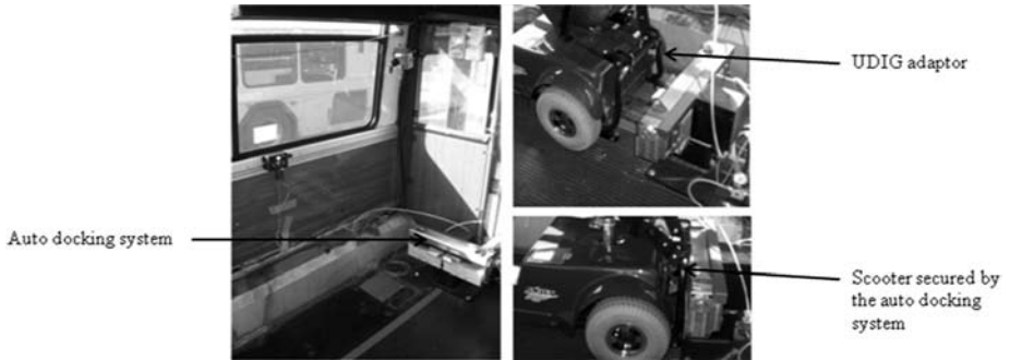
Figure 3. Auto docking system installed in LATV (left); scooter equipped with UDIG adaptor, backed into and secured by auto docking system
