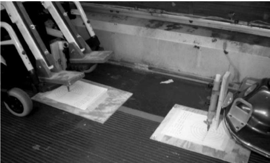
Figure 7. Spring-loaded pens and targets used for recording displacements of wheelchairs
