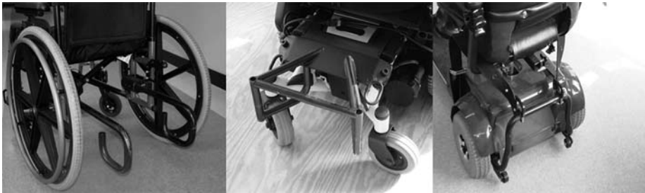
Figure 2. UDIGs attached to manual wheelchair (left), powered wheelchair (middle), and scooter (right)
