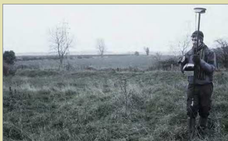
(a) Using a differential GPS unit for precise mapping of contours
