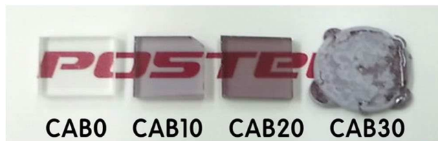
Figure 1. Photographs of calcium aluminoborate specimens with 0–30 mol% of Nd 2 O 3 .
