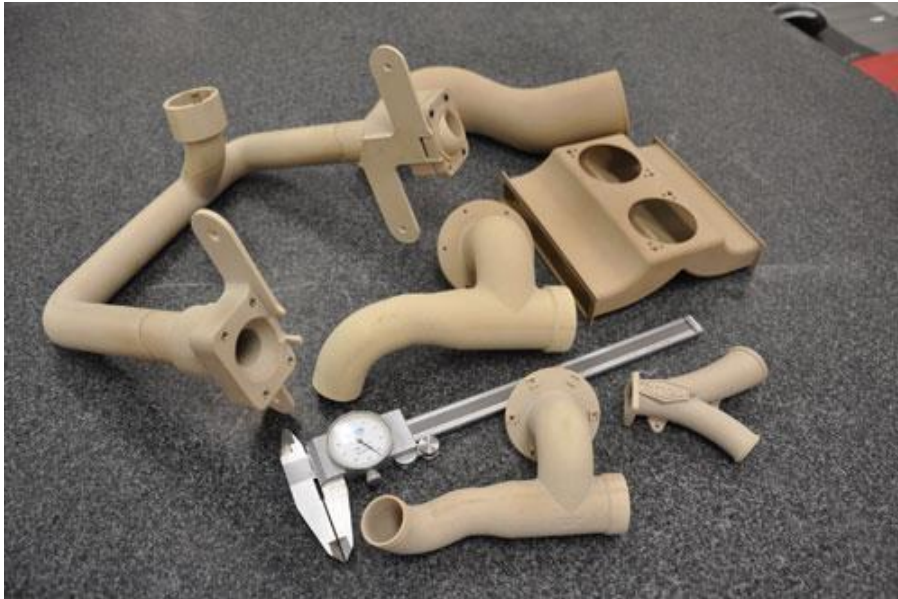
Fig 1.7: Cooling ducts for the F/A-18E/F Super Hornet manufactured from Duraform PA, produced using SLS (Hopkinson et al. , 2006)
