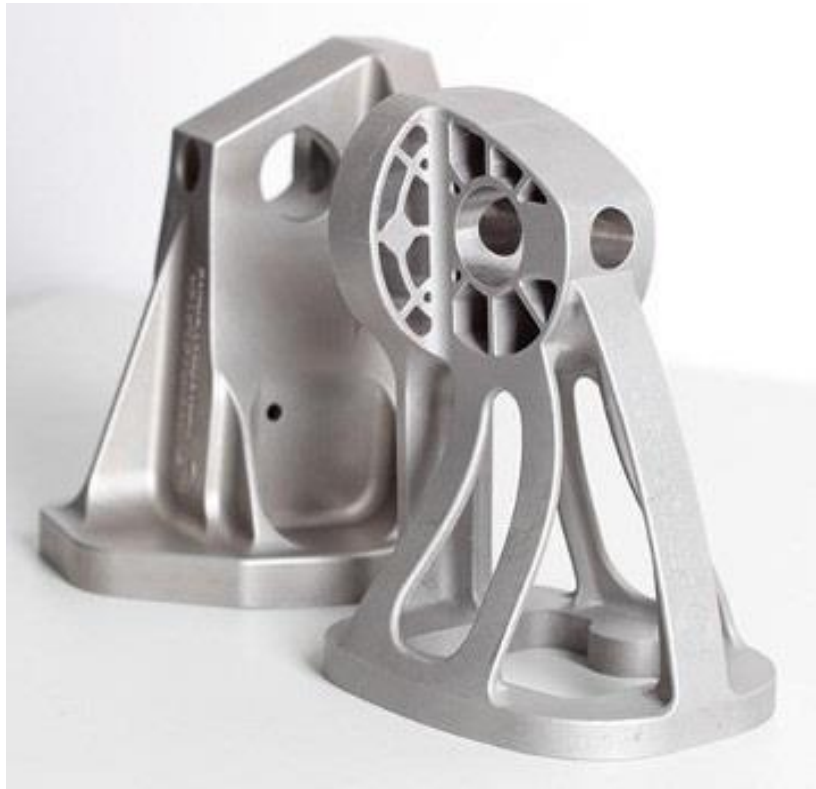
Fig 1.8: Typical AM parts of an optimised Airbus A380 bracket made of stainless-steel powder (Thompson et al. , 2016)
