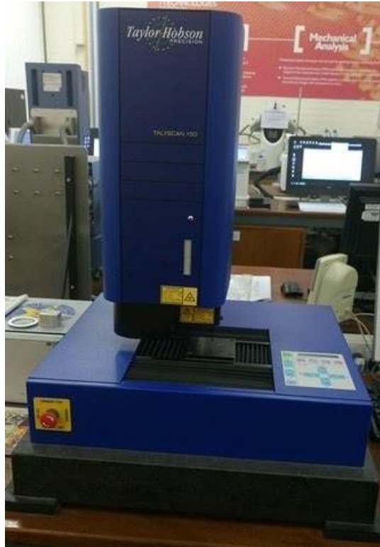
Fig 4.8: The Talyscan-150 surface roughness measurement equipment (at Exeter University).
