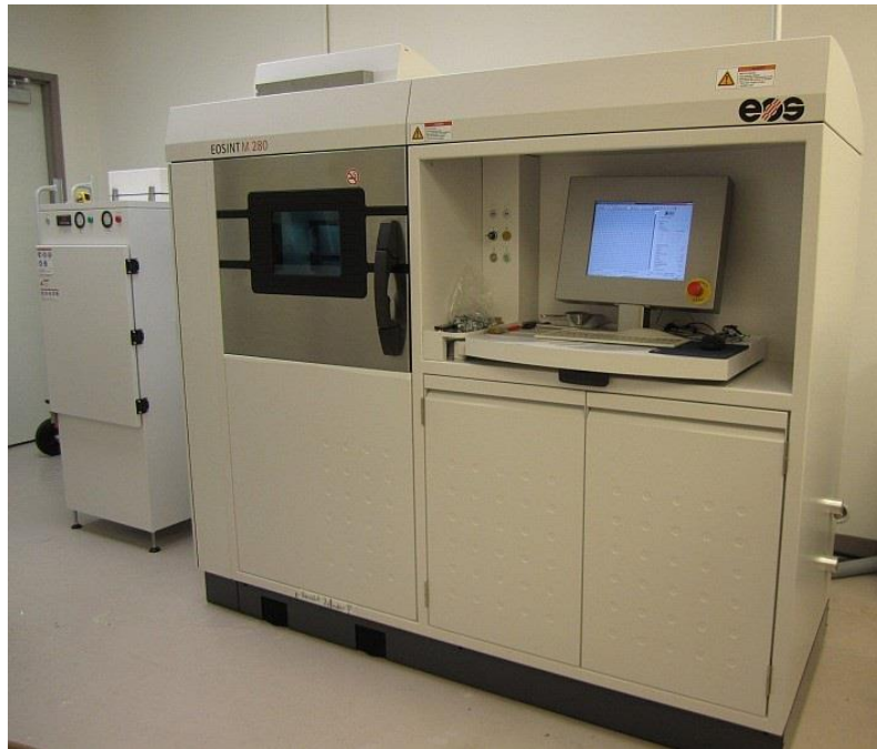
Fig 4.3: The DMLS machine at Chongqing University
