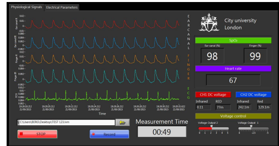
Fig. 7. Front panel of the virtual instrument (VI) showing the continuous display of AC PPG signals, the ECG signal (green). The SpO 2 values are also displayed on the right of the VI.
