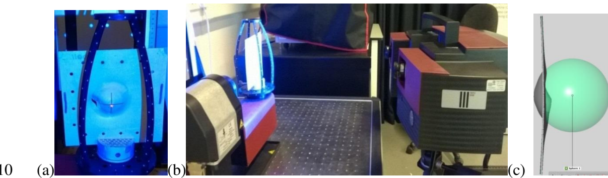
10 (a) (b) (c) 11 Figure 10: 3D scanning; (a) Formed part in scanning frame, (b) Part being scanned, (c) 12 Scanned geometry centered.
