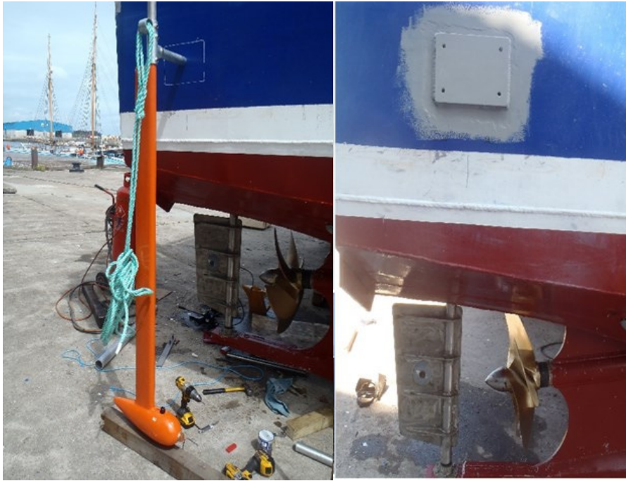
Figure 7 Attachment of the Hydropod to the vessel during drydock for underwater camera adjustment.
