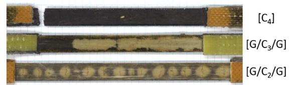
Figure 5. In-plane view of aligned discontinuous fiber and interlaminated specimens.
