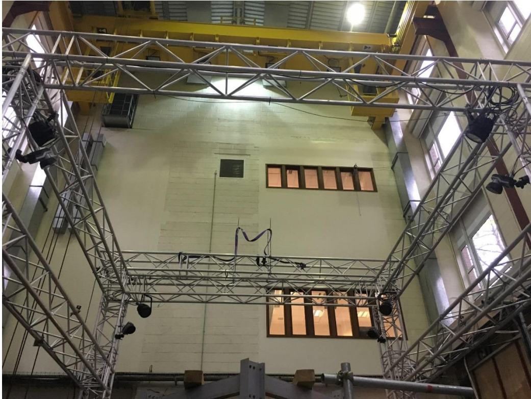
Figure 6. High speed video system and infrared vision system in each corner of the surrounding frame
