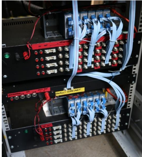
Figure 10. End of column hardware that distributes power and timing signals to the strings of
