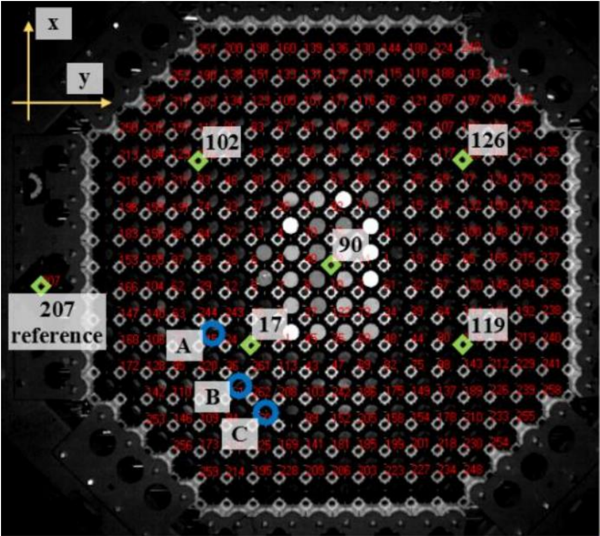
Figure 7: Location of the reference point (207), CoD bricks (A, B, C), monitored interstitial bricks (17, 102, 119, 126) and the table axes
