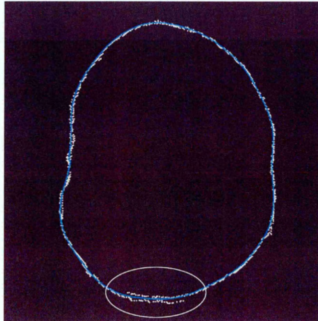
Figure 7.11 – A cross sectional point cloud slice showing participant movement during the scanning duration
