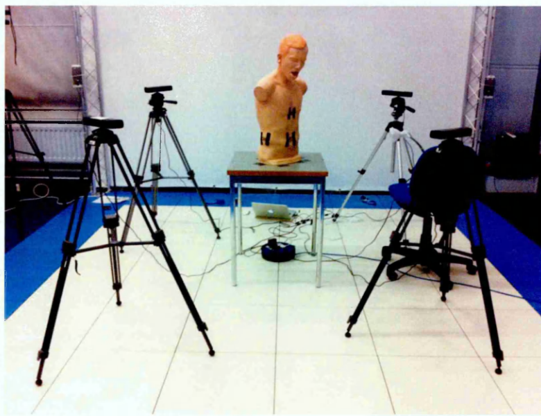
Figure 3.19 – Setup of the Kinect for calibration using the 3D spheres technique
