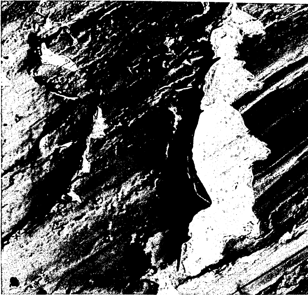
PLATE 4: MICROCRACK CONTRAST SEQUENCE SHOWING THE MIDDLE GREY BAND ASSOCIATED WITH POOR PENETRATION OF REPLICATING MATERIAL AND WITH THE COLLAPSE PHENOMENON
