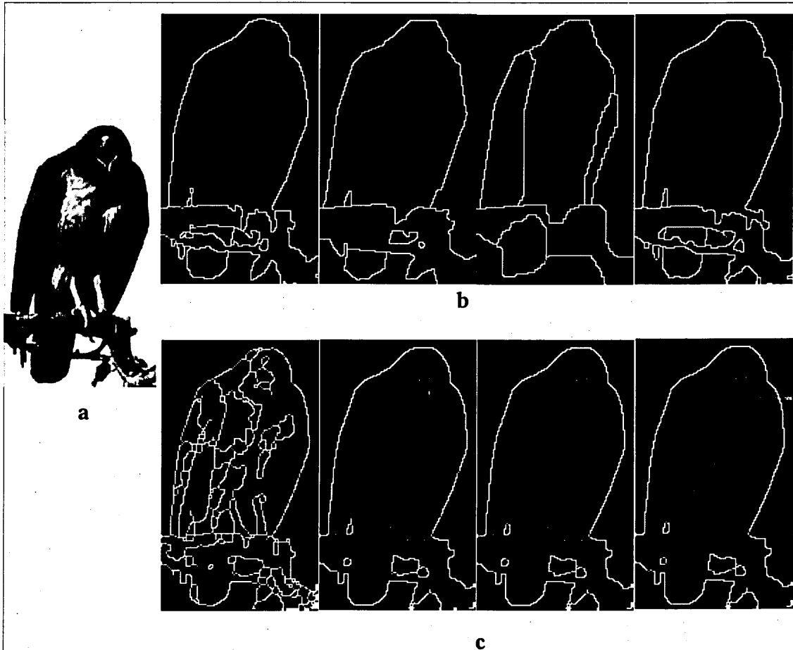
Figure 3.10 - HCS process segmented boundaries of a natural scene. A natural scene from the Berkley database (subset of Image ID 42049) (a). Top row of images are boundaries, marked by four different human subjects (b). Bottom row of thinned boundary images are the HCS process segmentation output when there were 22, 15, 10 and 6 regions (c). (Image courtesy Selvan Sept. 2011)
