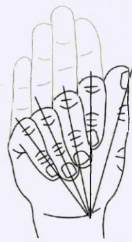
Figure 2.4: Effect of inclination of interphalangeal joints (Grebenstein, 2012)
