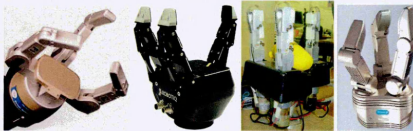
Figure 3.5: From left: Barrett Hand, Robotiq adaptive gripper, LARM hand, and SCHUNK Dexterous Hand
