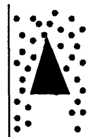
Figure 4.14(a). Side view for stratified (2) flow
