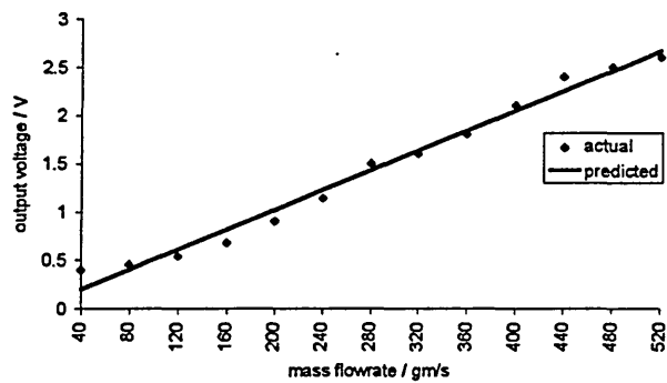
Figure 5.4 Relationship between mass flow rate and optical sensor output voltage for optical fibre receiver number twenty five
