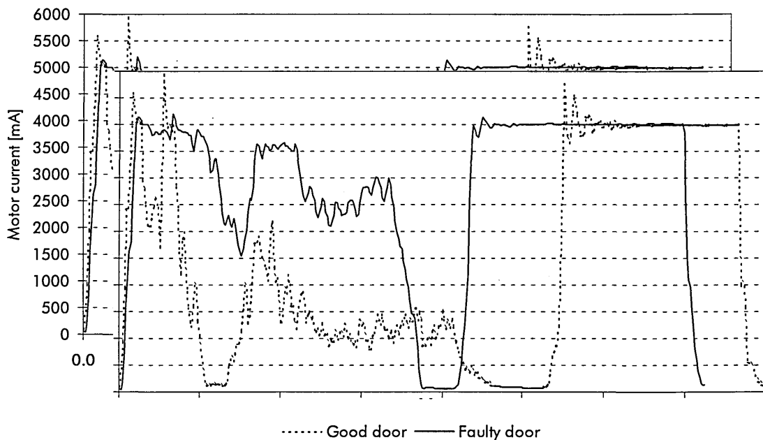
Figure 5f: Example faulty door motor characteristic 1
