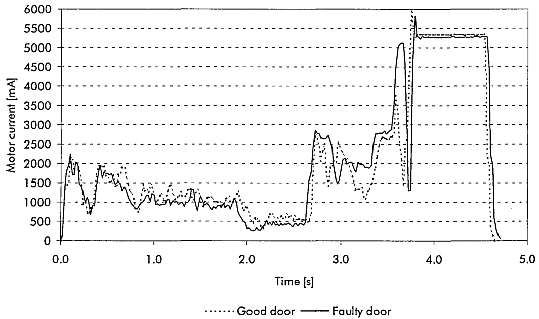
Figure 5h: Example faulty door motor characteristic 3
