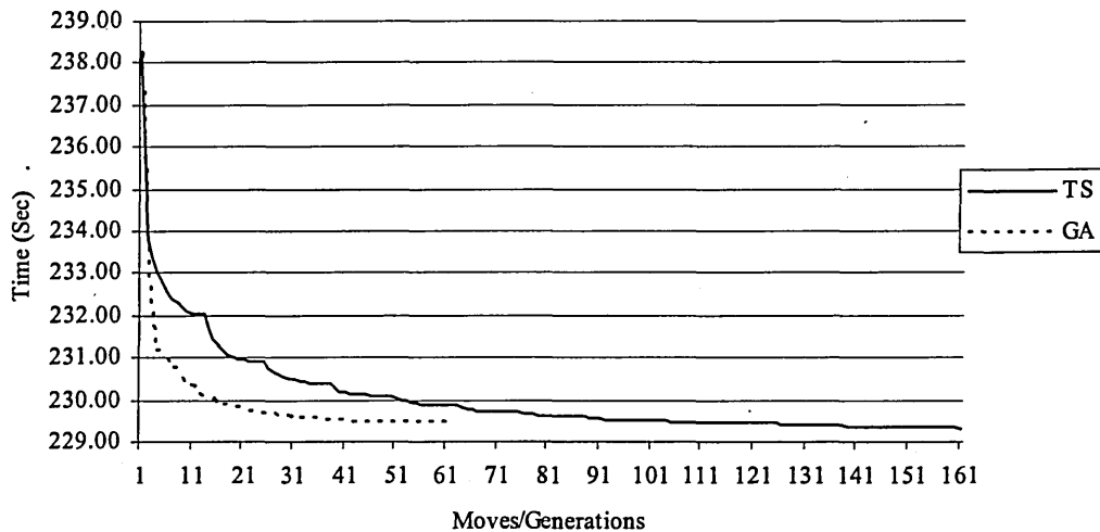
Figure 4.14. The relationship between processing time and number of moves/generations for board type A
