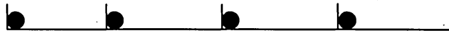
Figure 7.1: Schematic of systematic sampling (take the 1 st member of each n-packet bucket).
