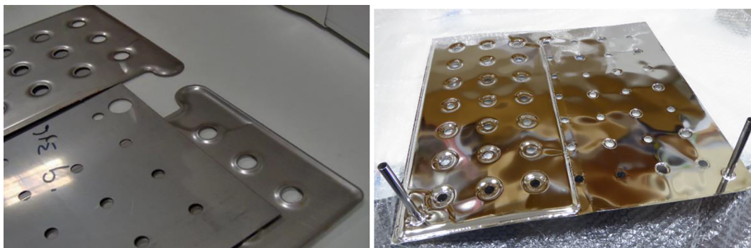
Fig. 3. (a) Laser-cut sheets prior to welding, (b) Absorber after leak testing and electro-polishing, prior to black chrome plating.
