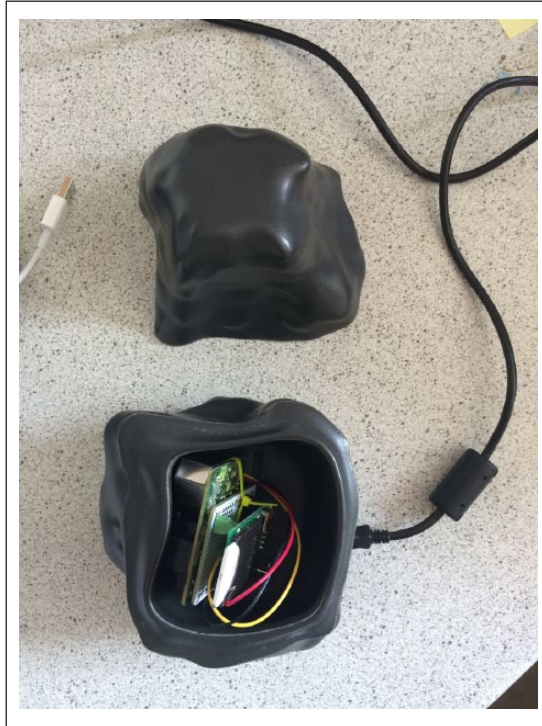
Figure 3. Dustbox particulate matter 2.5 monitor. Citizen Sense, 2016.
