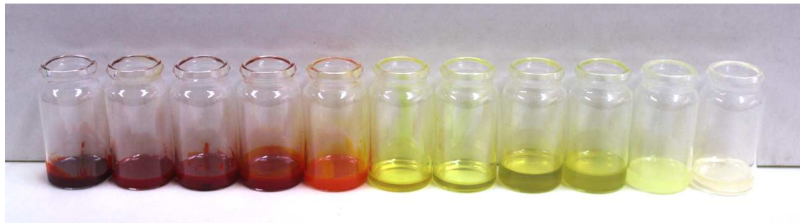
Figure 1. [\text{C}_4\text{C}_1\text{Im}]^+ based halobismuthate ionic liquids with different anions (from left to right): [\text{BiI}_3\text{Br}]^- , [\text{BiI}_3\text{Cl}]^- , [\text{BiBr}_2\text{I}_2]^- , [\text{BiCl}_2\text{I}_2]^- , [\text{BiBr}_2\text{ClI}]^- , [\text{BiBr}_4]^- , [\text{BiBr}_3\text{Cl}]^- , [\text{BiBr}_3\text{Cl}]^-_{0.5}[\text{NTf}_2]^-_{0.5} , [\text{BiBr}_2\text{Cl}_2]^- , [\text{BiBrCl}_3]^- , [\text{BiCl}_4]^- .
