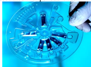
Figure 2. The LabDisk cartridge [13]
