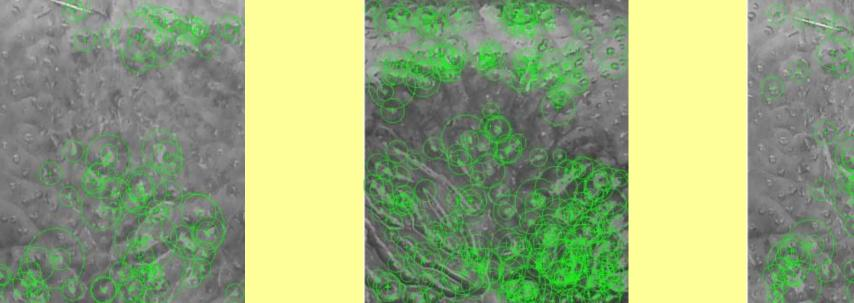
The next step is to extract the feature descriptors at interest points in both muzzle images. In the matching process we find putative point correspondences using feature's descriptors.
