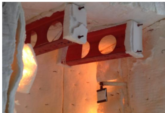
Figure 9. Cellular beam P5 in furnace test
