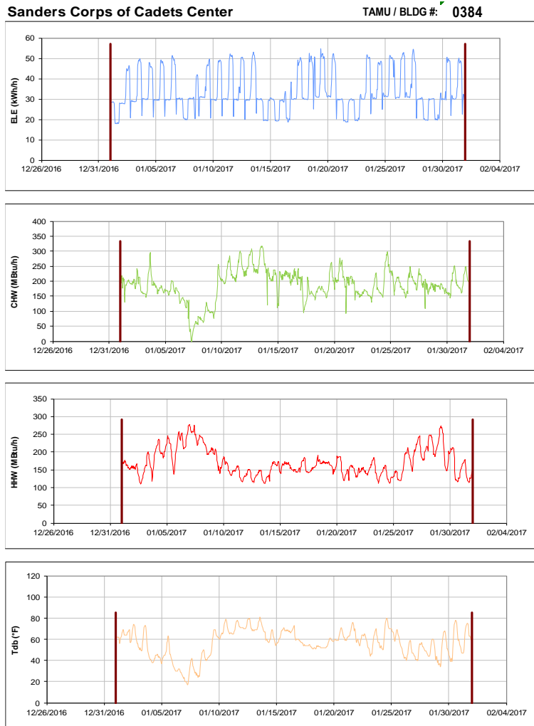
Figure III-19 Hourly Whole Building Electricity, Chilled Water, and Hot Water Consumption for Sanders Corps of Cadets Center during the Month of January 2017 and the Corresponding Hourly Outdoor Dry Bulb Temperature for College Station, TX
