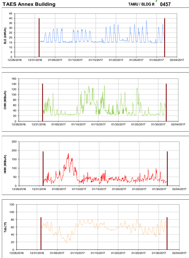
Figure III-75 Hourly Whole Building Electricity, Chilled Water, and Hot Water Consumption for TAES Annex Building during the Month of January 2017 and the Corresponding Hourly Outdoor Dry Bulb Temperature for College Station, TX
