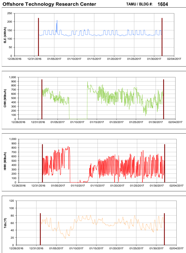
Figure III-181 Hourly Whole Building Electricity, Chilled Water, and Hot Water Consumption for Offshore Technology Research Center during the Month of January 2017 and the Corresponding Hourly Outdoor Dry Bulb Temperature for College Station, TX
