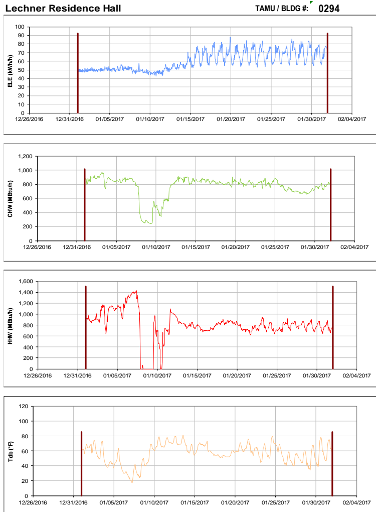
Figure III-7 Hourly Whole Building Electricity, Chilled Water, and Hot Water Consumption for Lechner Residence Hall during the Month of January 2017 and the Corresponding Hourly Outdoor Dry Bulb Temperature for College Station, TX
