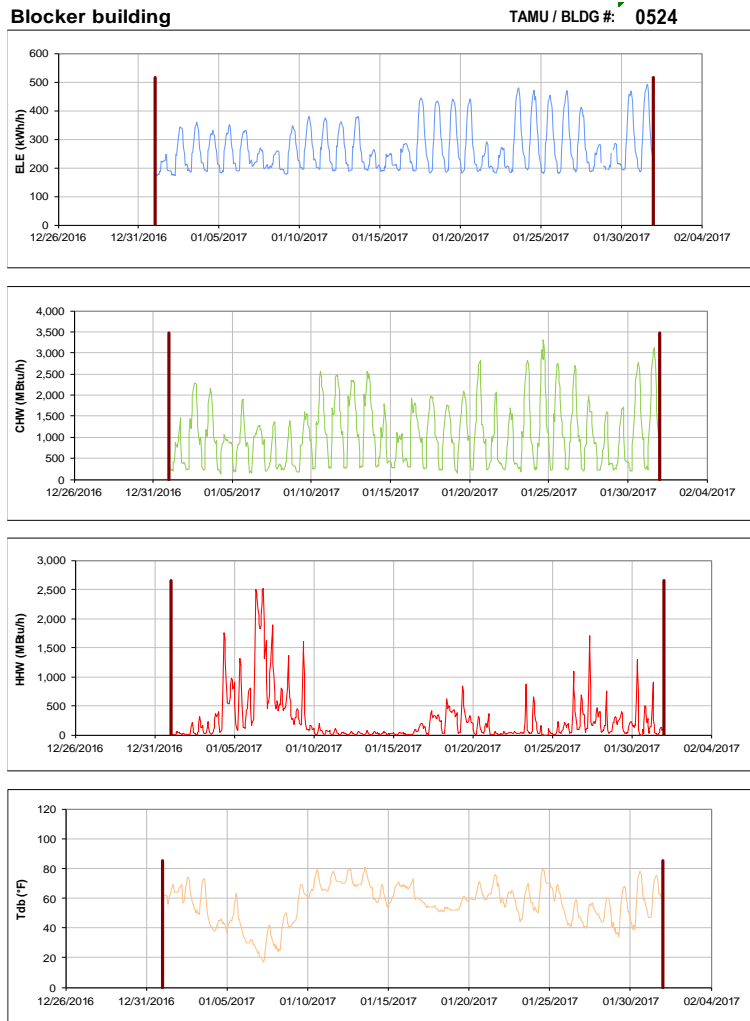
Figure III-113 Hourly Whole Building Electricity, Chilled Water, and Hot Water Consumption for Blocker building during the Month of January 2017 and the Corresponding Hourly Outdoor Dry Bulb Temperature for College Station, TX
