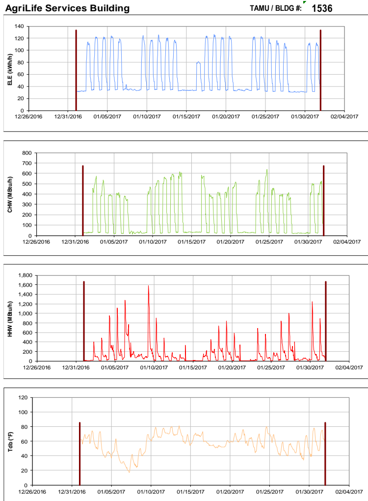
Figure III-165 Hourly Whole Building Electricity, Chilled Water, and Hot Water Consumption for AgriLife Services Building during the Month of January 2017 and the Corresponding Hourly Outdoor Dry Bulb Temperature for College Station, TX
