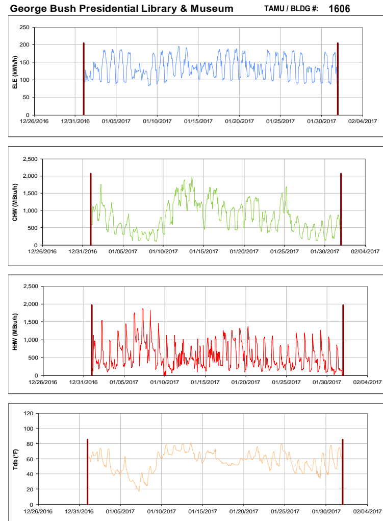
Figure III-182 Hourly Whole Building Electricity, Chilled Water, and Hot Water Consumption for George Bush Presidential Library & Museum during the Month of January 2017 and the Corresponding Hourly Outdoor Dry Bulb Temperature for College Station, TX
