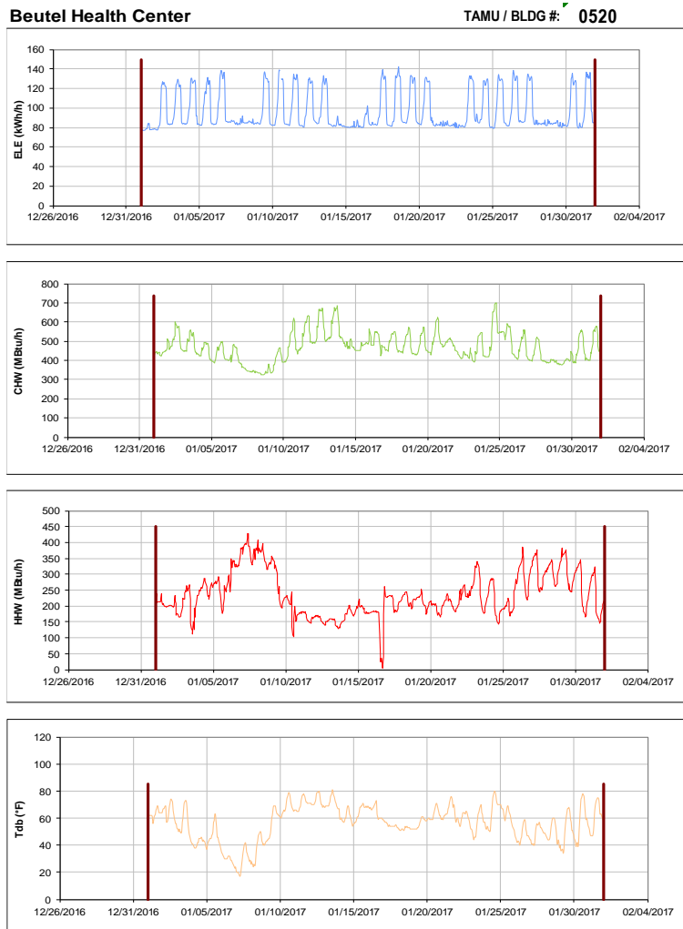
Figure III-111 Hourly Whole Building Electricity, Chilled Water, and Hot Water Consumption for Beutel Health Center during the Month of January 2017 and the Corresponding Hourly Outdoor Dry Bulb Temperature for College Station, TX
