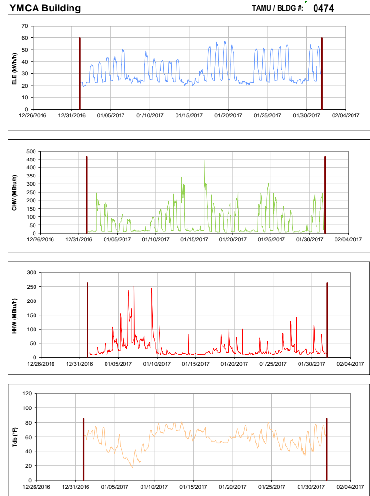
Figure III-88 Hourly Whole Building Electricity, Chilled Water, and Hot Water Consumption for YMCA Building during the Month of January 2017 and the Corresponding Hourly Outdoor Dry Bulb Temperature for College Station, TX
