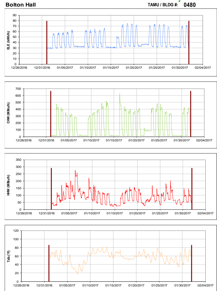
Figure III-92 Hourly Whole Building Electricity, Chilled Water, and Hot Water Consumption for Bolton Hall during the Month of January 2017 and the Corresponding Hourly Outdoor Dry Bulb Temperature for College Station, TX
