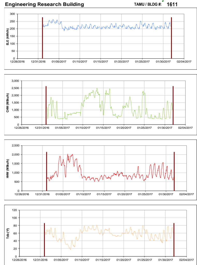
Figure III-186 Hourly Whole Building Electricity, Chilled Water, and Hot Water Consumption for Engineering Research Building during the Month of January 2017 and the Corresponding Hourly Outdoor Dry Bulb Temperature for College Station, TX
