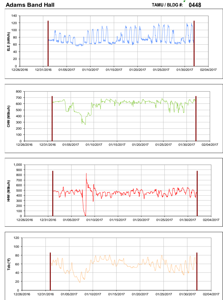
Figure III-70 Hourly Whole Building Electricity, Chilled Water, and Hot Water Consumption for Adams Band Hall during the Month of January 2017 and the Corresponding Hourly Outdoor Dry Bulb Temperature for College Station, TX
