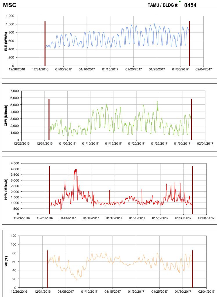
Figure III-73 Hourly Whole Building Electricity, Chilled Water, and Hot Water Consumption for MSC during the Month of January 2017 and the Corresponding Hourly Outdoor Dry Bulb Temperature for College Station, TX
