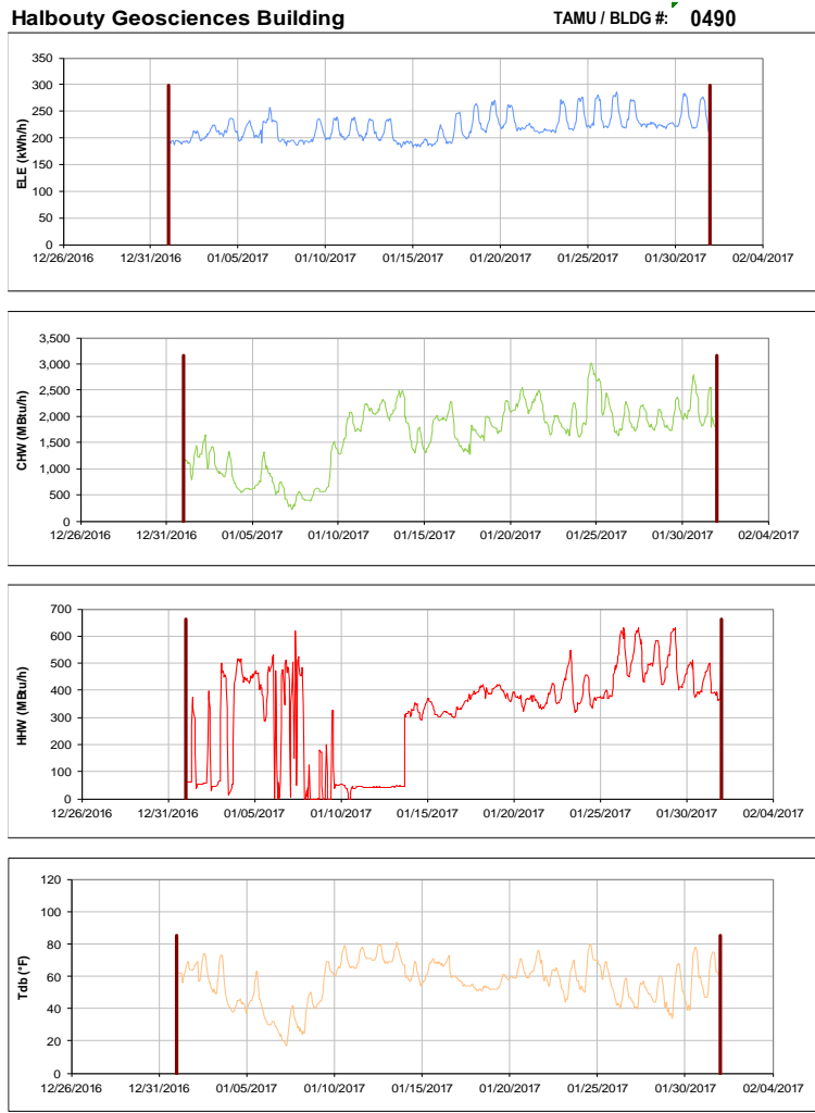
Figure III-97 Hourly Whole Building Electricity, Chilled Water, and Hot Water Consumption for Halbouty Geosciences Building during the Month of January 2017 and the Corresponding Hourly Outdoor Dry Bulb Temperature for College Station, TX
