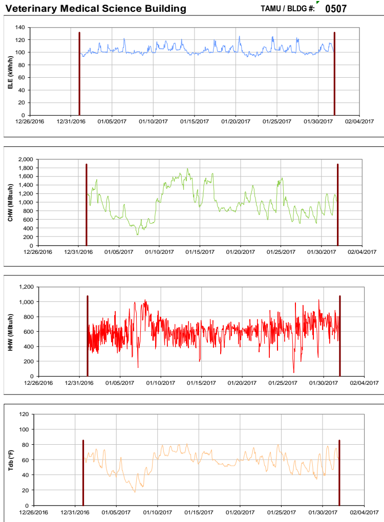
Figure III-103 Hourly Whole Building Electricity, Chilled Water, and Hot Water Consumption for Veterinary Medical Science Building during the Month of January 2017 and the Corresponding Hourly Outdoor Dry Bulb Temperature for College Station, TX
