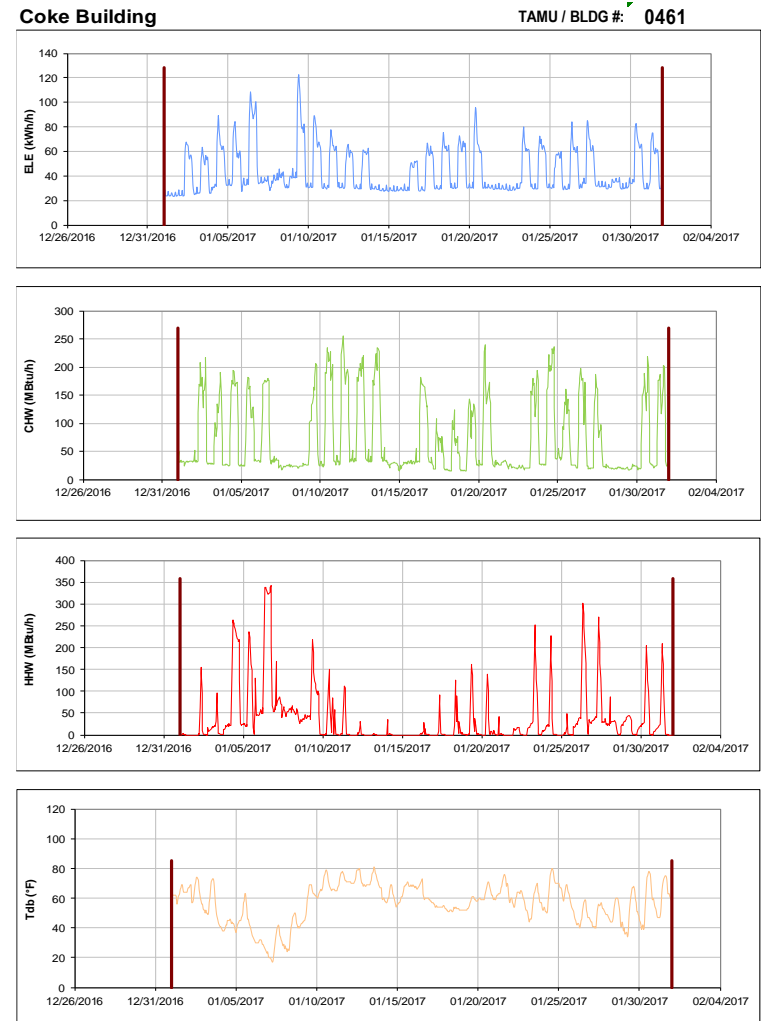
Figure III-76 Hourly Whole Building Electricity, Chilled Water, and Hot Water Consumption for Coke Building during the Month of January 2017 and the Corresponding Hourly Outdoor Dry Bulb Temperature for College Station, TX
