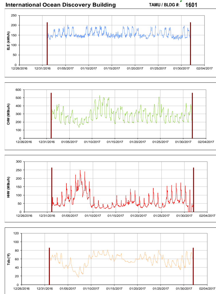
Figure III-180 Hourly Whole Building Electricity, Chilled Water, and Hot Water Consumption for International Ocean Discovery Building during the Month of January 2017 and the Corresponding Hourly Outdoor Dry Bulb Temperature for College Station, TX
