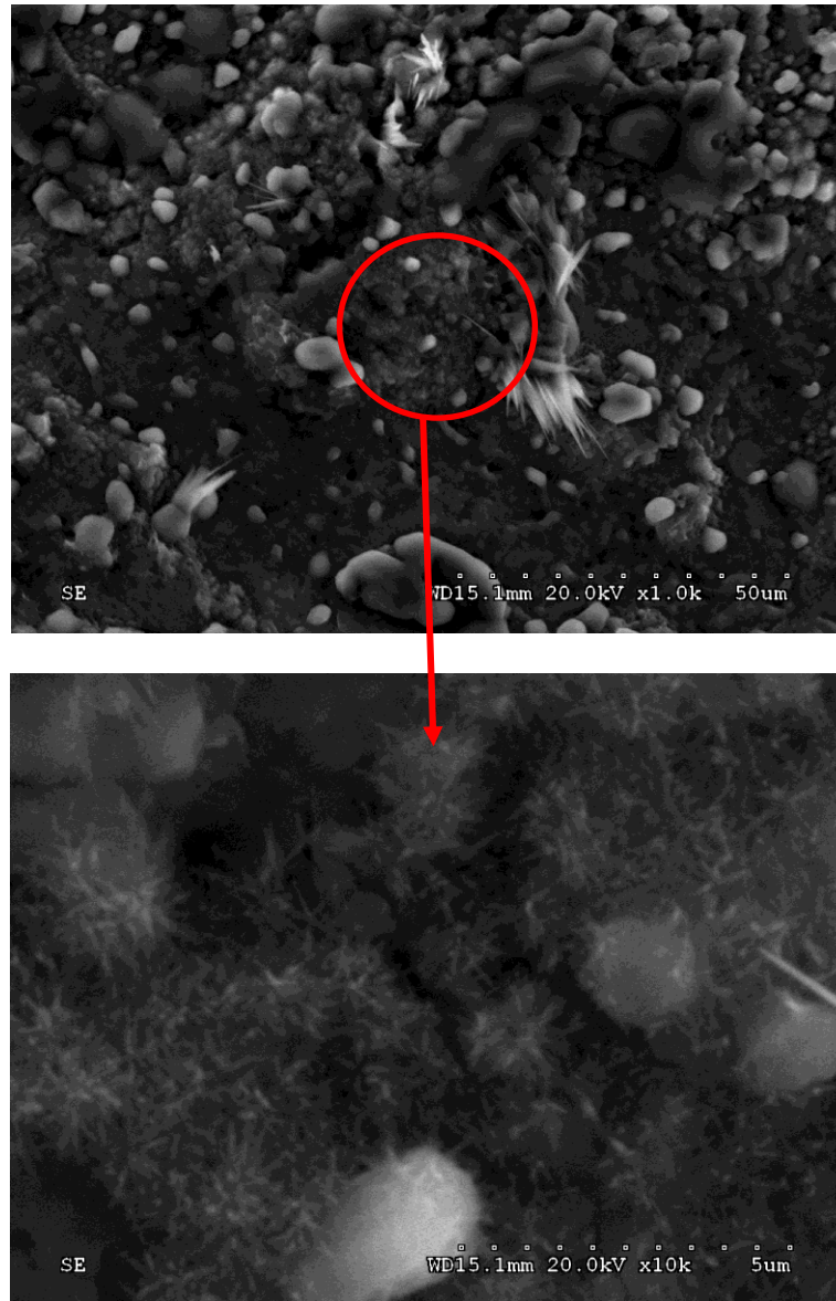
Figure 54. SEM images of solar salt nanofluid samples (one-step synthesis protocol). In addition to the cluster of single nano-needles observed in Figure 50 - the image shows other forms of secondary nanostructures: such as - fractal and dendritic structures that are formed in the sample. Images courtesy of Dr. D. Shin and his research group at the University of Texas at Arlington is gratefully acknowledged
