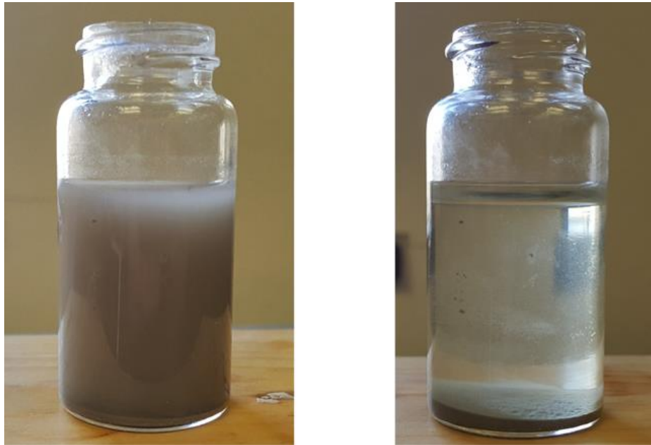
Figure 89. Observation of solar salt sample with magnesium nitrate additive. Image on the right shows solar salt with additive (immediately after thermal decomposition for in-situ synthesis). The image shows a colloidal suspension in the vial. The image on the right shows a dense sediment formed at the bottom of the vial with a clear and transparent liquid layer on top. This shows that the particles synthesized in-situ form an unstable colloidal solution which precipitate rapidly and therefore the specific heat capacity is not enhanced.
