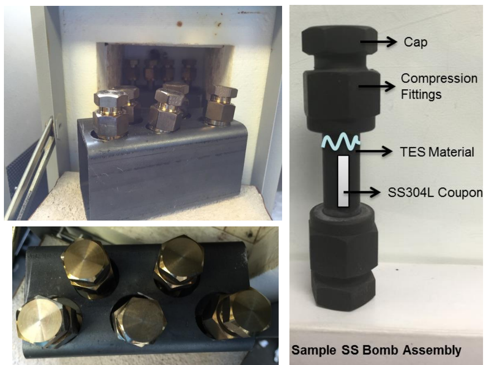
Figure 28. High temperature corrosion test apparatus indicating the level of the molten salt in the bomb.
