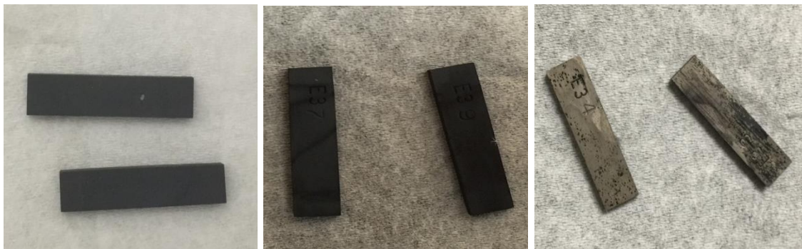
Figure 106. Images of the corrosion test coupons showing the change in sample morphology on implementing the following descaling protocols [97]: (LEFT) C.7.1; (MIDDLE) C.7.2; (RIGHT) C.7.4. Protocol C.7.4 appears to be the most effective descaling protocol in these experiments.
