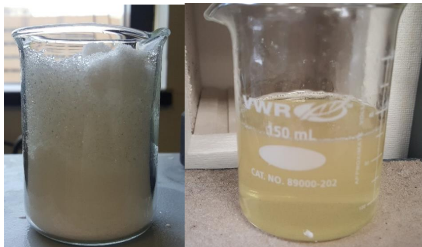
Figure 16. Images of solar salt samples. (LEFT) Additives mixed with pure solar salt before melting. (RIGHT) After melting and baking the mixture.
