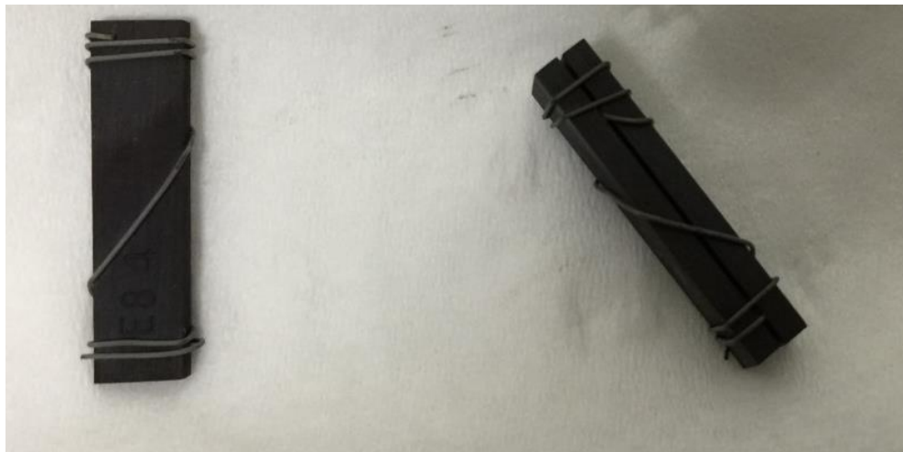
Figure 29. Separation of coupons by ceramic wire for electrical isolation.
