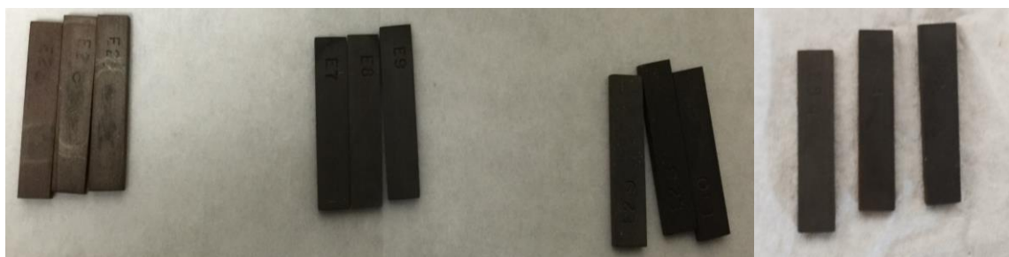
Figure 103. Image of the test coupons after heating at 565 °C for 120 hours in different environments (from left to right): (a) in air (control experiment); (b) in pure solar salt; (c) in solar salt nanofluid (with silica nanoparticles at a mass fraction of 1%); and (d) solar salt nanofluid with aluminum nitrate additive at a mass fraction of 6.9% (for a target mass fraction of 1% for alumina nanoparticles)
