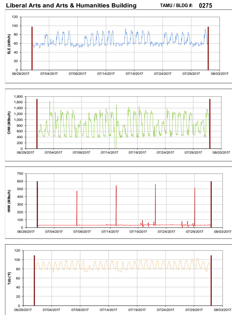
Figure III-2 Hourly Whole Building Electricity, Chilled Water, and Hot Water Consumption for Liberal Arts and Arts & Humanities Building during the Month of July 2017 and the Corresponding Hourly Outdoor Dry Bulb Temperature for College Station, TX
