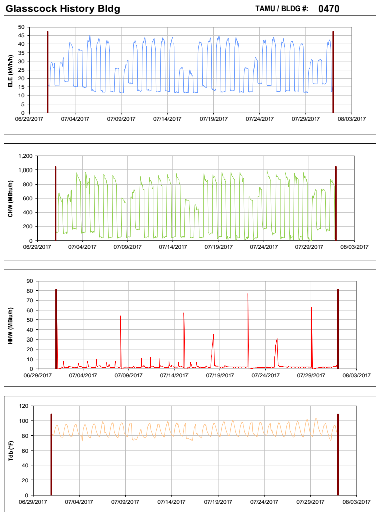
Figure III-83 Hourly Whole Building Electricity, Chilled Water, and Hot Water Consumption for Glasscock History Bldg during the Month of July 2017 and the Corresponding Hourly Outdoor Dry Bulb Temperature for College Station, TX
