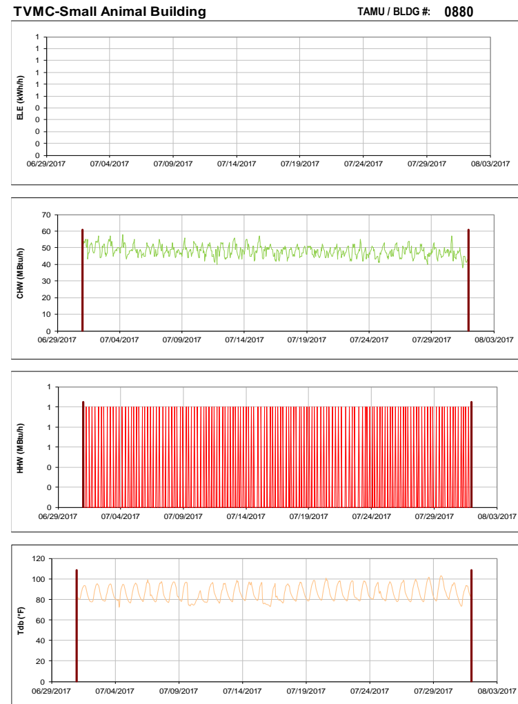
Figure III-124 Hourly Whole Building Electricity, Chilled Water, and Hot Water Consumption for TVMC-Small Animal Building during the Month of July 2017 and the Corresponding Hourly Outdoor Dry Bulb Temperature for College Station, TX
