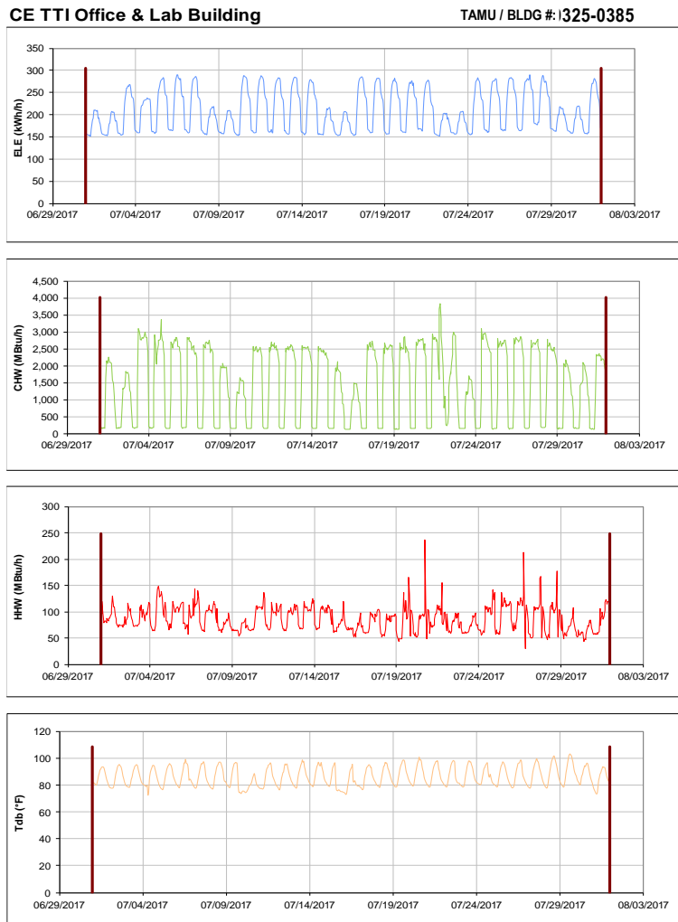
Figure III-9 Hourly Whole Building Electricity, Chilled Water, and Hot Water Consumption for CE TTI Office & Lab Building during the Month of July 2017 and the Corresponding Hourly Outdoor Dry Bulb Temperature for College Station, TX
