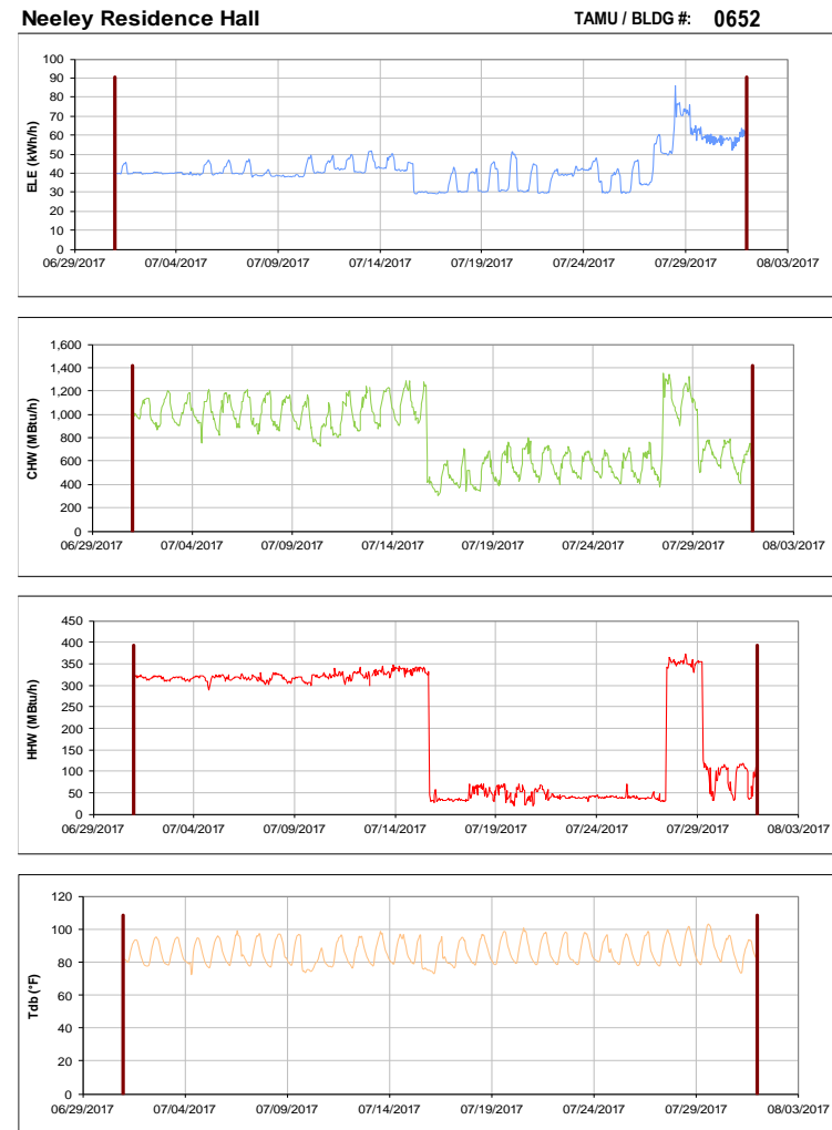
Figure III-118 Hourly Whole Building Electricity, Chilled Water, and Hot Water Consumption for Neeley Residence Hall during the Month of July 2017 and the Corresponding Hourly Outdoor Dry Bulb Temperature for College Station, TX
