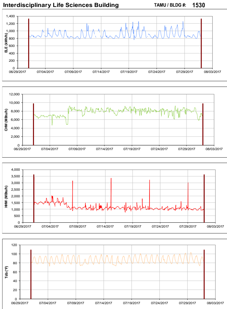
Figure III-169 Hourly Whole Building Electricity, Chilled Water, and Hot Water Consumption for Interdisciplinary Life Sciences Building during the Month of July 2017 and the Corresponding Hourly Outdoor Dry Bulb Temperature for College Station, TX
