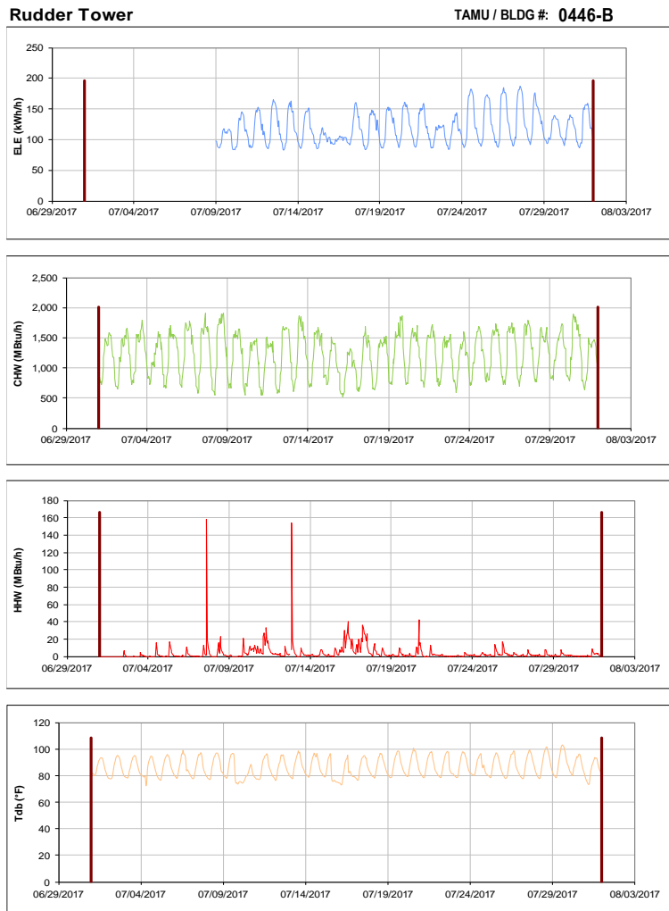
Figure III-67 Hourly Whole Building Electricity, Chilled Water, and Hot Water Consumption for Rudder Tower during the Month of July 2017 and the Corresponding Hourly Outdoor Dry Bulb Temperature for College Station, TX
