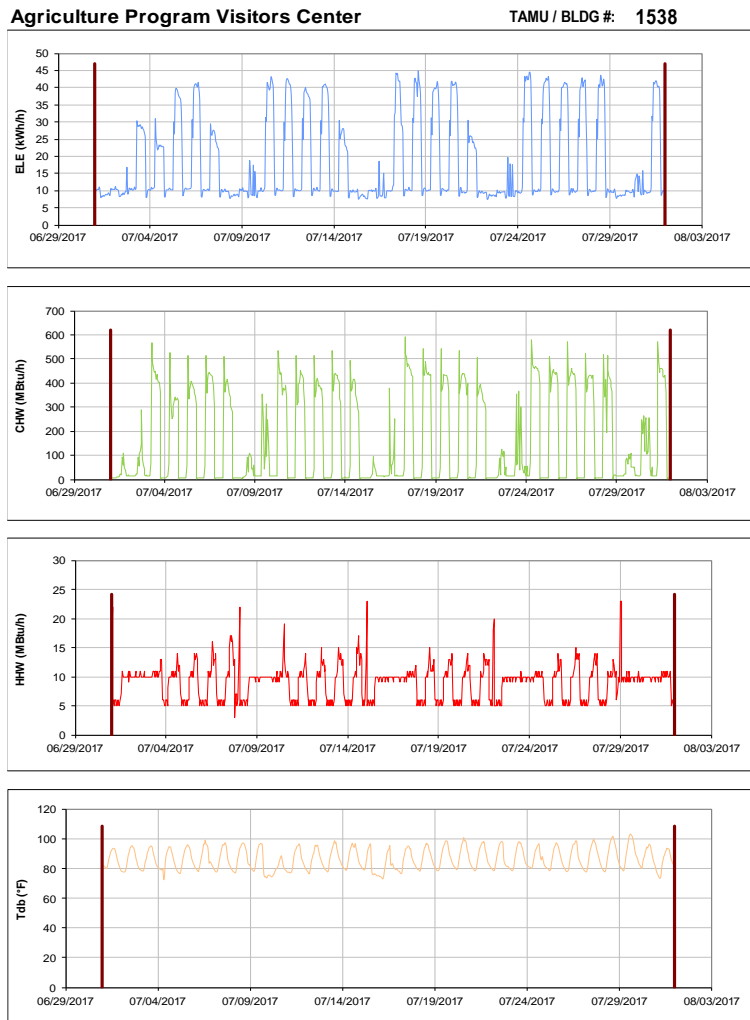
Figure III-173 Hourly Whole Building Electricity, Chilled Water, and Hot Water Consumption for Agriculture Program Visitors Center during the Month of July 2017 and the Corresponding Hourly Outdoor Dry Bulb Temperature for College Station, TX
