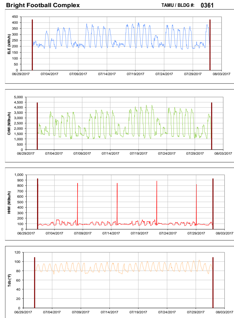
Figure III-14 Hourly Whole Building Electricity, Chilled Water, and Hot Water Consumption for Bright Football Complex during the Month of July 2017 and the Corresponding Hourly Outdoor Dry Bulb Temperature for College Station, TX
