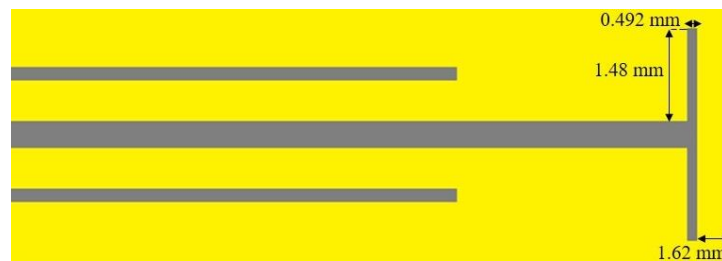
Fig. 10. Dielectric coated monopole with terminating cap
