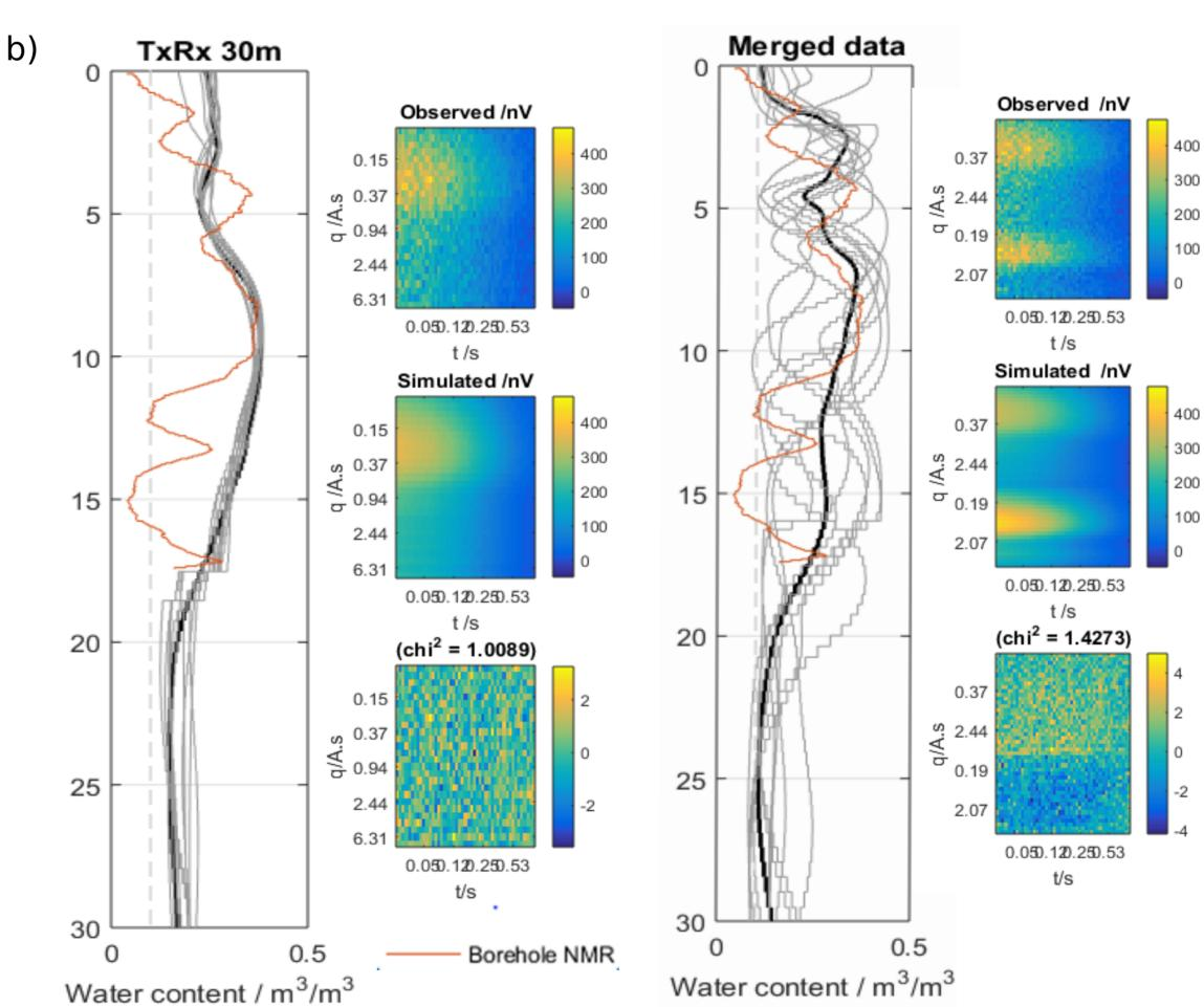
The loss in data fitting precision is likely due to a wrong weighting of the data due the different noise distribution of the two data sets. Fig. 3c
