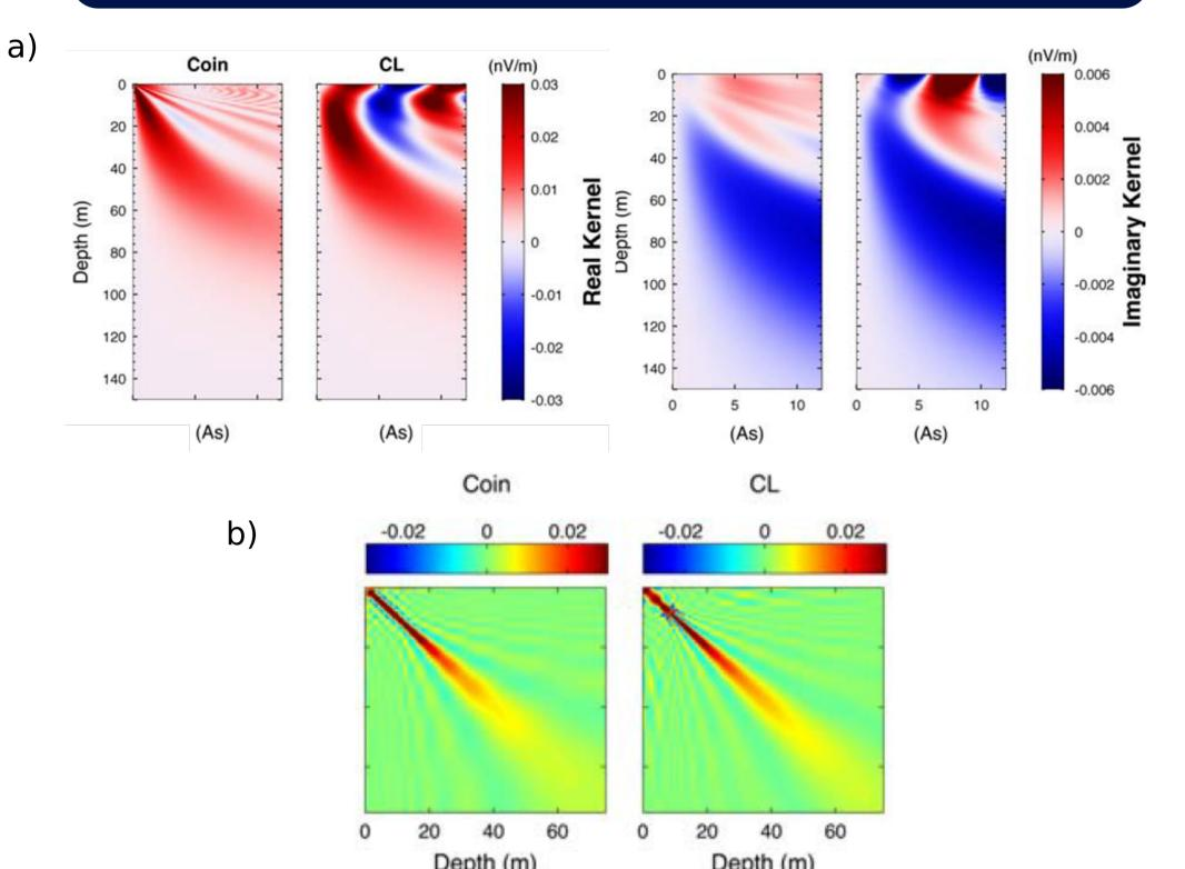
The central-loop (CL) configuration has benefits compared to the "classical" coincident loop configuration, as demonstrated by Berhoozmand et al. (2016). The complex kernels show additional sensitivity features in the shallow part (Fig. 1a). Also, resolution studies show that the CL configuration probes deeper than the coincident one when using complex data (Fig. 1b, modified after Berhoozmand et al. 2016).
