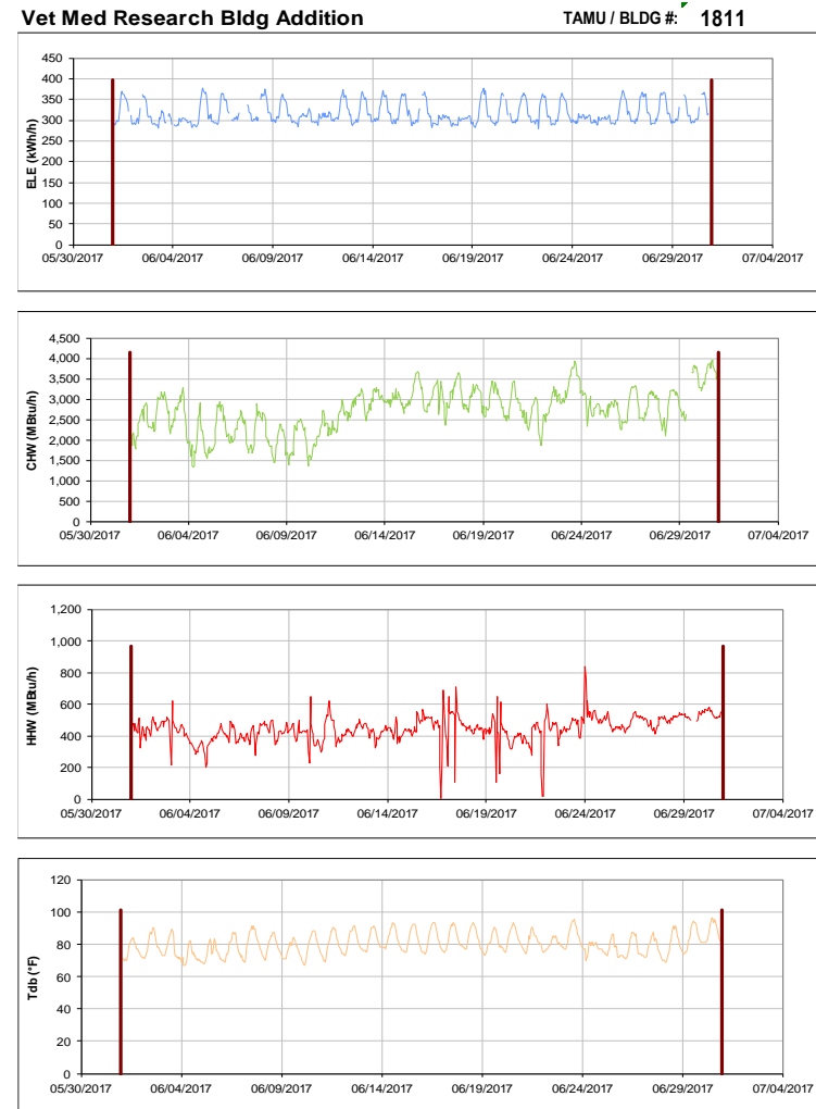
Figure III-196 Hourly Whole Building Electricity, Chilled Water, and Hot Water Consumption for Vet Med Research Bldg Addition during the Month of June 2017 and the Corresponding Hourly Outdoor Dry Bulb Temperature for College Station, TX
