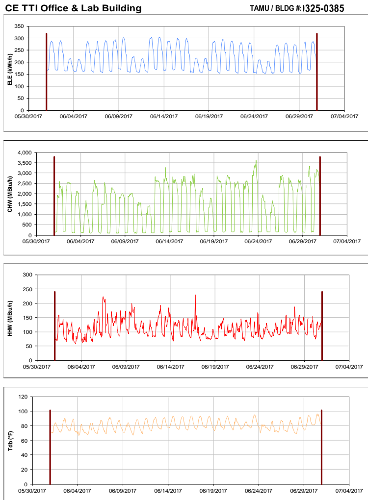
Figure III-9 Hourly Whole Building Electricity, Chilled Water, and Hot Water Consumption for CE TTI Office & Lab Building during the Month of June 2017 and the Corresponding Hourly Outdoor Dry Bulb Temperature for College Station, TX
