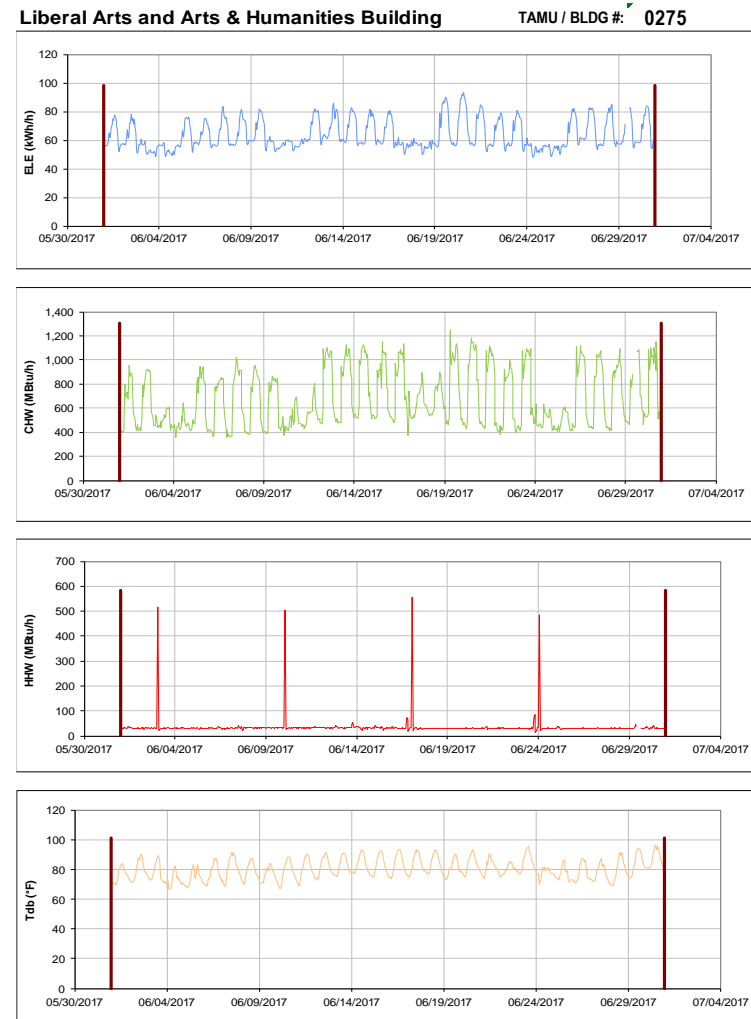
Figure III-2 Hourly Whole Building Electricity, Chilled Water, and Hot Water Consumption for Liberal Arts and Arts & Humanities Building during the Month of June 2017 and the Corresponding Hourly Outdoor Dry Bulb Temperature for College Station, TX
