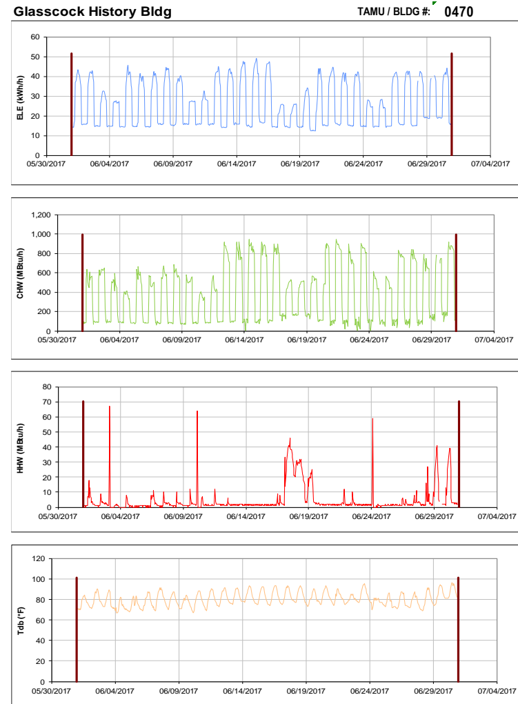
Figure III-88 Hourly Whole Building Electricity, Chilled Water, and Hot Water Consumption for Glasscock History Bldg during the Month of June 2017 and the Corresponding Hourly Outdoor Dry Bulb Temperature for College Station, TX
