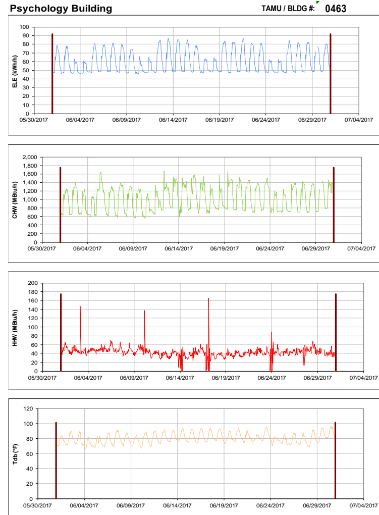
Figure III-82 Hourly Whole Building Electricity, Chilled Water, and Hot Water Consumption for Psychology Building during the Month of June 2017 and the Corresponding Hourly Outdoor Dry Bulb Temperature for College Station, TX
