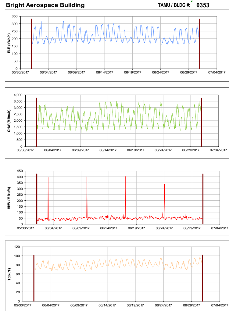
Figure III-10 Hourly Whole Building Electricity, Chilled Water, and Hot Water Consumption for Bright Aerospace Building during the Month of June 2017 and the Corresponding Hourly Outdoor Dry Bulb Temperature for College Station, TX
