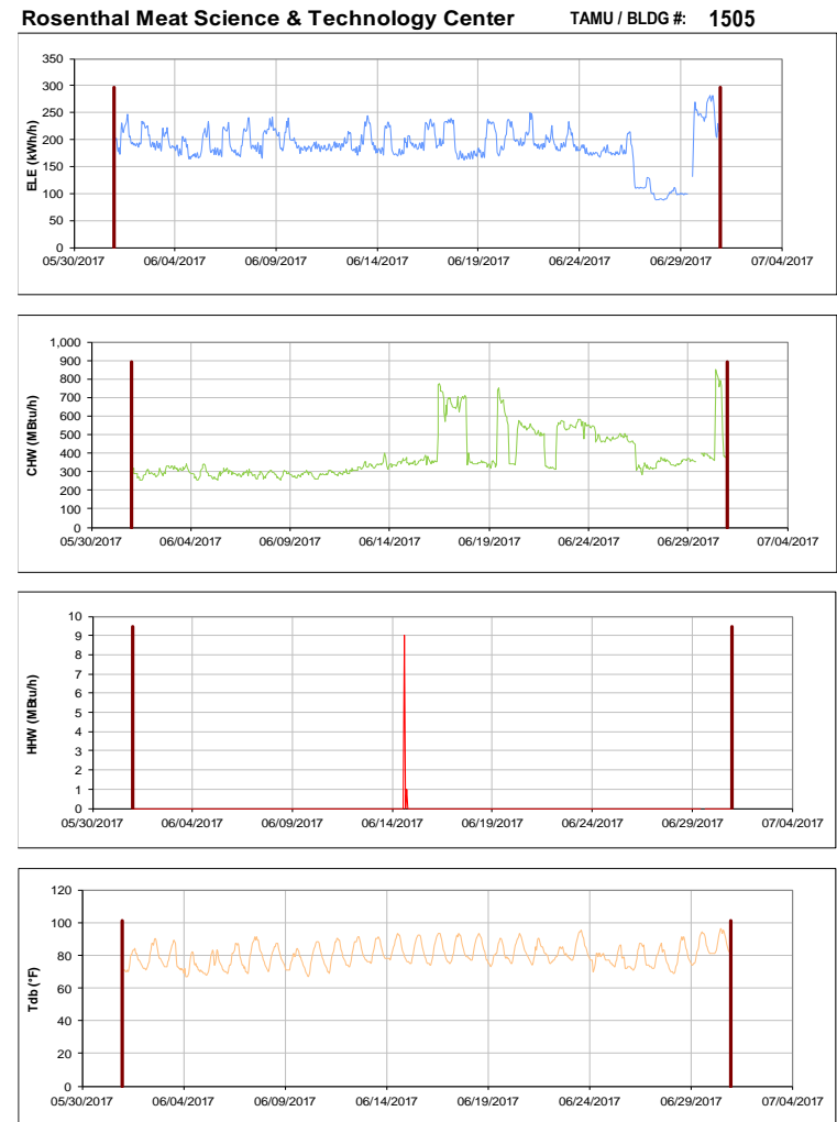
Figure III-158 Hourly Whole Building Electricity, Chilled Water, and Hot Water Consumption for Rosenthal Meat Science & Technology Center during the Month of June 2017 and the Corresponding Hourly Outdoor Dry Bulb Temperature for College Station, TX
