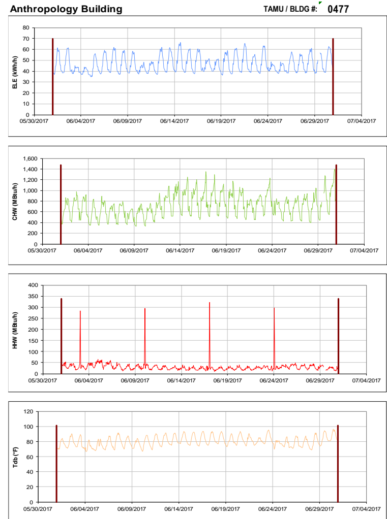
Figure III-94 Hourly Whole Building Electricity, Chilled Water, and Hot Water Consumption for Anthropology Building during the Month of June 2017 and the Corresponding Hourly Outdoor Dry Bulb Temperature for College Station, TX
