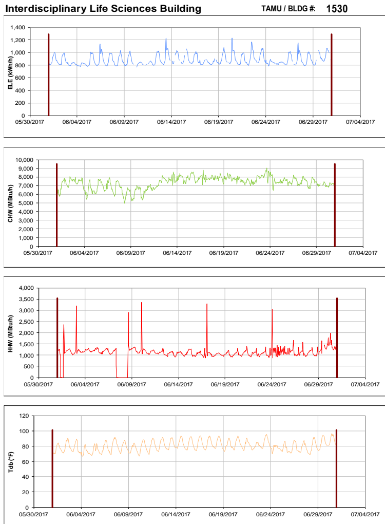
Figure III-169 Hourly Whole Building Electricity, Chilled Water, and Hot Water Consumption for Interdisciplinary Life Sciences Building during the Month of June 2017 and the Corresponding Hourly Outdoor Dry Bulb Temperature for College Station, TX
