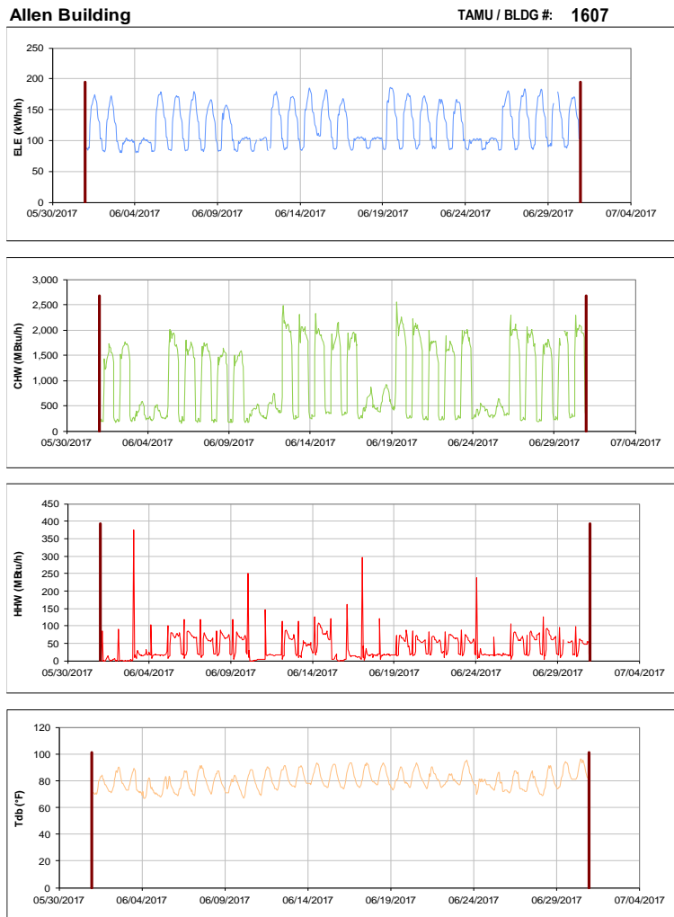
Figure III-189 Hourly Whole Building Electricity, Chilled Water, and Hot Water Consumption for Allen Building during the Month of June 2017 and the Corresponding Hourly Outdoor Dry Bulb Temperature for College Station, TX
