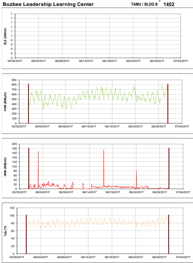
Figure III-39 Hourly Whole Building Electricity, Chilled Water, and Hot Water Consumption for Buzbee Leadership Learning Center during the Month of June 2017 and the Corresponding Hourly Outdoor Dry Bulb Temperature for College Station, TX
