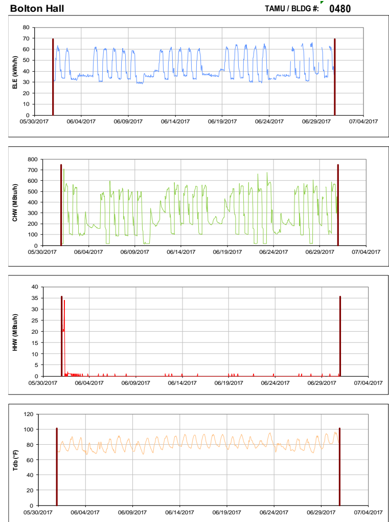
Figure III-96 Hourly Whole Building Electricity, Chilled Water, and Hot Water Consumption for Bolton Hall during the Month of June 2017 and the Corresponding Hourly Outdoor Dry Bulb Temperature for College Station, TX
