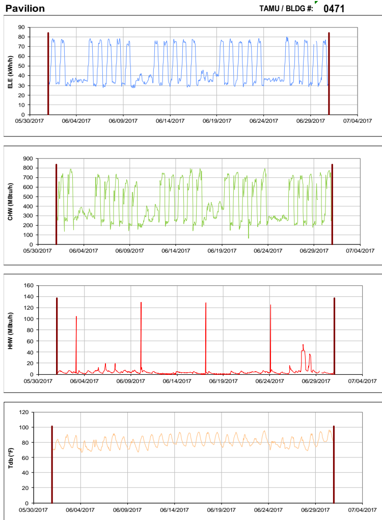
Figure III-89 Hourly Whole Building Electricity, Chilled Water, and Hot Water Consumption for Pavilion during the Month of June 2017 and the Corresponding Hourly Outdoor Dry Bulb Temperature for College Station, TX
