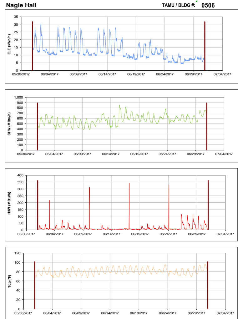
Figure III-106 Hourly Whole Building Electricity, Chilled Water, and Hot Water Consumption for Nagle Hall during the Month of June 2017 and the Corresponding Hourly Outdoor Dry Bulb Temperature for College Station, TX
