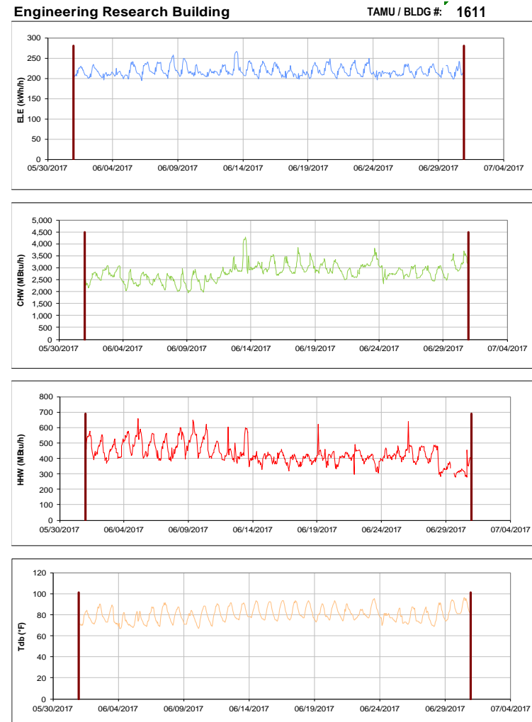
Figure III-192 Hourly Whole Building Electricity, Chilled Water, and Hot Water Consumption for Engineering Research Building during the Month of June 2017 and the Corresponding Hourly Outdoor Dry Bulb Temperature for College Station, TX
