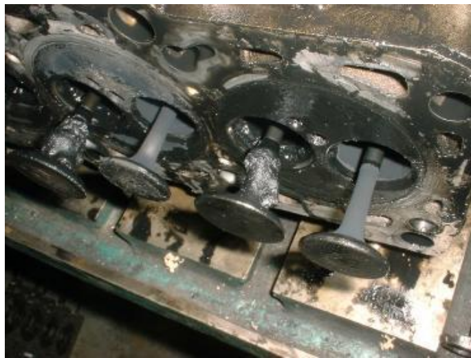
Figure 1-3: Hydrocarbon Deposits on Inlet Valves. Reprinted from [10]
