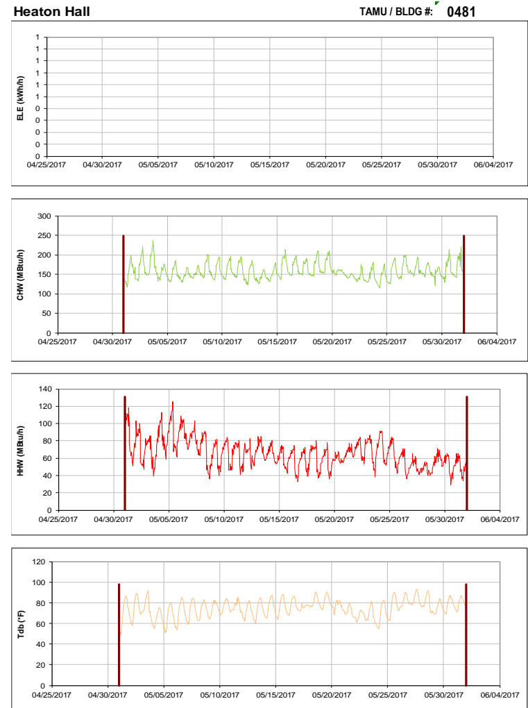
Figure III-98 Hourly Whole Building Electricity, Chilled Water, and Hot Water Consumption for Heaton Hall during the Month of May 2017 and the Corresponding Hourly Outdoor Dry Bulb Temperature for College Station, TX
