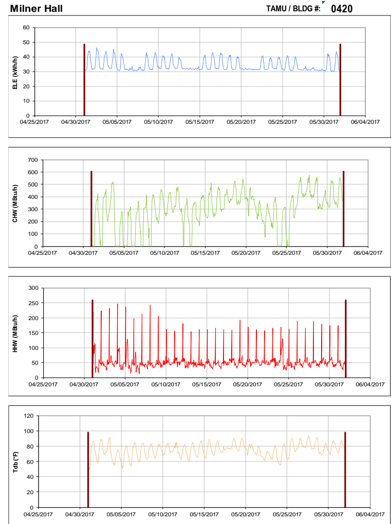
Figure III-48 Hourly Whole Building Electricity, Chilled Water, and Hot Water Consumption for Milner Hall during the Month of May 2017 and the Corresponding Hourly Outdoor Dry Bulb Temperature for College Station, TX
