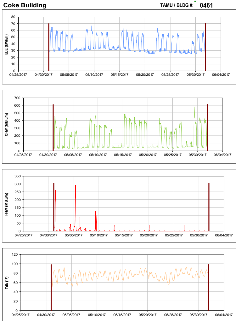
Figure III-81 Hourly Whole Building Electricity, Chilled Water, and Hot Water Consumption for Coke Building during the Month of May 2017 and the Corresponding Hourly Outdoor Dry Bulb Temperature for College Station, TX
