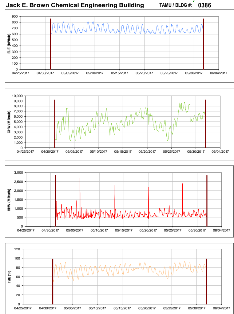
Figure III-20 Hourly Whole Building Electricity, Chilled Water, and Hot Water Consumption for Jack E. Brown Chemical Engineering Building during the Month of May 2017 and the Corresponding Hourly Outdoor Dry Bulb Temperature for College Station, TX
