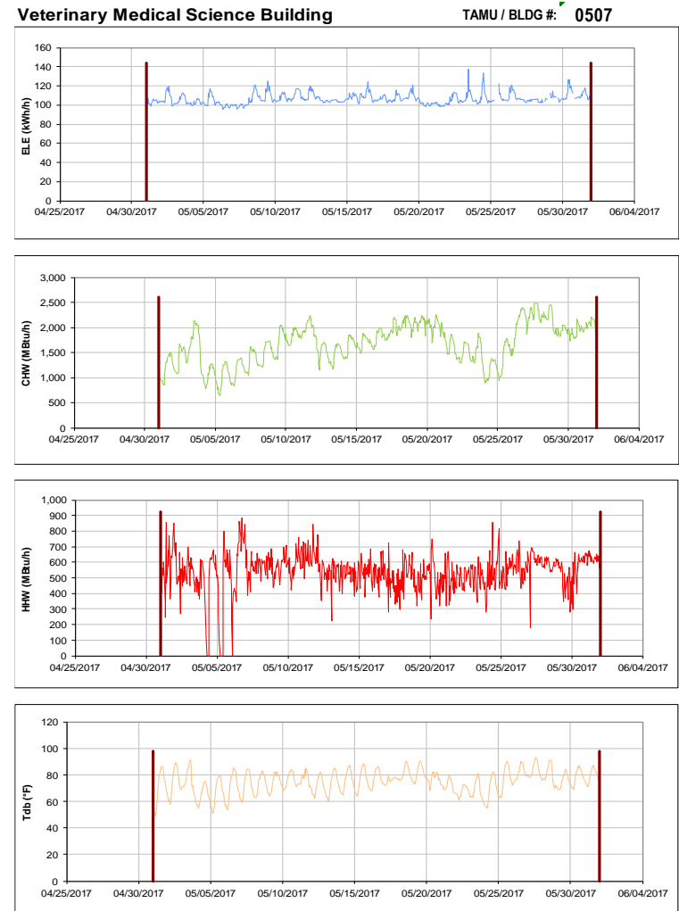
Figure III-108 Hourly Whole Building Electricity, Chilled Water, and Hot Water Consumption for Veterinary Medical Science Building during the Month of May 2017 and the Corresponding Hourly Outdoor Dry Bulb Temperature for College Station, TX
