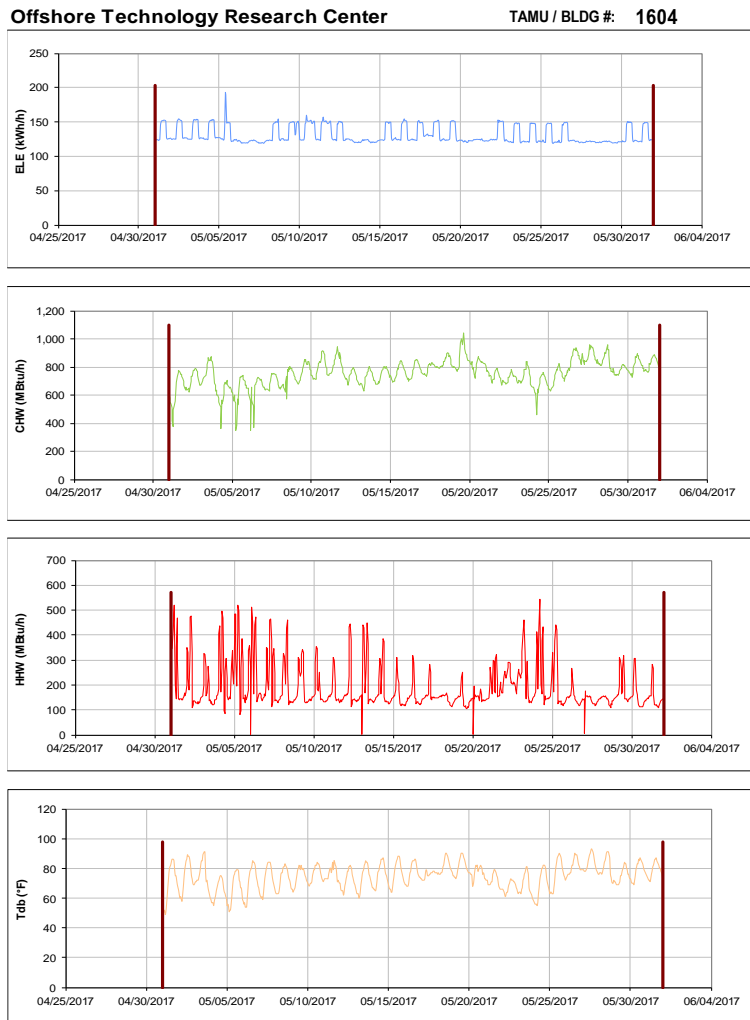
Figure III-187 Hourly Whole Building Electricity, Chilled Water, and Hot Water Consumption for Offshore Technology Research Center during the Month of May 2017 and the Corresponding Hourly Outdoor Dry Bulb Temperature for College Station, TX
