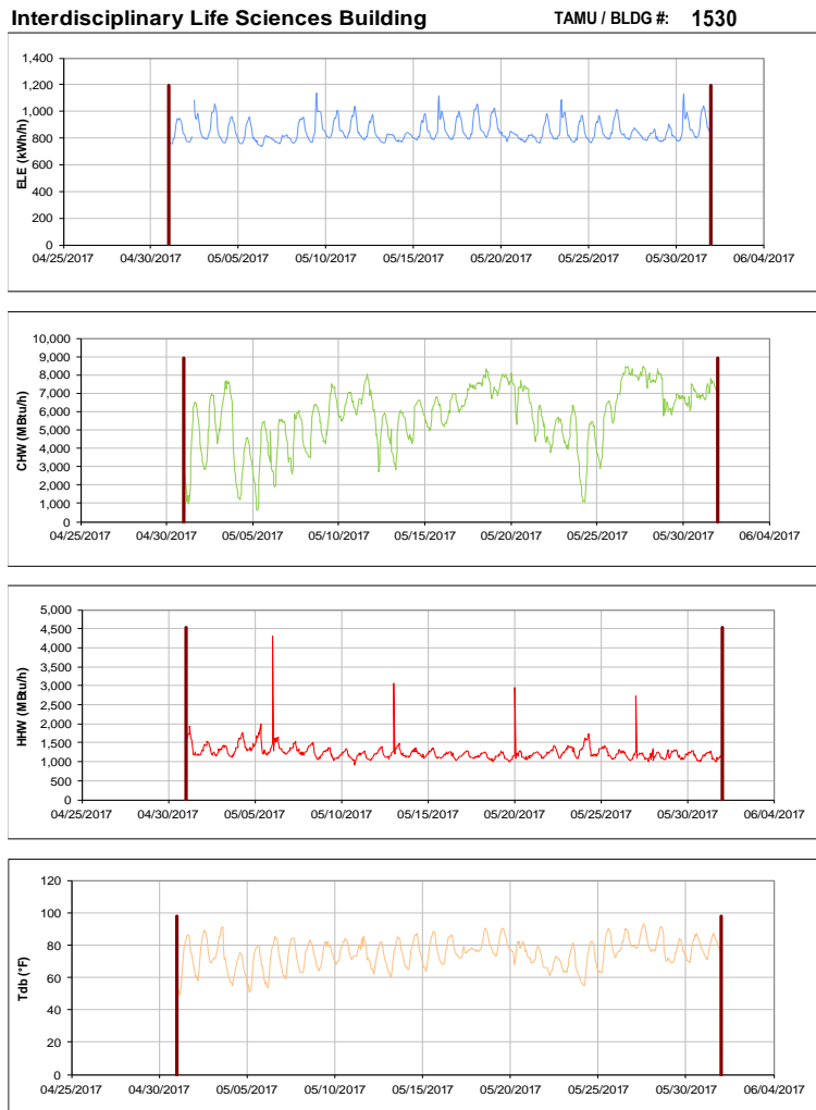
Figure III-169 Hourly Whole Building Electricity, Chilled Water, and Hot Water Consumption for Interdisciplinary Life Sciences Building during the Month of May 2017 and the Corresponding Hourly Outdoor Dry Bulb Temperature for College Station, TX
