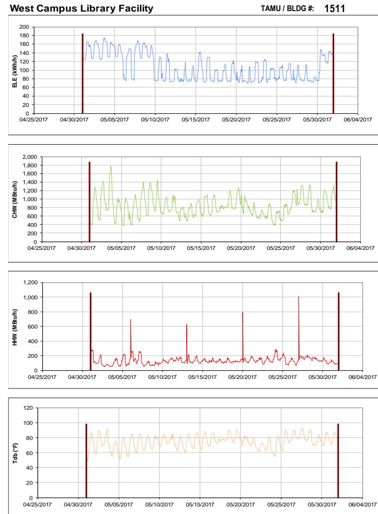
Figure III-164 Hourly Whole Building Electricity, Chilled Water, and Hot Water Consumption for West Campus Library Facility during the Month of May 2017 and the Corresponding Hourly Outdoor Dry Bulb Temperature for College Station, TX
