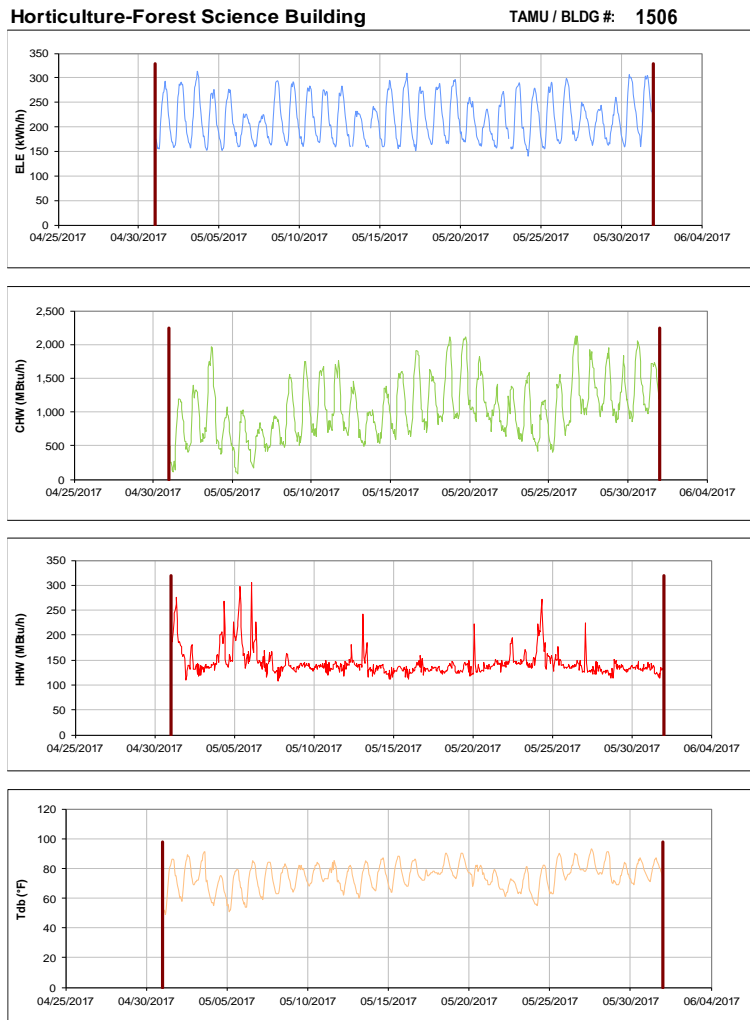
Figure III-159 Hourly Whole Building Electricity, Chilled Water, and Hot Water Consumption for Horticulture-Forest Science Building during the Month of May 2017 and the Corresponding Hourly Outdoor Dry Bulb Temperature for College Station, TX
