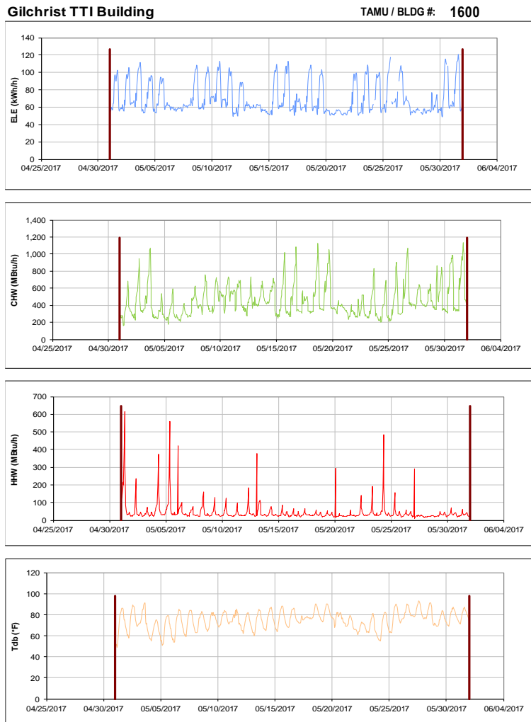
Figure III-185 Hourly Whole Building Electricity, Chilled Water, and Hot Water Consumption for Gilchrist TTI Building during the Month of May 2017 and the Corresponding Hourly Outdoor Dry Bulb Temperature for College Station, TX
