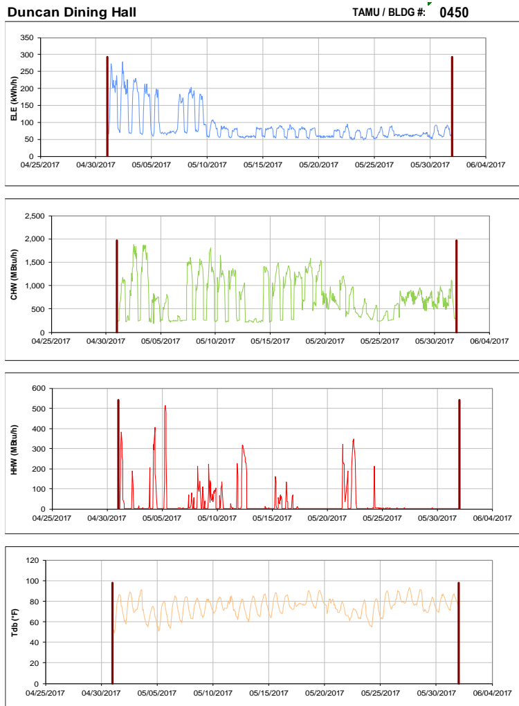
Figure III-77 Hourly Whole Building Electricity, Chilled Water, and Hot Water Consumption for Duncan Dining Hall during the Month of May 2017 and the Corresponding Hourly Outdoor Dry Bulb Temperature for College Station, TX
