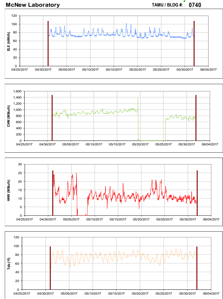
Figure III-126 Hourly Whole Building Electricity, Chilled Water, and Hot Water Consumption for McNew Laboratory during the Month of May 2017 and the Corresponding Hourly Outdoor Dry Bulb Temperature for College Station, TX
