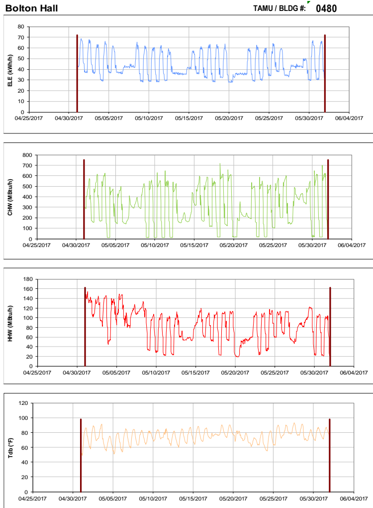
Figure III-97 Hourly Whole Building Electricity, Chilled Water, and Hot Water Consumption for Bolton Hall during the Month of May 2017 and the Corresponding Hourly Outdoor Dry Bulb Temperature for College Station, TX
