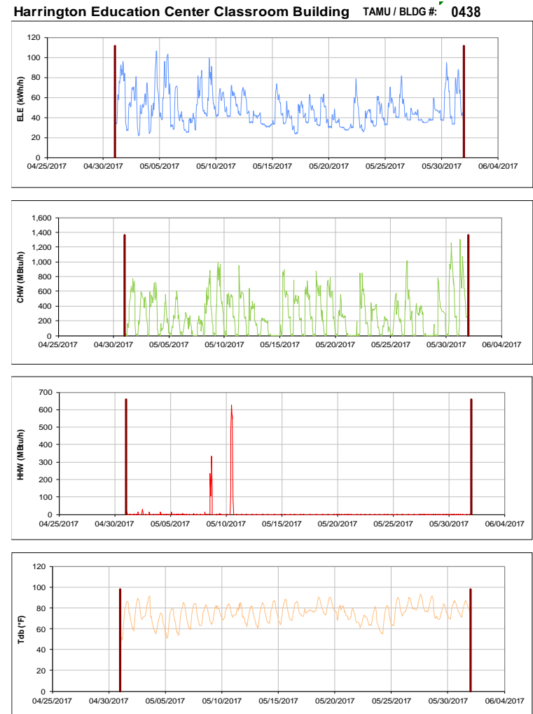
Figure III-66 Hourly Whole Building Electricity, Chilled Water, and Hot Water Consumption for Harrington Education Center Classroom Building during the Month of May 2017 and the Corresponding Hourly Outdoor Dry Bulb Temperature for College Station, TX
