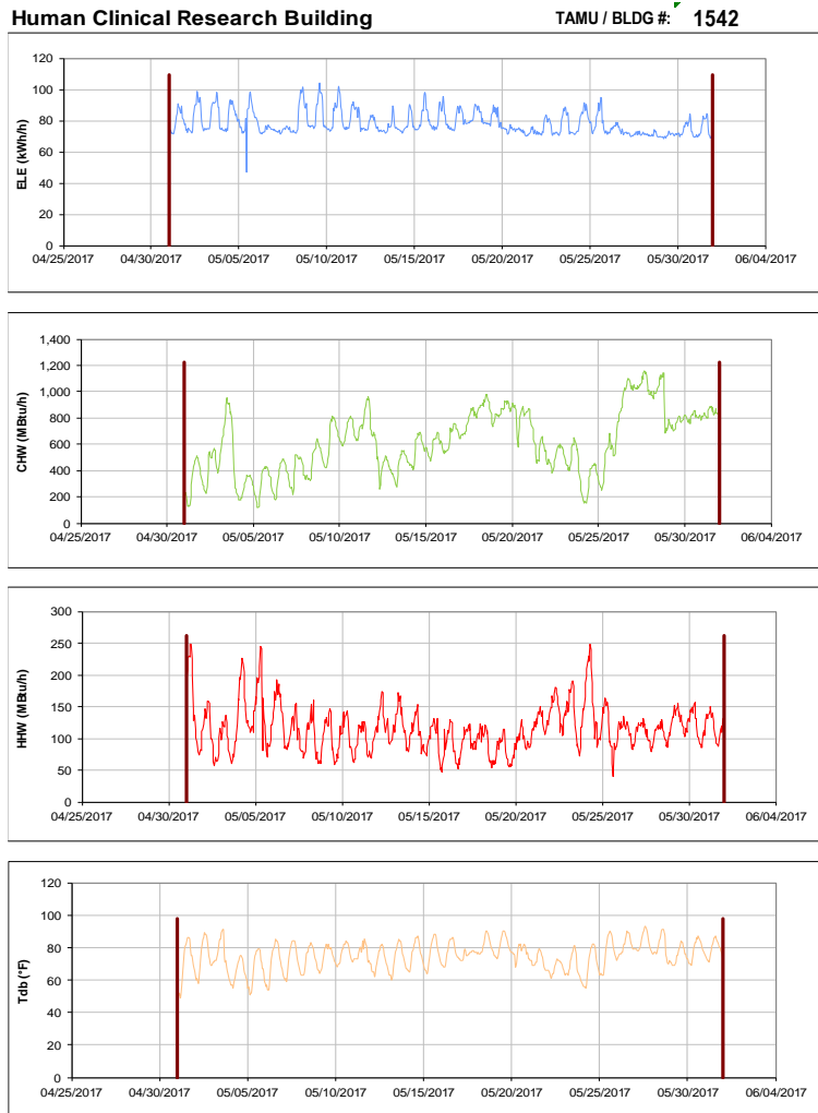
Figure III-175 Hourly Whole Building Electricity, Chilled Water, and Hot Water Consumption for Human Clinical Research Building during the Month of May 2017 and the Corresponding Hourly Outdoor Dry Bulb Temperature for College Station, TX
