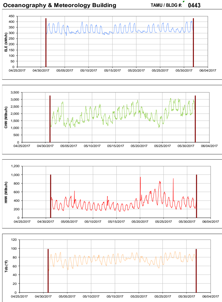
Figure III-67 Hourly Whole Building Electricity, Chilled Water, and Hot Water Consumption for Oceanography & Meteorology Building during the Month of May 2017 and the Corresponding Hourly Outdoor Dry Bulb Temperature for College Station, TX
