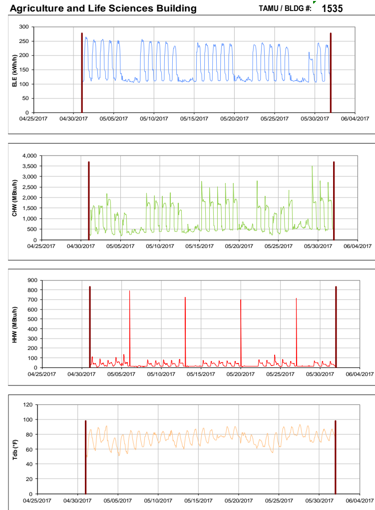
Figure III-170 Hourly Whole Building Electricity, Chilled Water, and Hot Water Consumption for Agriculture and Life Sciences Building during the Month of May 2017 and the Corresponding Hourly Outdoor Dry Bulb Temperature for College Station, TX
