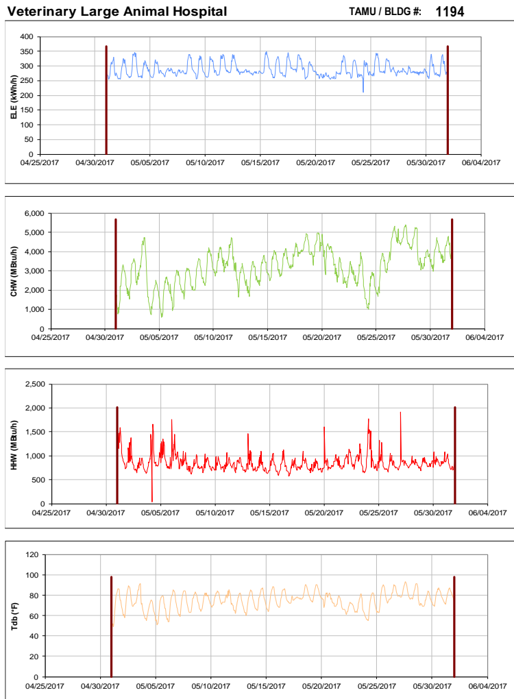
Figure III-139 Hourly Whole Building Electricity, Chilled Water, and Hot Water Consumption for Veterinary Large Animal Hospital during the Month of May 2017 and the Corresponding Hourly Outdoor Dry Bulb Temperature for College Station, TX
