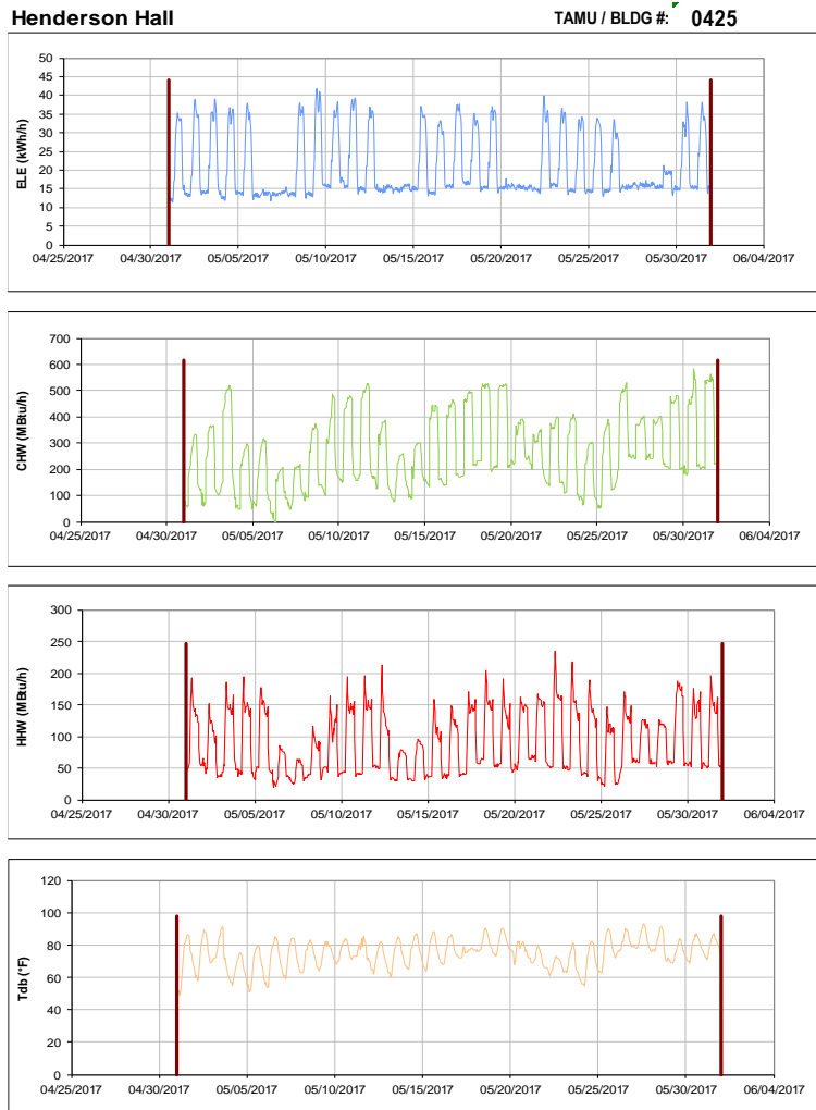
Figure III-51 Hourly Whole Building Electricity, Chilled Water, and Hot Water Consumption for Henderson Hall during the Month of May 2017 and the Corresponding Hourly Outdoor Dry Bulb Temperature for College Station, TX
