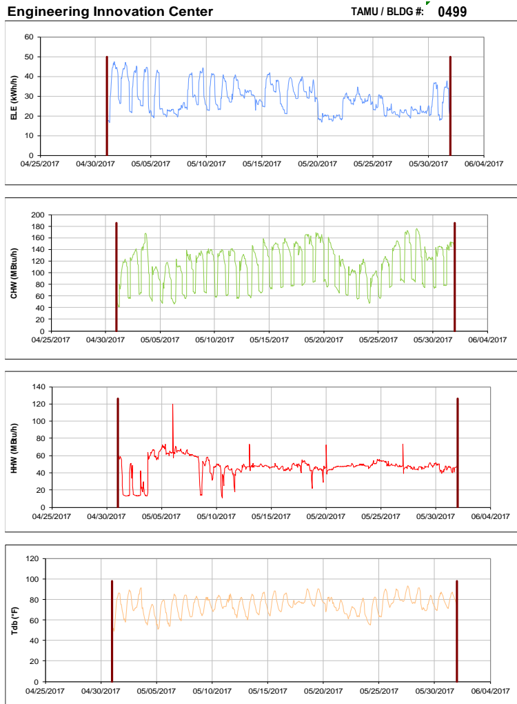
Figure III-65 Hourly Whole Building Electricity, Chilled Water, and Hot Water Consumption for Engineering Innovation Center during the Month of May 2017 and the Corresponding Hourly Outdoor Dry Bulb Temperature for College Station, TX
