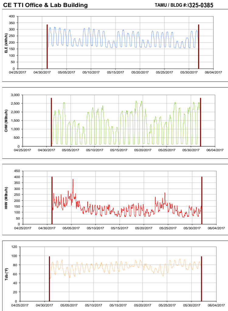
Figure III-9 Hourly Whole Building Electricity, Chilled Water, and Hot Water Consumption for CE TTI Office & Lab Building during the Month of May 2017 and the Corresponding Hourly Outdoor Dry Bulb Temperature for College Station, TX
