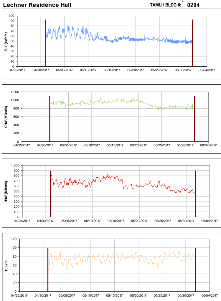
Figure III-7 Hourly Whole Building Electricity, Chilled Water, and Hot Water Consumption for Lechner Residence Hall during the Month of May 2017 and the Corresponding Hourly Outdoor Dry Bulb Temperature for College Station, TX
