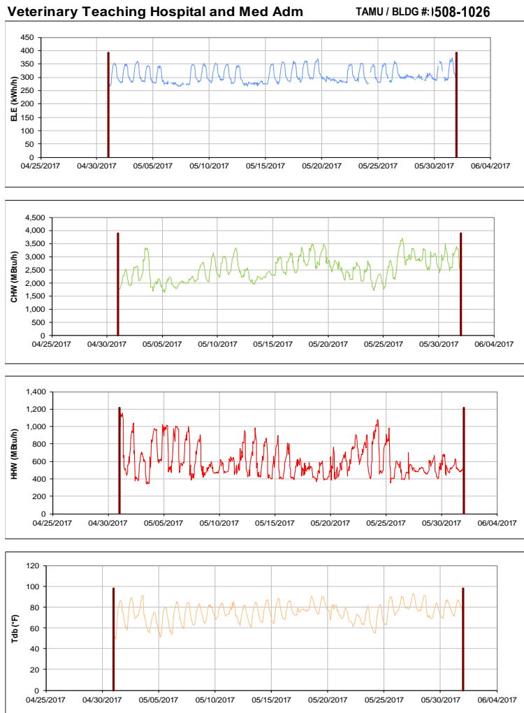
Figure III-109 Hourly Whole Building Electricity, Chilled Water, and Hot Water Consumption for Veterinary Teaching Hospital and Med Adm during the Month of May 2017 and the Corresponding Hourly Outdoor Dry Bulb Temperature for College Station, TX
