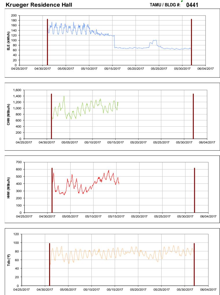
Figure III-58 Hourly Whole Building Electricity, Chilled Water, and Hot Water Consumption for Krueger Residence Hall during the Month of May 2017 and the Corresponding Hourly Outdoor Dry Bulb Temperature for College Station, TX
