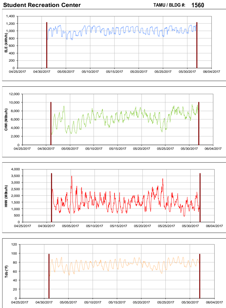
Figure III-181 Hourly Whole Building Electricity, Chilled Water, and Hot Water Consumption for Student Recreation Center during the Month of May 2017 and the Corresponding Hourly Outdoor Dry Bulb Temperature for College Station, TX
