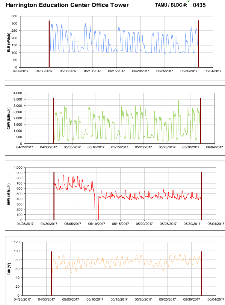
Figure III-62 Hourly Whole Building Electricity, Chilled Water, and Hot Water Consumption for Harrington Education Center Office Tower during the Month of May 2017 and the Corresponding Hourly Outdoor Dry Bulb Temperature for College Station, TX
