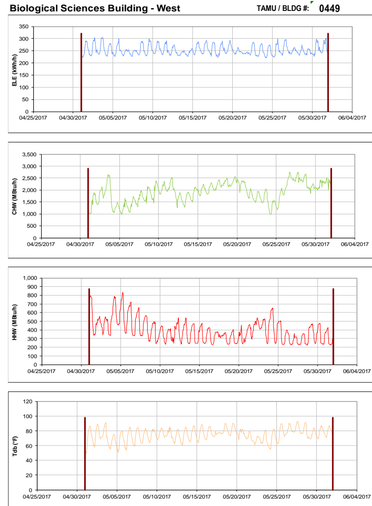
Figure III-76 Hourly Whole Building Electricity, Chilled Water, and Hot Water Consumption for Biological Sciences Building - West during the Month of May 2017 and the Corresponding Hourly Outdoor Dry Bulb Temperature for College Station, TX
