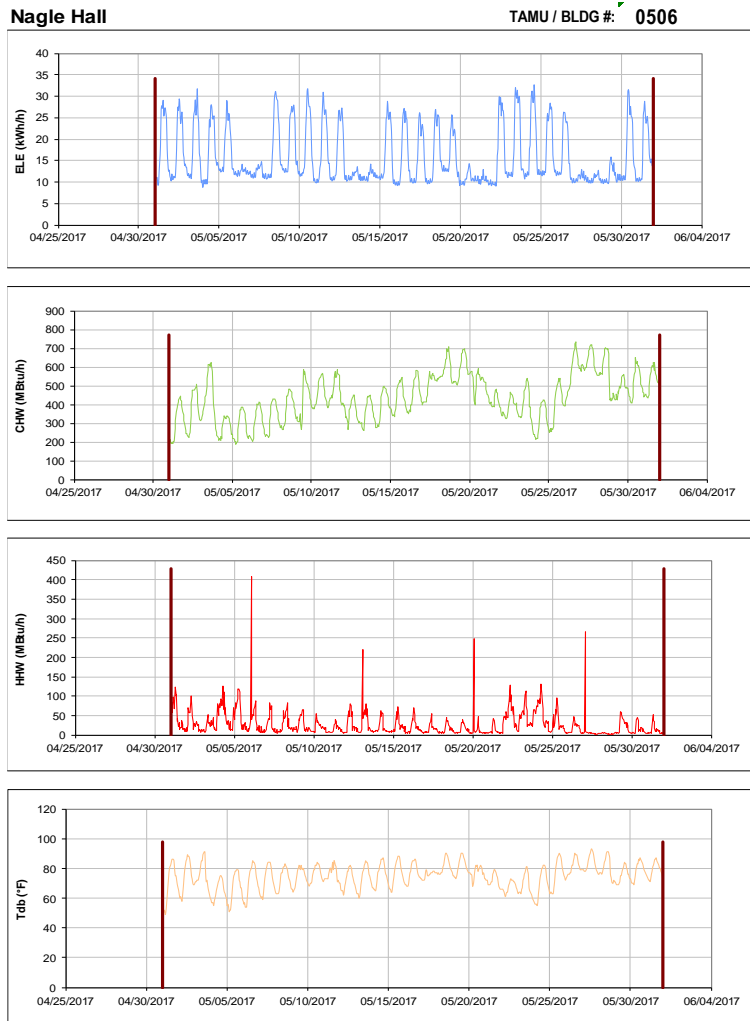
Figure III-107 Hourly Whole Building Electricity, Chilled Water, and Hot Water Consumption for Nagle Hall during the Month of May 2017 and the Corresponding Hourly Outdoor Dry Bulb Temperature for College Station, TX
