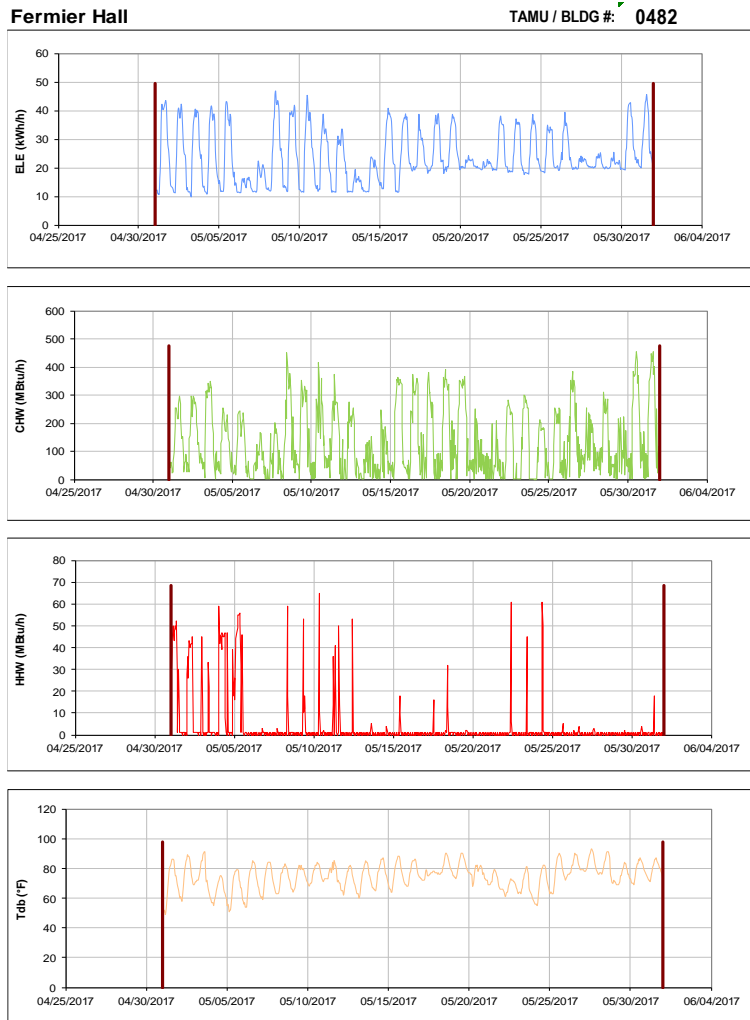
Figure III-99 Hourly Whole Building Electricity, Chilled Water, and Hot Water Consumption for Fermier Hall during the Month of May 2017 and the Corresponding Hourly Outdoor Dry Bulb Temperature for College Station, TX
