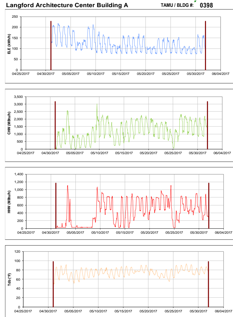
Figure III-24 Hourly Whole Building Electricity, Chilled Water, and Hot Water Consumption for Langford Architecture Center Building A during the Month of May 2017 and the Corresponding Hourly Outdoor Dry Bulb Temperature for College Station, TX
