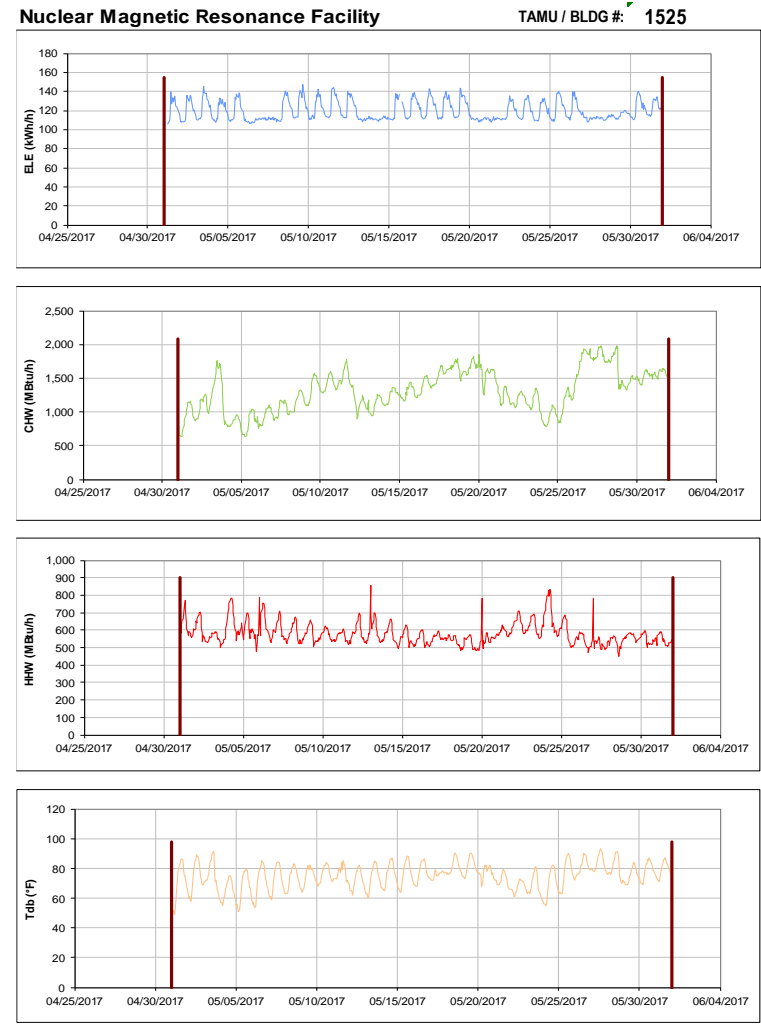
Figure III-168 Hourly Whole Building Electricity, Chilled Water, and Hot Water Consumption for Nuclear Magnetic Resonance Facility during the Month of May 2017 and the Corresponding Hourly Outdoor Dry Bulb Temperature for College Station, TX
