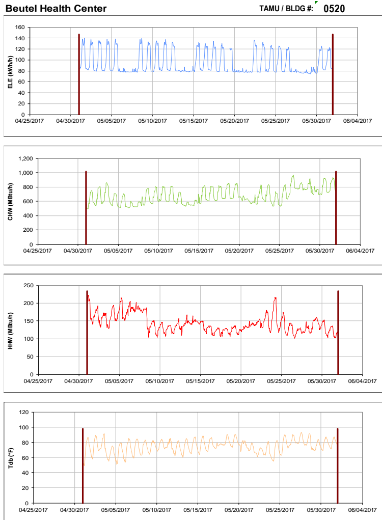
Figure III-117 Hourly Whole Building Electricity, Chilled Water, and Hot Water Consumption for Beutel Health Center during the Month of May 2017 and the Corresponding Hourly Outdoor Dry Bulb Temperature for College Station, TX
