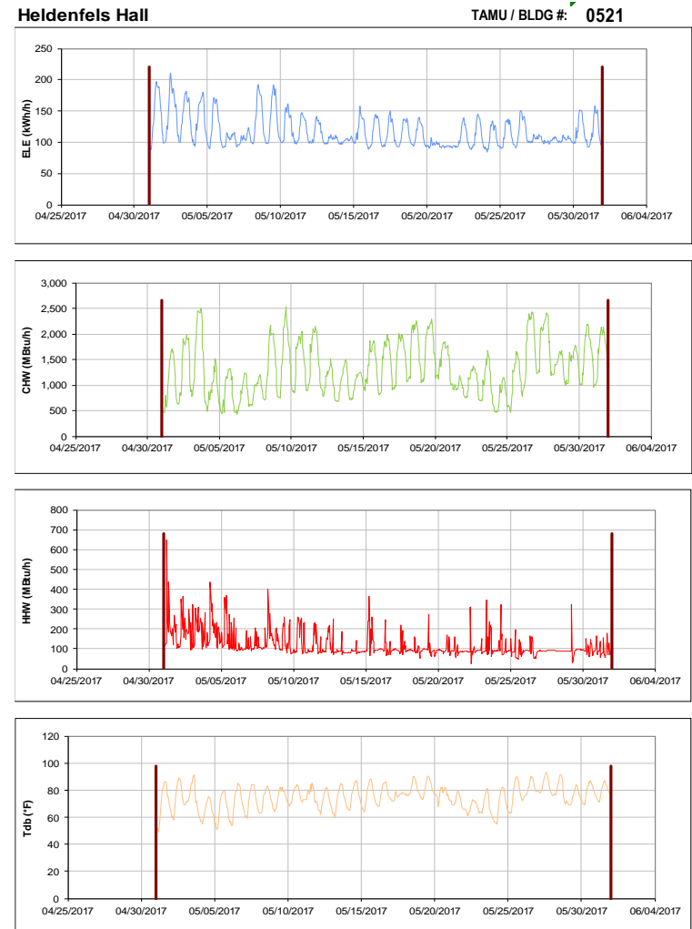
Figure III-118 Hourly Whole Building Electricity, Chilled Water, and Hot Water Consumption for Heldenfels Hall during the Month of May 2017 and the Corresponding Hourly Outdoor Dry Bulb Temperature for College Station, TX
