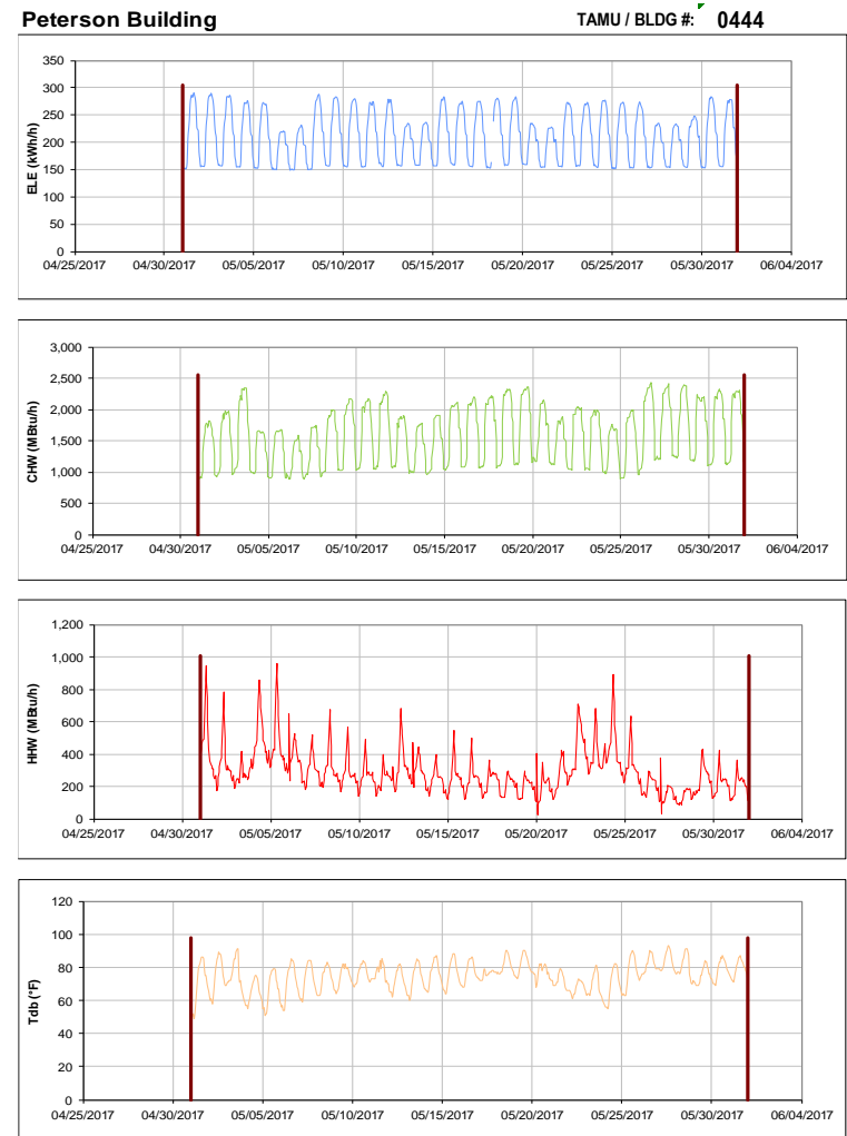
Figure III-68 Hourly Whole Building Electricity, Chilled Water, and Hot Water Consumption for Peterson Building during the Month of May 2017 and the Corresponding Hourly Outdoor Dry Bulb Temperature for College Station, TX
