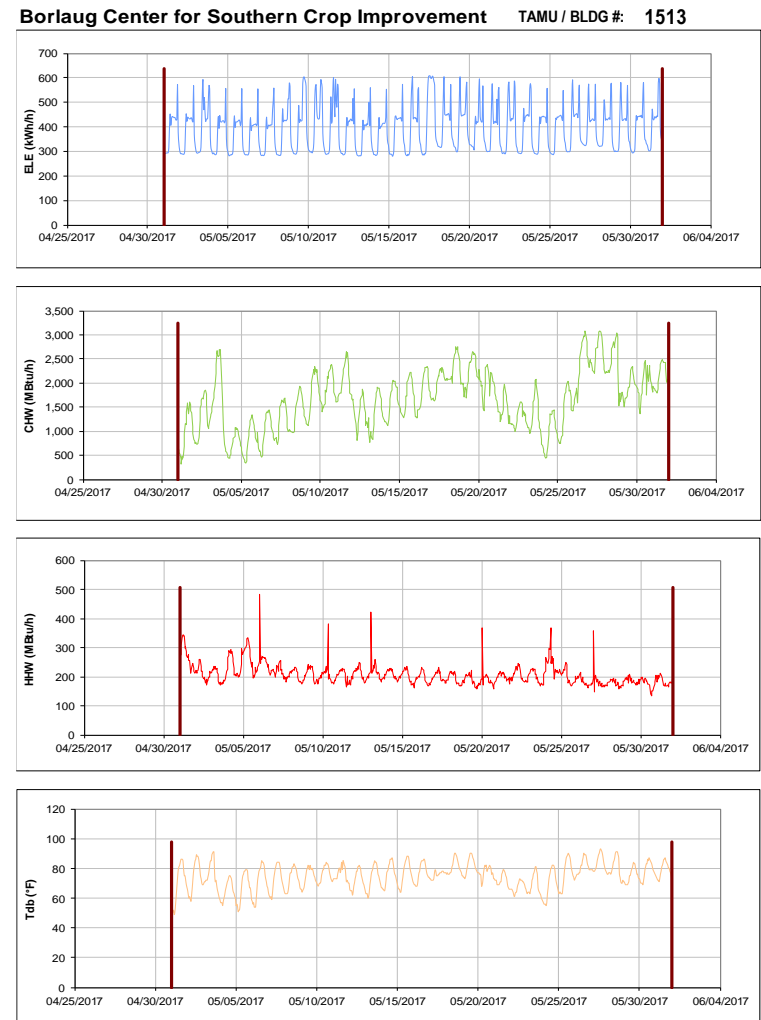
Figure III-166 Hourly Whole Building Electricity, Chilled Water, and Hot Water Consumption for Borlaug Center for Southern Crop Improvement during the Month of May 2017 and the Corresponding Hourly Outdoor Dry Bulb Temperature for College Station, TX
