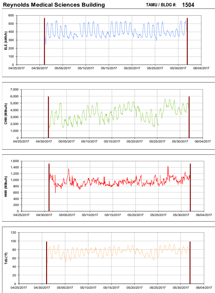
Figure III-157 Hourly Whole Building Electricity, Chilled Water, and Hot Water Consumption for Reynolds Medical Sciences Building during the Month of May 2017 and the Corresponding Hourly Outdoor Dry Bulb Temperature for College Station, TX
