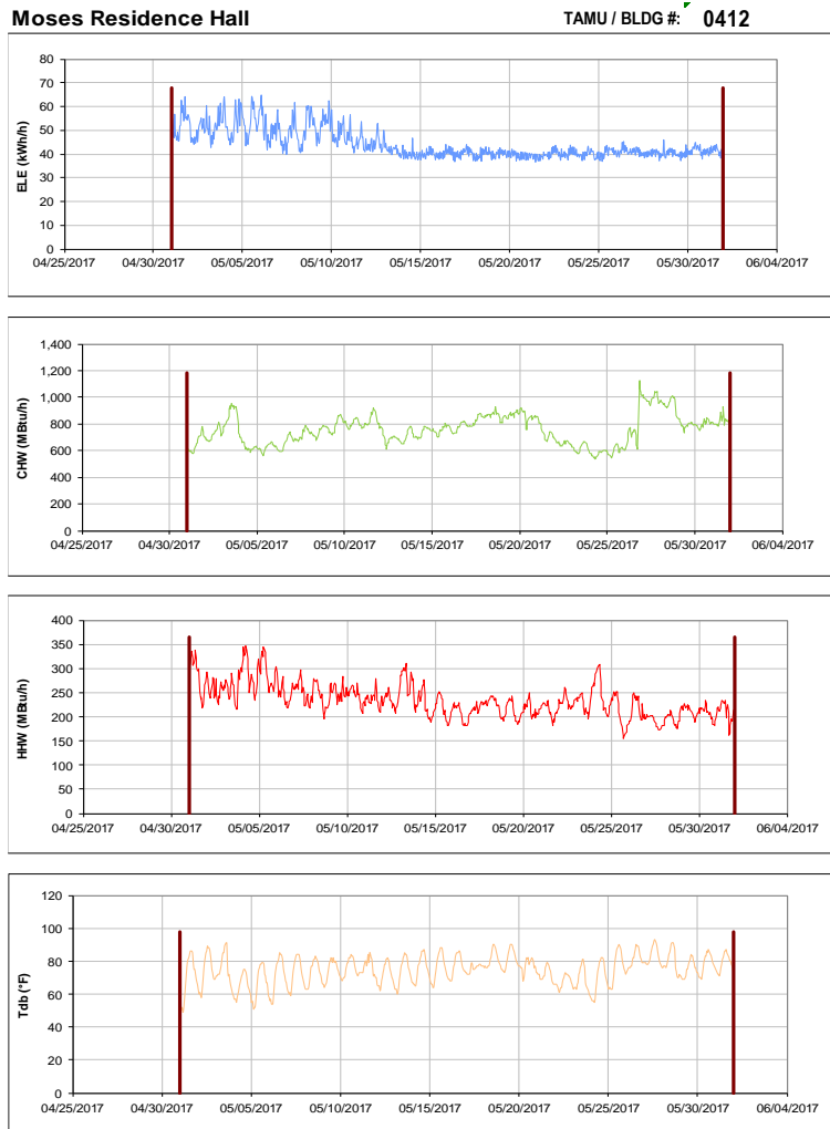
Figure III-45 Hourly Whole Building Electricity, Chilled Water, and Hot Water Consumption for Moses Residence Hall during the Month of May 2017 and the Corresponding Hourly Outdoor Dry Bulb Temperature for College Station, TX
