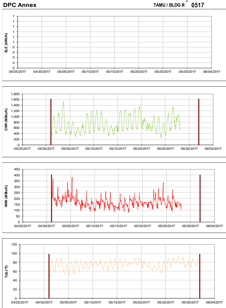
Figure III-71 Hourly Whole Building Electricity, Chilled Water, and Hot Water Consumption for DPC Annex during the Month of May 2017 and the Corresponding Hourly Outdoor Dry Bulb Temperature for College Station, TX
