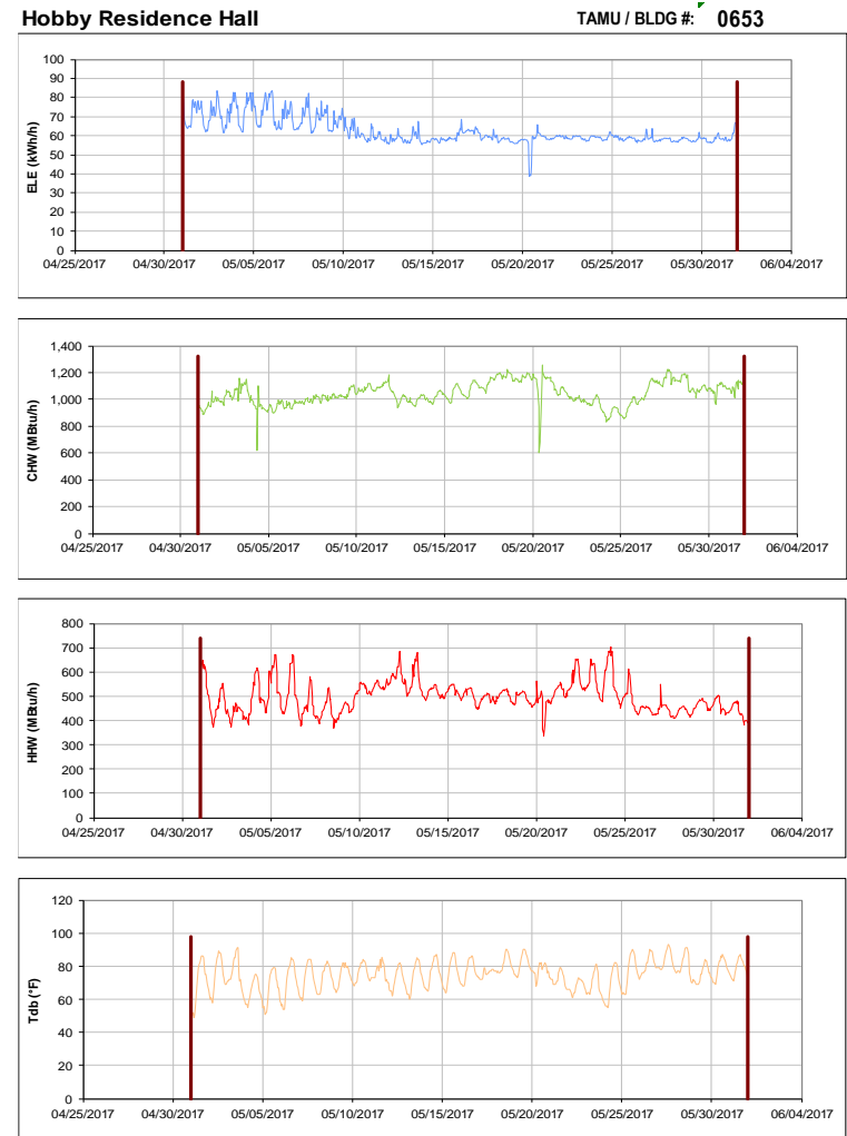
Figure III-124 Hourly Whole Building Electricity, Chilled Water, and Hot Water Consumption for Hobby Residence Hall during the Month of May 2017 and the Corresponding Hourly Outdoor Dry Bulb Temperature for College Station, TX
