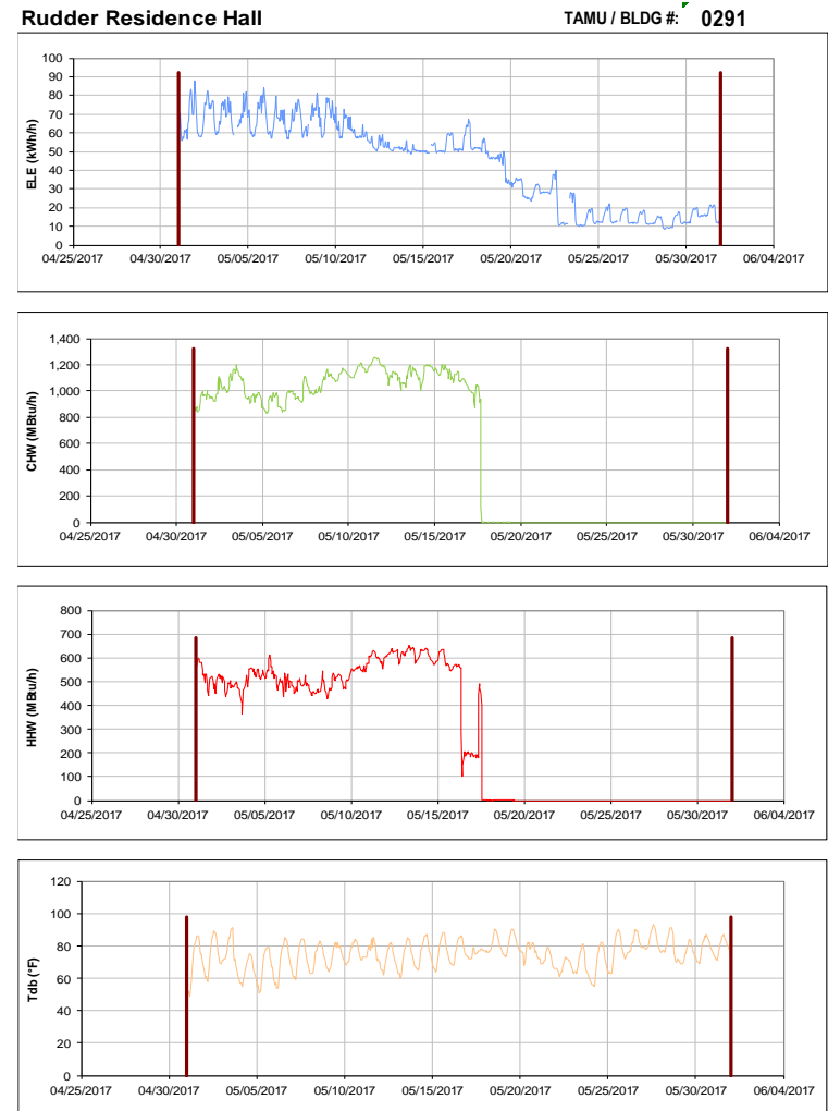
Figure III-4 Hourly Whole Building Electricity, Chilled Water, and Hot Water Consumption for Rudder Residence Hall during the Month of May 2017 and the Corresponding Hourly Outdoor Dry Bulb Temperature for College Station, TX
