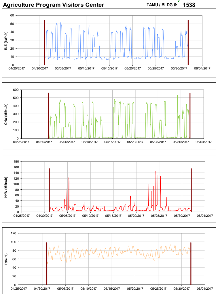
Figure III-173 Hourly Whole Building Electricity, Chilled Water, and Hot Water Consumption for Agriculture Program Visitors Center during the Month of May 2017 and the Corresponding Hourly Outdoor Dry Bulb Temperature for College Station, TX
