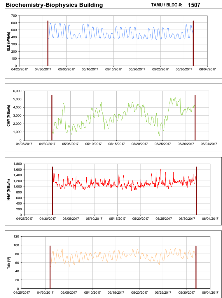
Figure III-160 Hourly Whole Building Electricity, Chilled Water, and Hot Water Consumption for Biochemistry-Biophysics Building during the Month of May 2017 and the Corresponding Hourly Outdoor Dry Bulb Temperature for College Station, TX
