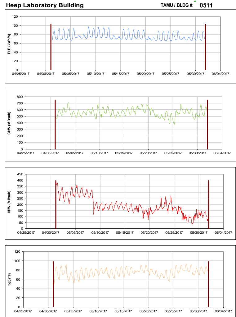
Figure III-112 Hourly Whole Building Electricity, Chilled Water, and Hot Water Consumption for Heep Laboratory Building during the Month of May 2017 and the Corresponding Hourly Outdoor Dry Bulb Temperature for College Station, TX
