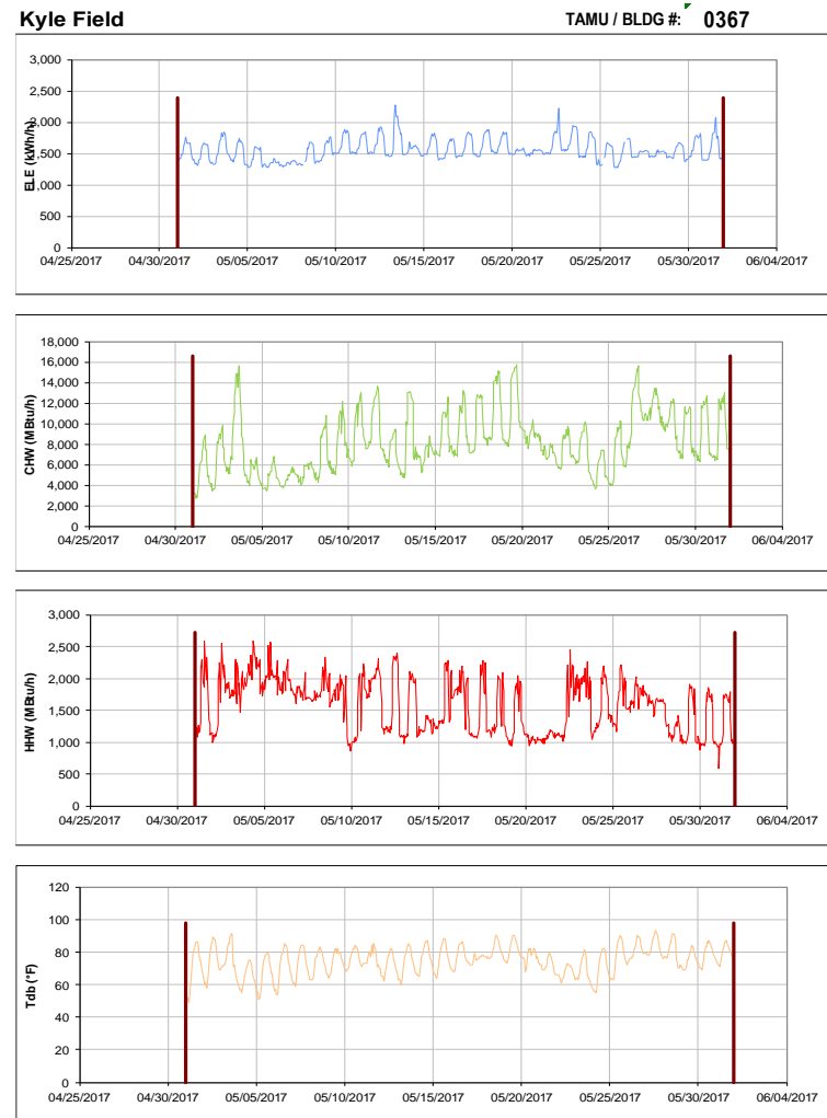
Figure III-16 Hourly Whole Building Electricity, Chilled Water, and Hot Water Consumption for Kyle Field during the Month of May 2017 and the Corresponding Hourly Outdoor Dry Bulb Temperature for College Station, TX
