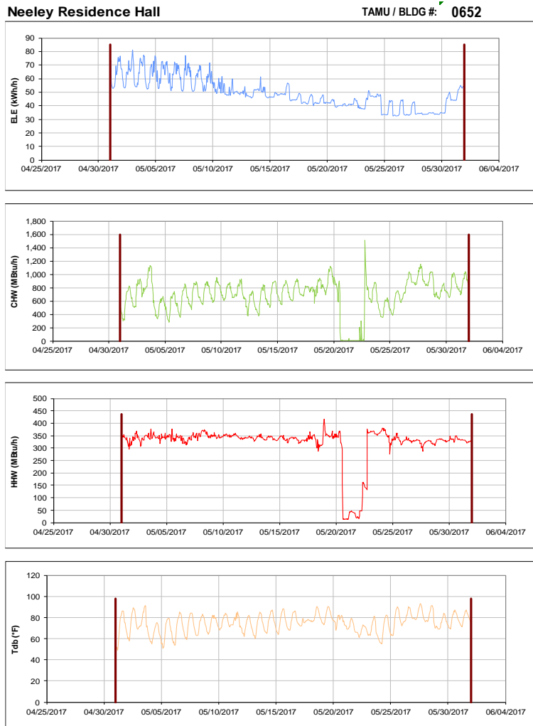
Figure III-123 Hourly Whole Building Electricity, Chilled Water, and Hot Water Consumption for Neeley Residence Hall during the Month of May 2017 and the Corresponding Hourly Outdoor Dry Bulb Temperature for College Station, TX
