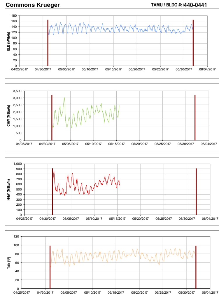
Figure III-56 Hourly Whole Building Electricity, Chilled Water, and Hot Water Consumption for Commons Krueger during the Month of May 2017 and the Corresponding Hourly Outdoor Dry Bulb Temperature for College Station, TX
