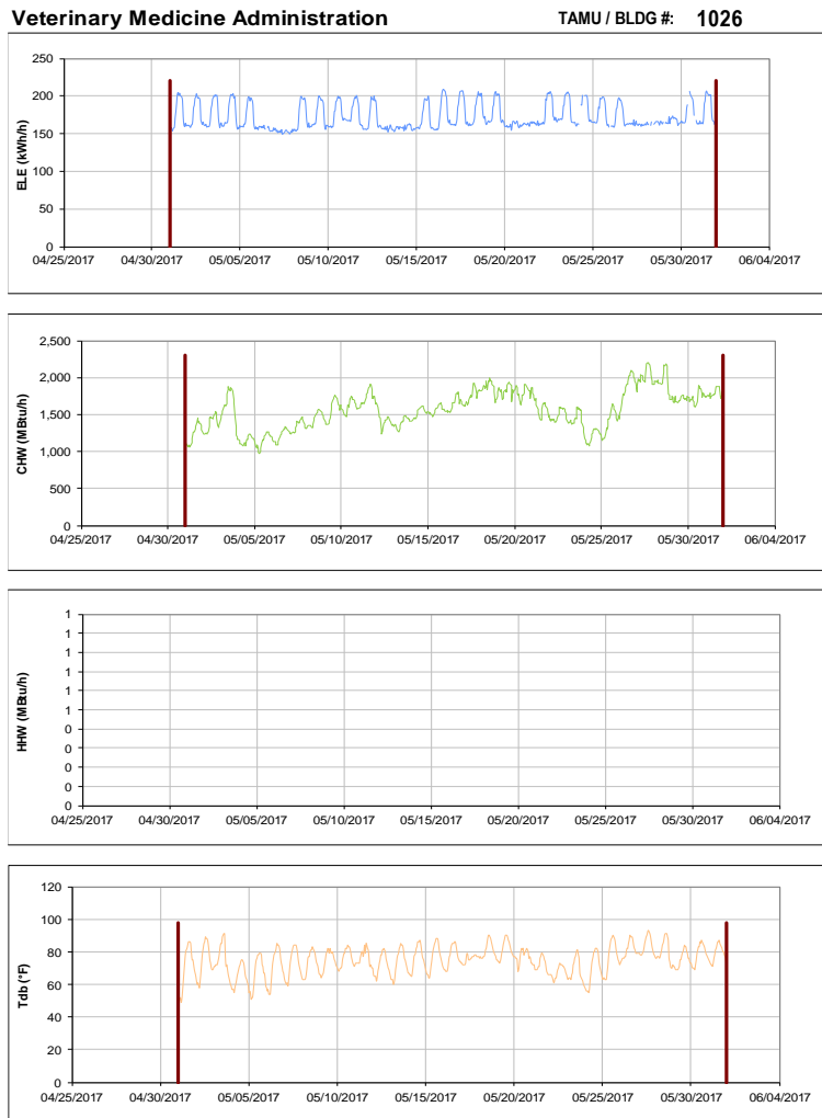
Figure III-111 Hourly Whole Building Electricity, Chilled Water, and Hot Water Consumption for Veterinary Medicine Administration during the Month of May 2017 and the Corresponding Hourly Outdoor Dry Bulb Temperature for College Station, TX
