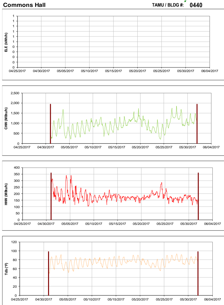
Figure III-57 Hourly Whole Building Electricity, Chilled Water, and Hot Water Consumption for Commons Hall during the Month of May 2017 and the Corresponding Hourly Outdoor Dry Bulb Temperature for College Station, TX
