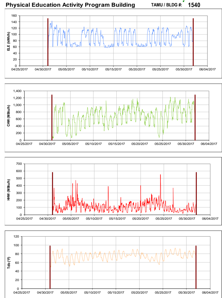
Figure III-174 Hourly Whole Building Electricity, Chilled Water, and Hot Water Consumption for Physical Education Activity Program Building during the Month of May 2017 and the Corresponding Hourly Outdoor Dry Bulb Temperature for College Station, TX
