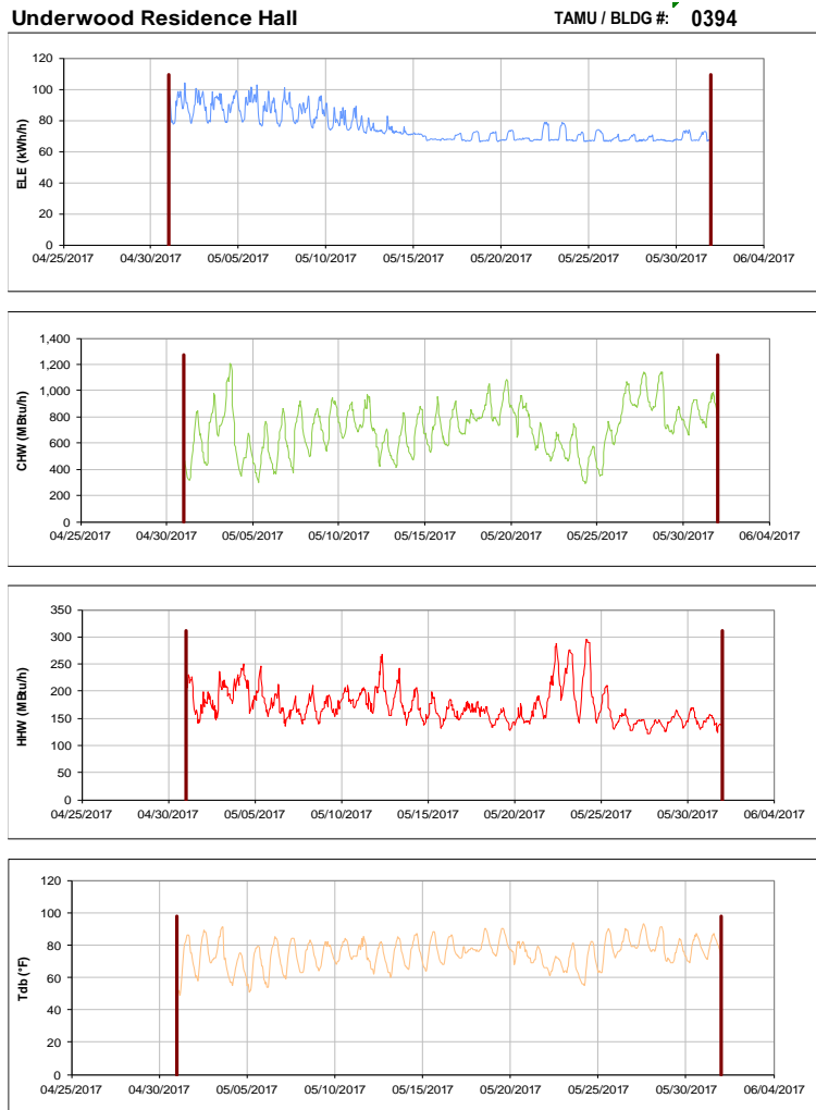
Figure III-23 Hourly Whole Building Electricity, Chilled Water, and Hot Water Consumption for Underwood Residence Hall during the Month of May 2017 and the Corresponding Hourly Outdoor Dry Bulb Temperature for College Station, TX
