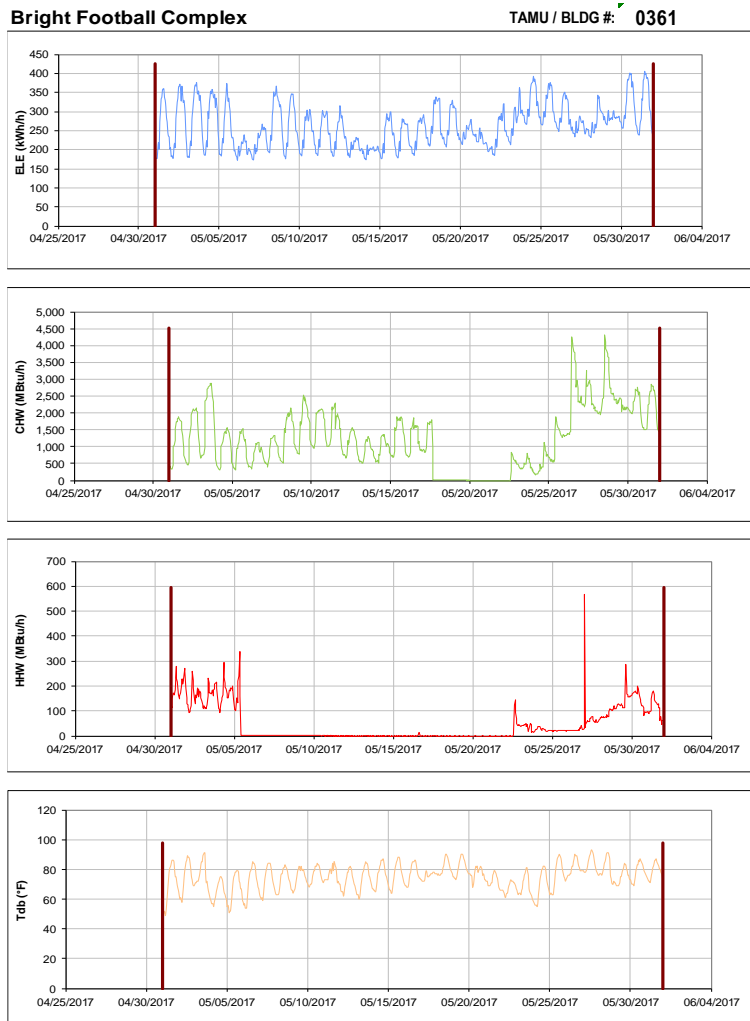
Figure III-15 Hourly Whole Building Electricity, Chilled Water, and Hot Water Consumption for Bright Football Complex during the Month of May 2017 and the Corresponding Hourly Outdoor Dry Bulb Temperature for College Station, TX
