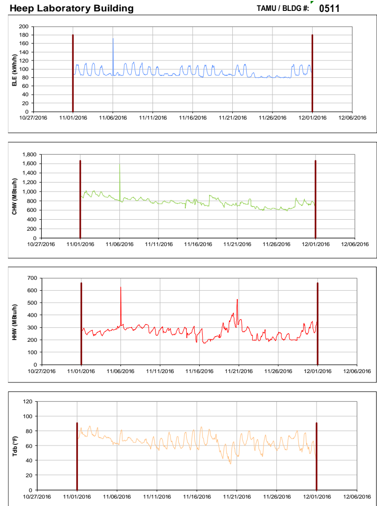
Figure III-106 Hourly Whole Building Electricity, Chilled Water, and Hot Water Consumption for Heep Laboratory Building during the Month of November 2016 and the Corresponding Hourly Outdoor Dry Bulb Temperature for College Station, TX
