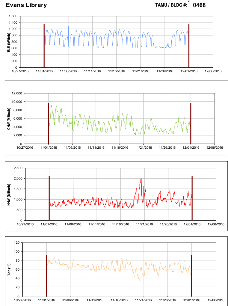
Figure III-82 Hourly Whole Building Electricity, Chilled Water, and Hot Water Consumption for Evans Library during the Month of November 2016 and the Corresponding Hourly Outdoor Dry Bulb Temperature for College Station, TX
