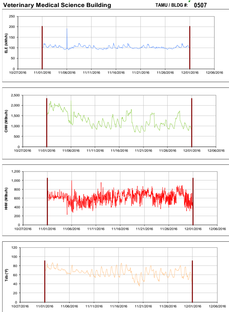
Figure III-103 Hourly Whole Building Electricity, Chilled Water, and Hot Water Consumption for Veterinary Medical Science Building during the Month of November 2016 and the Corresponding Hourly Outdoor Dry Bulb Temperature for College Station, TX
