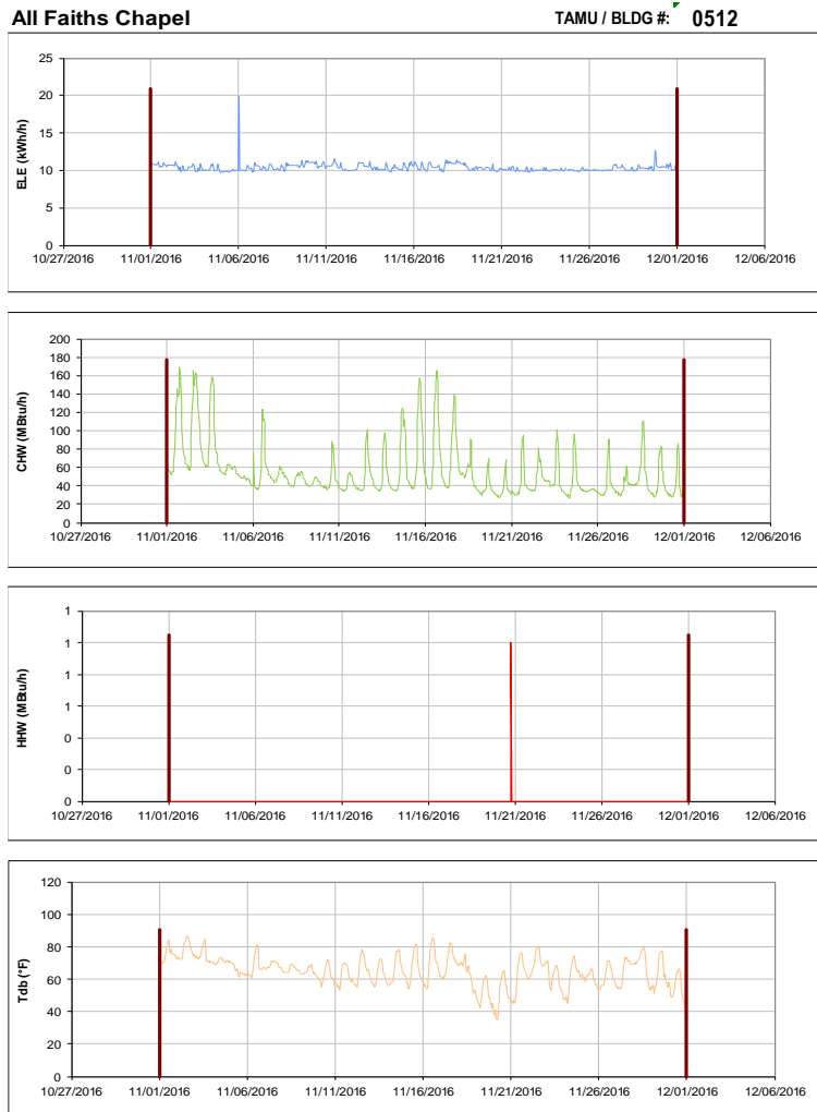
Figure III-107 Hourly Whole Building Electricity, Chilled Water, and Hot Water Consumption for All Faiths Chapel during the Month of November 2016 and the Corresponding Hourly Outdoor Dry Bulb Temperature for College Station, TX
