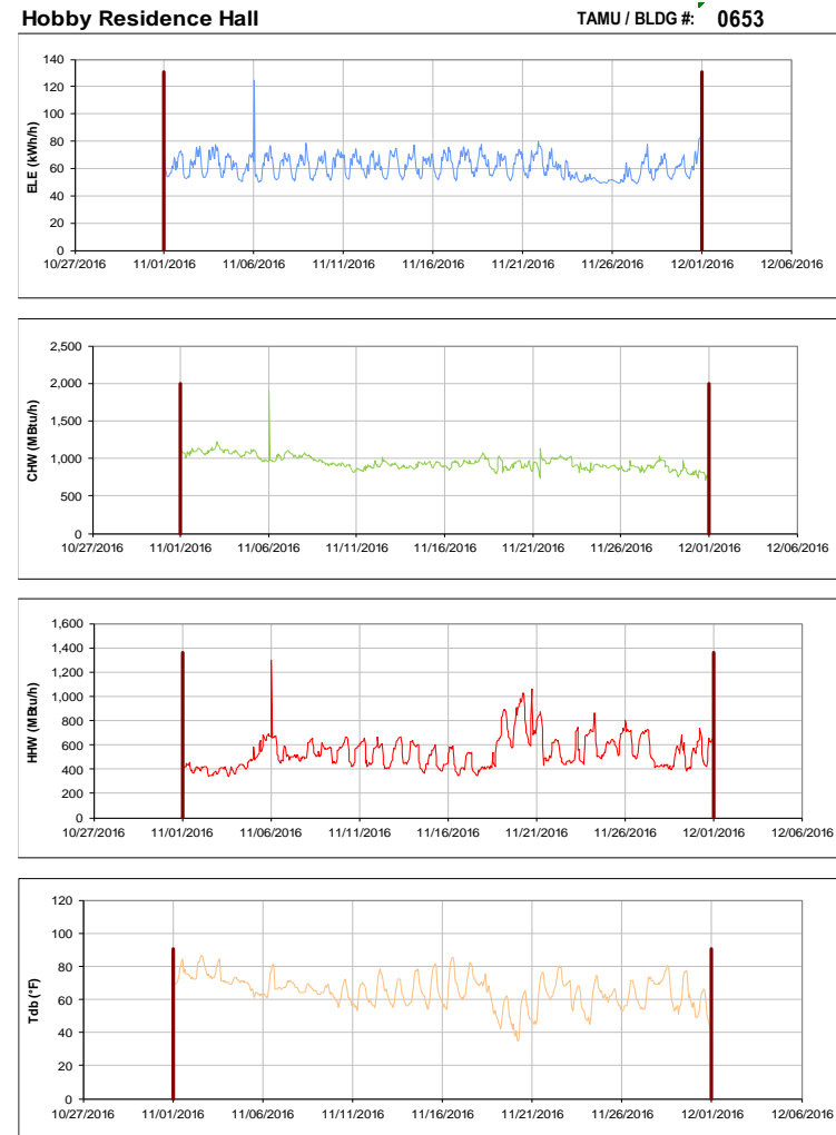
Figure III-118 Hourly Whole Building Electricity, Chilled Water, and Hot Water Consumption for Hobby Residence Hall during the Month of November 2016 and the Corresponding Hourly Outdoor Dry Bulb Temperature for College Station, TX
