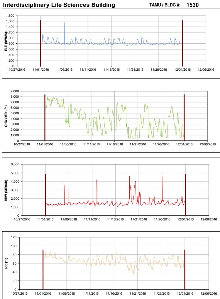
Figure III-163 Hourly Whole Building Electricity, Chilled Water, and Hot Water Consumption for Interdisciplinary Life Sciences Building during the Month of November 2016 and the Corresponding Hourly Outdoor Dry Bulb Temperature for College Station, TX
