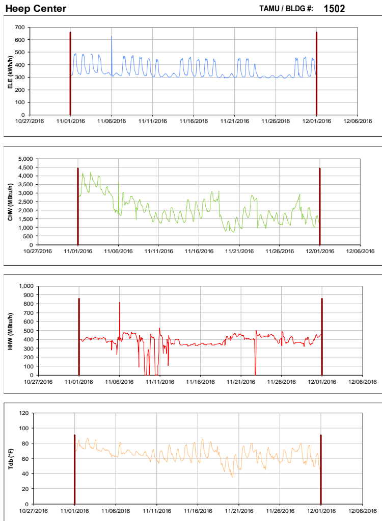
Figure III-149 Hourly Whole Building Electricity, Chilled Water, and Hot Water Consumption for Heep Center during the Month of November 2016 and the Corresponding Hourly Outdoor Dry Bulb Temperature for College Station, TX
