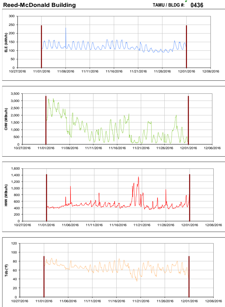
Figure III-59 Hourly Whole Building Electricity, Chilled Water, and Hot Water Consumption for Reed-McDonald Building during the Month of November 2016 and the Corresponding Hourly Outdoor Dry Bulb Temperature for College Station, TX
