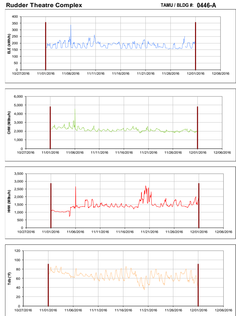
Figure III-68 Hourly Whole Building Electricity, Chilled Water, and Hot Water Consumption for Rudder Theatre Complex during the Month of November 2016 and the Corresponding Hourly Outdoor Dry Bulb Temperature for College Station, TX
