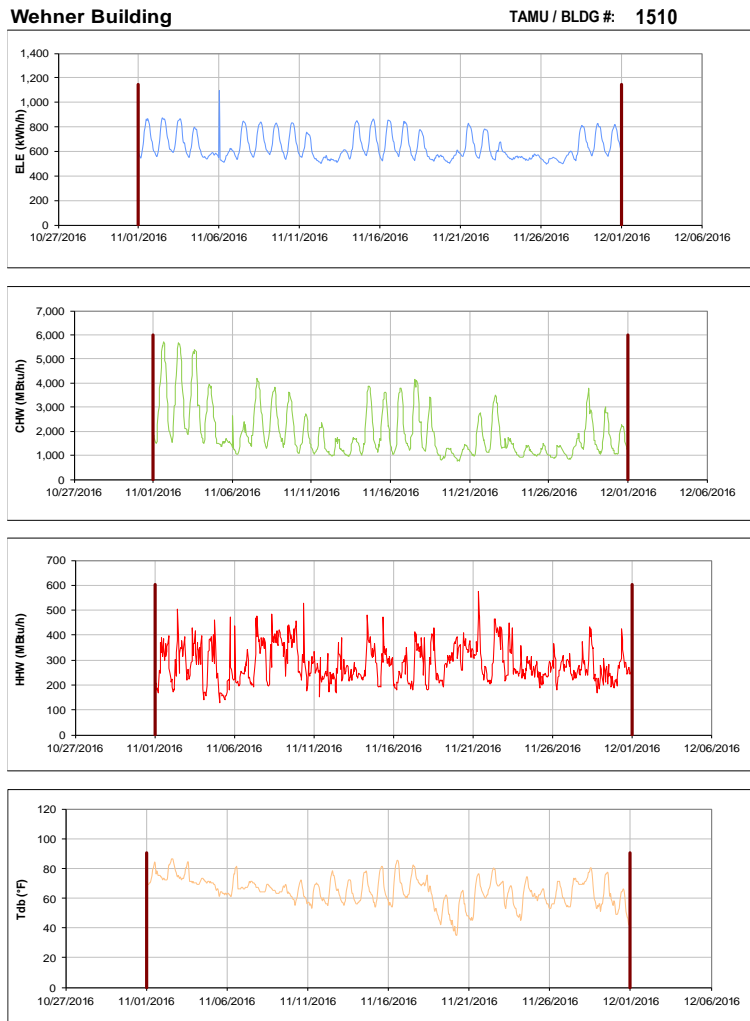
Figure III-157 Hourly Whole Building Electricity, Chilled Water, and Hot Water Consumption for Wehner Building during the Month of November 2016 and the Corresponding Hourly Outdoor Dry Bulb Temperature for College Station, TX
