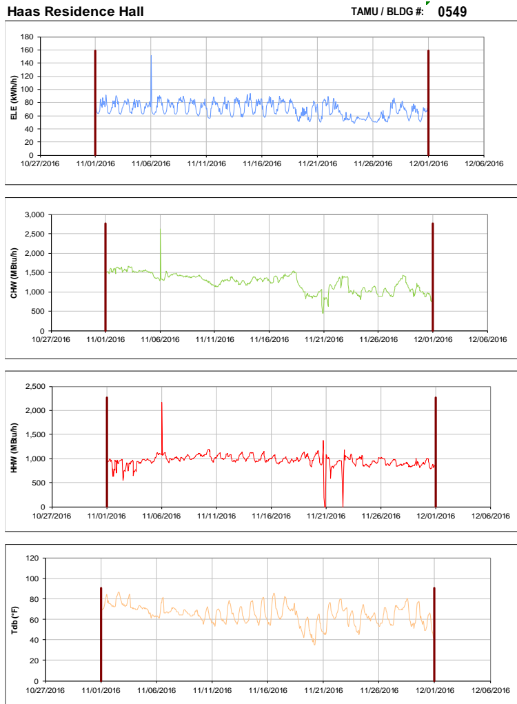
Figure III-115 Hourly Whole Building Electricity, Chilled Water, and Hot Water Consumption for Haas Residence Hall during the Month of November 2016 and the Corresponding Hourly Outdoor Dry Bulb Temperature for College Station, TX
