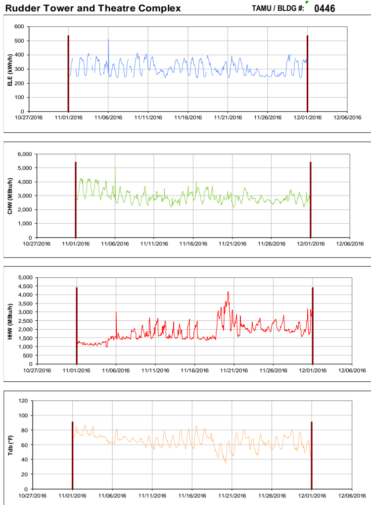
Figure III-67 Hourly Whole Building Electricity, Chilled Water, and Hot Water Consumption for Rudder Tower and Theatre Complex during the Month of November 2016 and the Corresponding Hourly Outdoor Dry Bulb Temperature for College Station, TX
