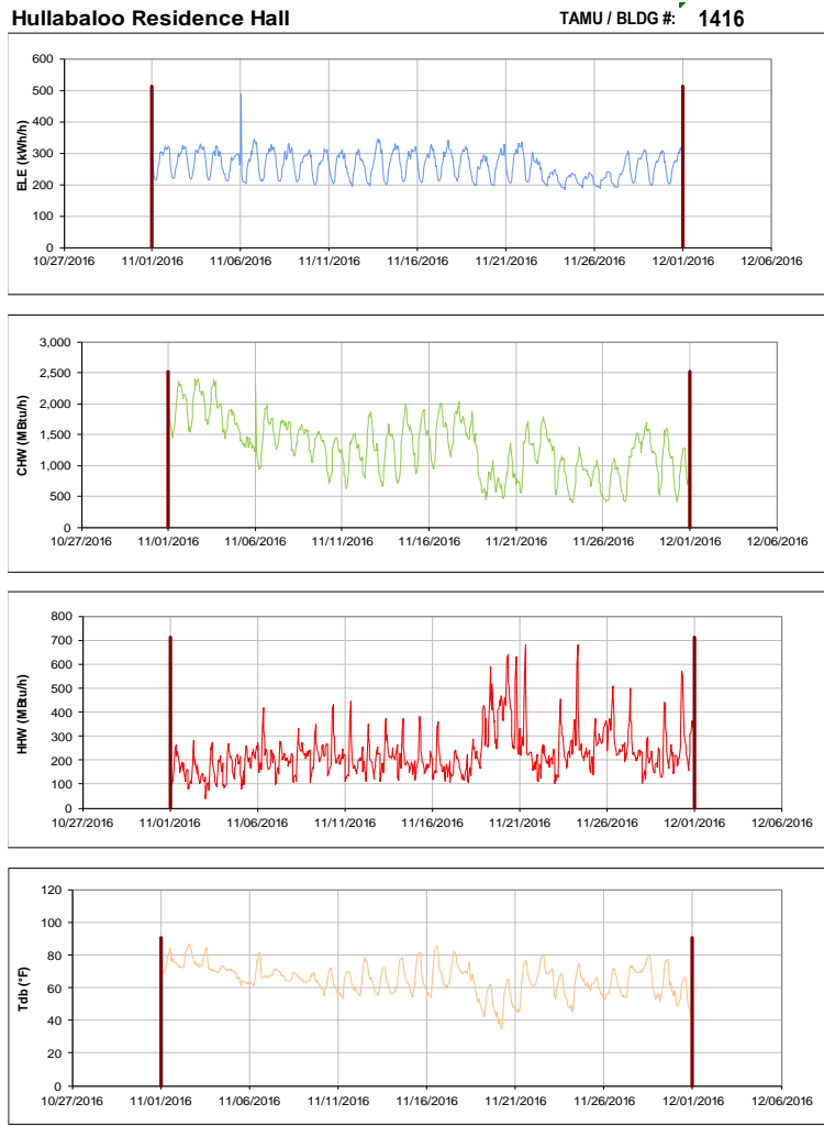
Figure III-135 Hourly Whole Building Electricity, Chilled Water, and Hot Water Consumption for Hullabaloo Residence Hall during the Month of November 2016 and the Corresponding Hourly Outdoor Dry Bulb Temperature for College Station, TX
