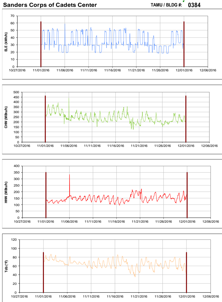
Figure III-19 Hourly Whole Building Electricity, Chilled Water, and Hot Water Consumption for Sanders Corps of Cadets Center during the Month of November 2016 and the Corresponding Hourly Outdoor Dry Bulb Temperature for College Station, TX
