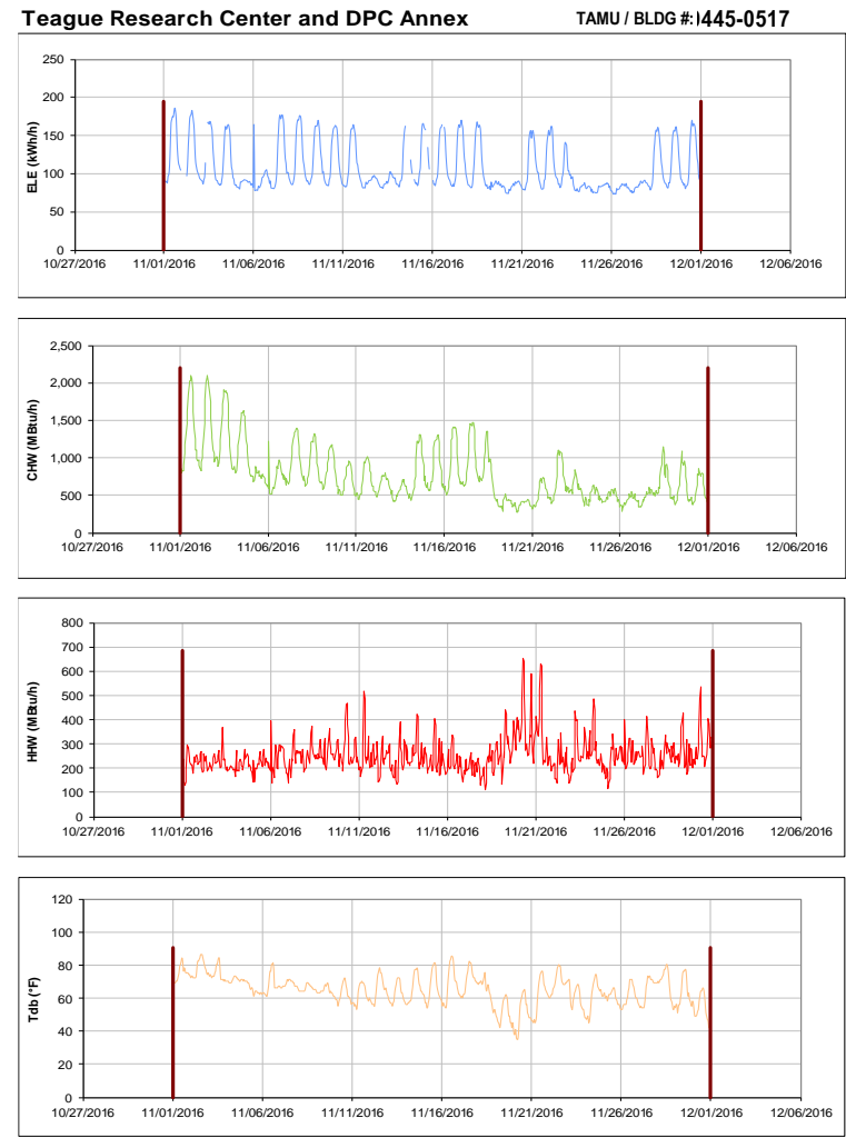
Figure III-64 Hourly Whole Building Electricity, Chilled Water, and Hot Water Consumption for Teague Research Center and DPC Annex during the Month of November 2016 and the Corresponding Hourly Outdoor Dry Bulb Temperature for College Station, TX
