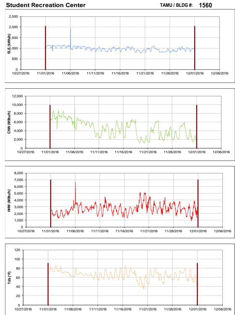
Figure III-172 Hourly Whole Building Electricity, Chilled Water, and Hot Water Consumption for Student Recreation Center during the Month of November 2016 and the Corresponding Hourly Outdoor Dry Bulb Temperature for College Station, TX
