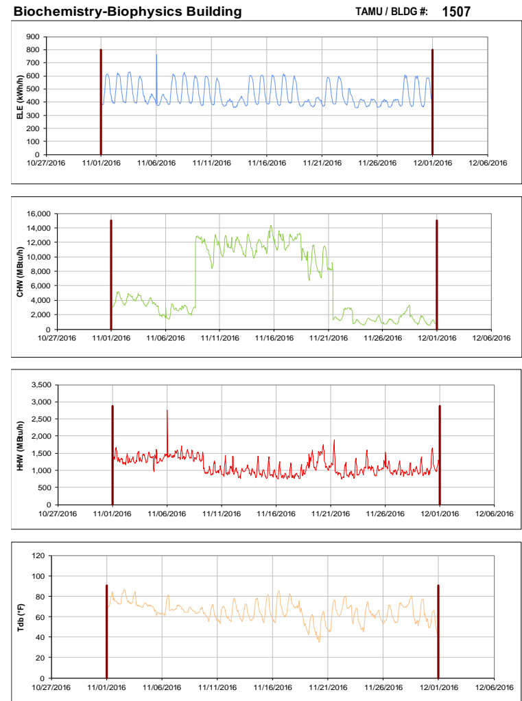
Figure III-154 Hourly Whole Building Electricity, Chilled Water, and Hot Water Consumption for Biochemistry-Biophysics Building during the Month of November 2016 and the Corresponding Hourly Outdoor Dry Bulb Temperature for College Station, TX
