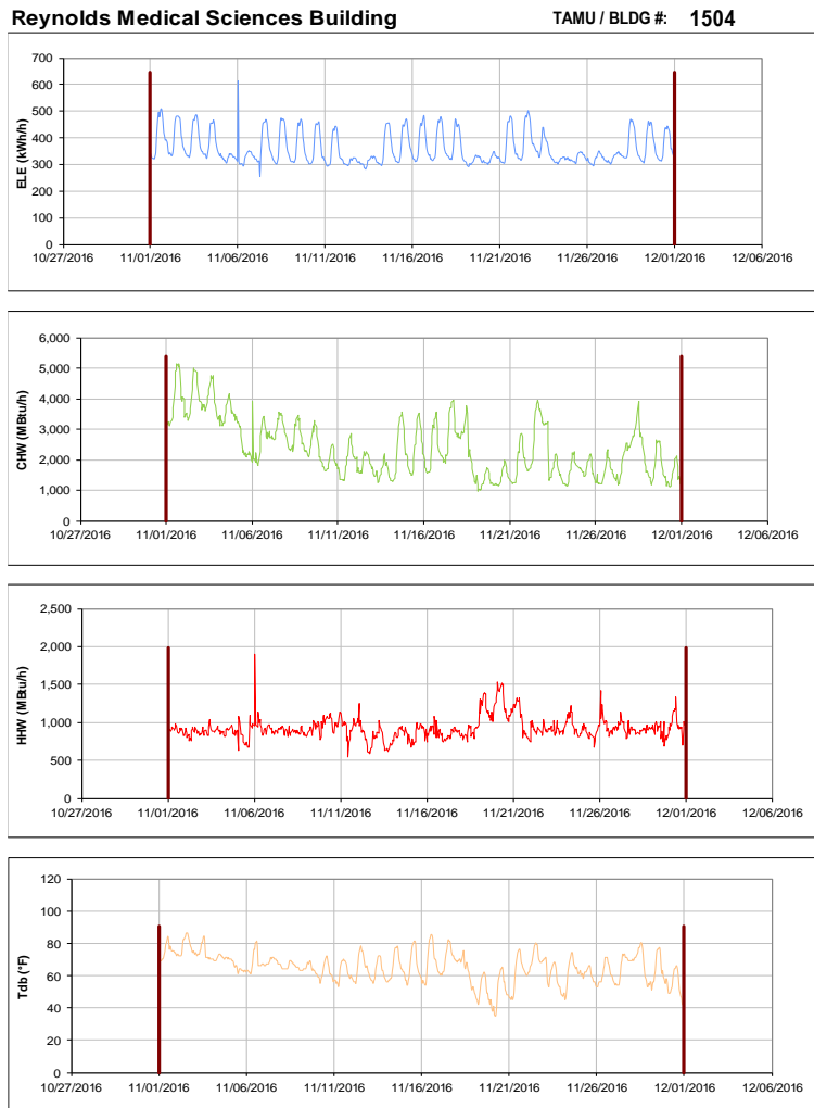
Figure III-151 Hourly Whole Building Electricity, Chilled Water, and Hot Water Consumption for Reynolds Medical Sciences Building during the Month of November 2016 and the Corresponding Hourly Outdoor Dry Bulb Temperature for College Station, TX
