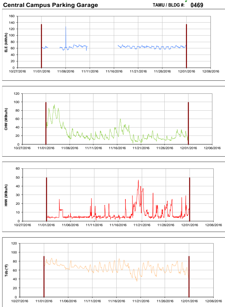
Figure III-83 Hourly Whole Building Electricity, Chilled Water, and Hot Water Consumption for Central Campus Parking Garage during the Month of November 2016 and the Corresponding Hourly Outdoor Dry Bulb Temperature for College Station, TX
