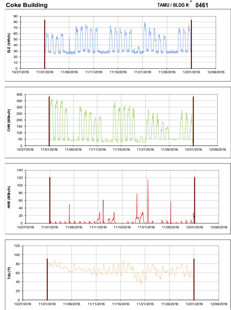
Figure III-76 Hourly Whole Building Electricity, Chilled Water, and Hot Water Consumption for Coke Building during the Month of November 2016 and the Corresponding Hourly Outdoor Dry Bulb Temperature for College Station, TX
