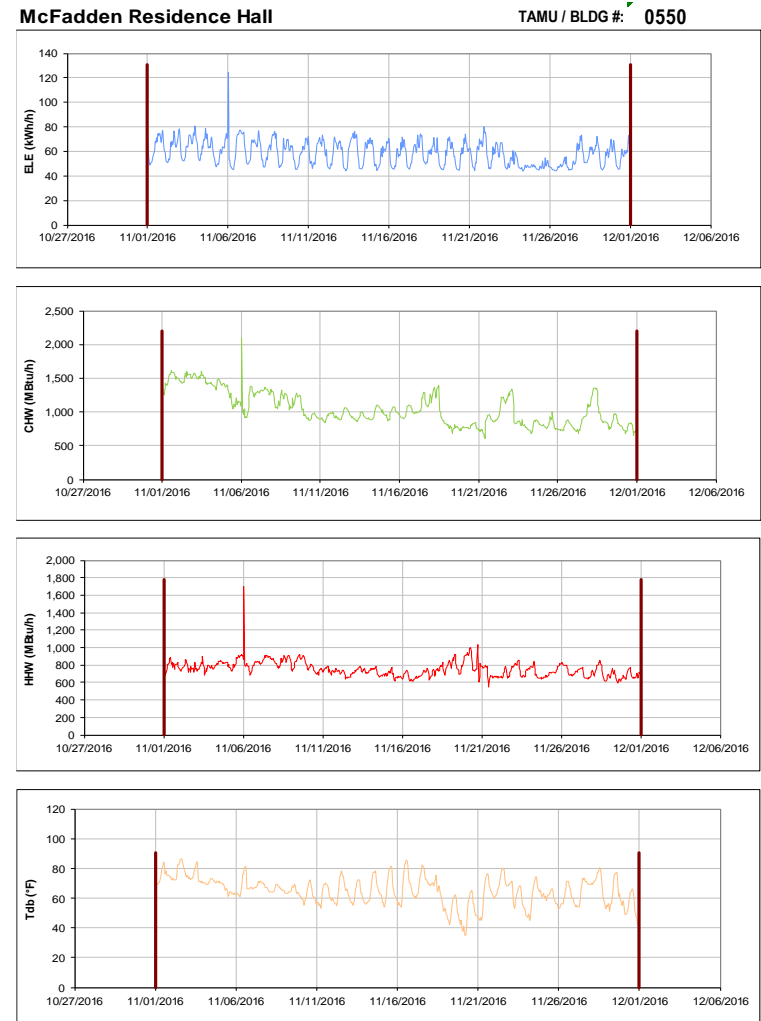
Figure III-116 Hourly Whole Building Electricity, Chilled Water, and Hot Water Consumption for McFadden Residence Hall during the Month of November 2016 and the Corresponding Hourly Outdoor Dry Bulb Temperature for College Station, TX
