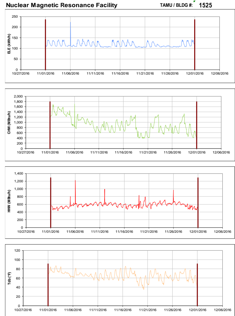
Figure III-162 Hourly Whole Building Electricity, Chilled Water, and Hot Water Consumption for Nuclear Magnetic Resonance Facility during the Month of November 2016 and the Corresponding Hourly Outdoor Dry Bulb Temperature for College Station, TX
