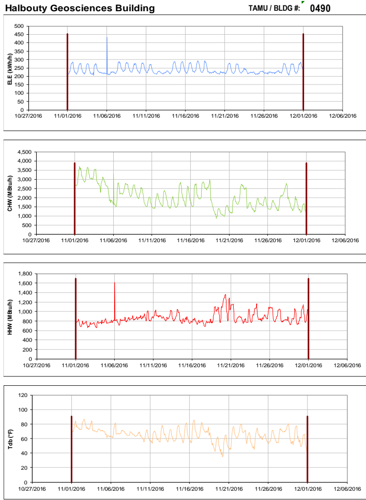
Figure III-97 Hourly Whole Building Electricity, Chilled Water, and Hot Water Consumption for Halbouty Geosciences Building during the Month of November 2016 and the Corresponding Hourly Outdoor Dry Bulb Temperature for College Station, TX
