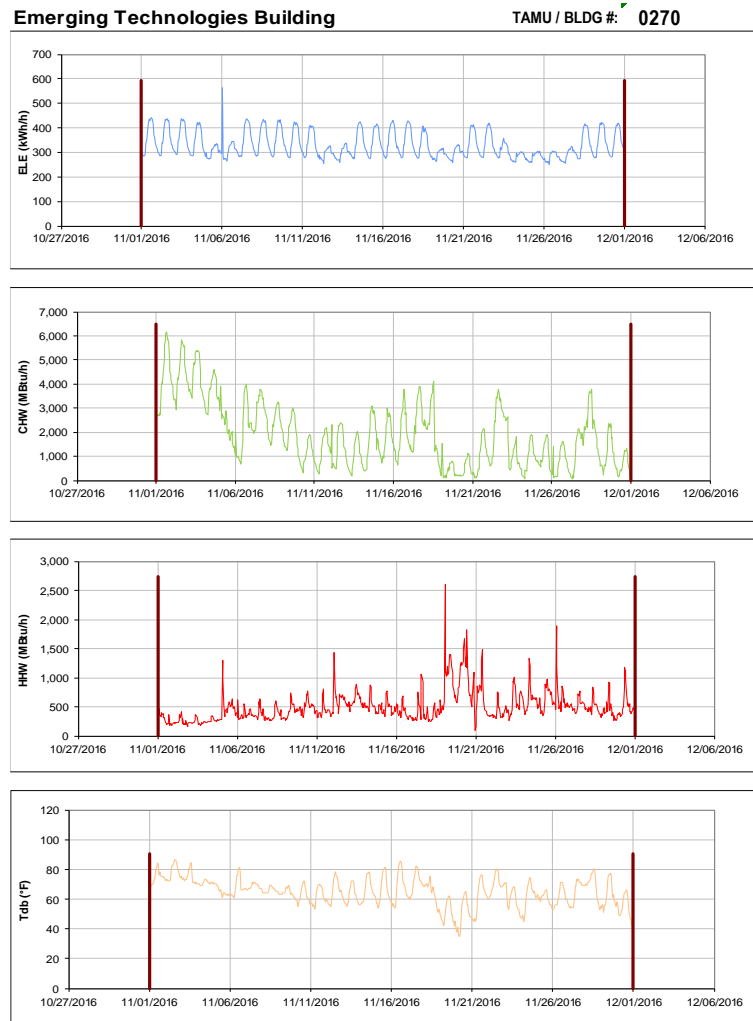
Figure III-1 Hourly Whole Building Electricity, Chilled Water, and Hot Water Consumption for Emerging Technologies Building during the Month of November 2016 and the Corresponding Hourly Outdoor Dry Bulb Temperature for College Station, TX
