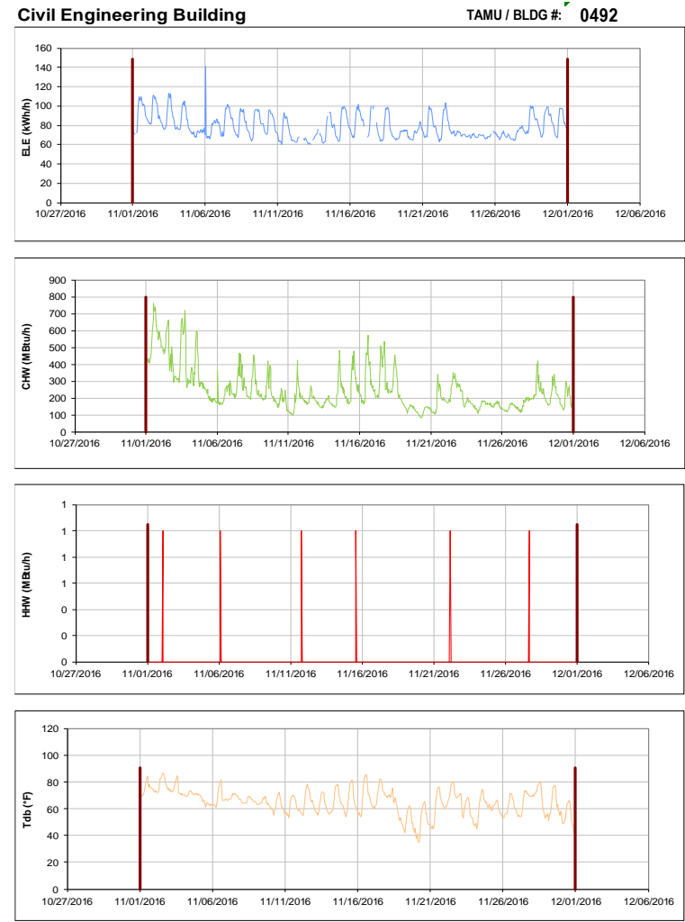
Figure III-98 Hourly Whole Building Electricity, Chilled Water, and Hot Water Consumption for Civil Engineering Building during the Month of November 2016 and the Corresponding Hourly Outdoor Dry Bulb Temperature for College Station, TX
