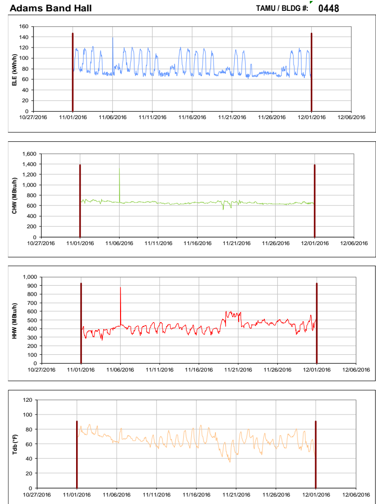
Figure III-70 Hourly Whole Building Electricity, Chilled Water, and Hot Water Consumption for Adams Band Hall during the Month of November 2016 and the Corresponding Hourly Outdoor Dry Bulb Temperature for College Station, TX
