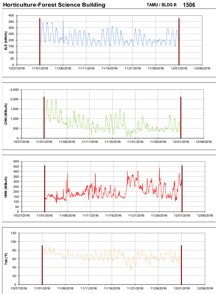
Figure III-153 Hourly Whole Building Electricity, Chilled Water, and Hot Water Consumption for Horticulture-Forest Science Building during the Month of November 2016 and the Corresponding Hourly Outdoor Dry Bulb Temperature for College Station, TX
