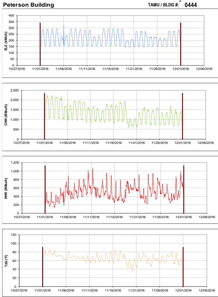
Figure III-63 Hourly Whole Building Electricity, Chilled Water, and Hot Water Consumption for Peterson Building during the Month of November 2016 and the Corresponding Hourly Outdoor Dry Bulb Temperature for College Station, TX
