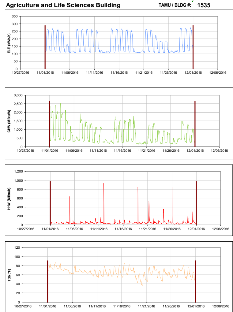
Figure III-164 Hourly Whole Building Electricity, Chilled Water, and Hot Water Consumption for Agriculture and Life Sciences Building during the Month of November 2016 and the Corresponding Hourly Outdoor Dry Bulb Temperature for College Station, TX
