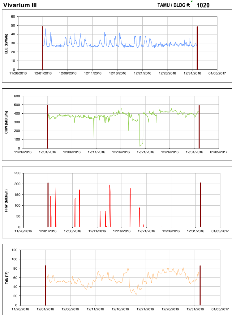
Figure III-125 Hourly Whole Building Electricity, Chilled Water, and Hot Water Consumption for Vivarium III during the Month of December 2016 and the Corresponding Hourly Outdoor Dry Bulb Temperature for College Station, TX
