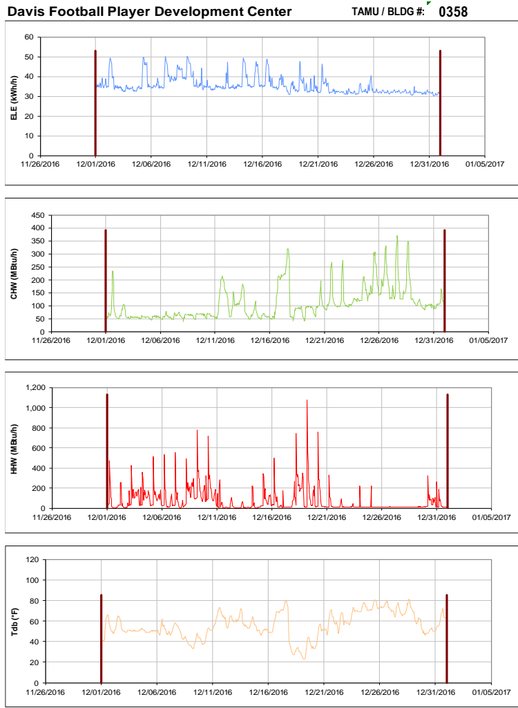
Figure III-11 Hourly Whole Building Electricity, Chilled Water, and Hot Water Consumption for Davis Football Player Development Center during the Month of December 2016 and the Corresponding Hourly Outdoor Dry Bulb Temperature for College Station, TX
