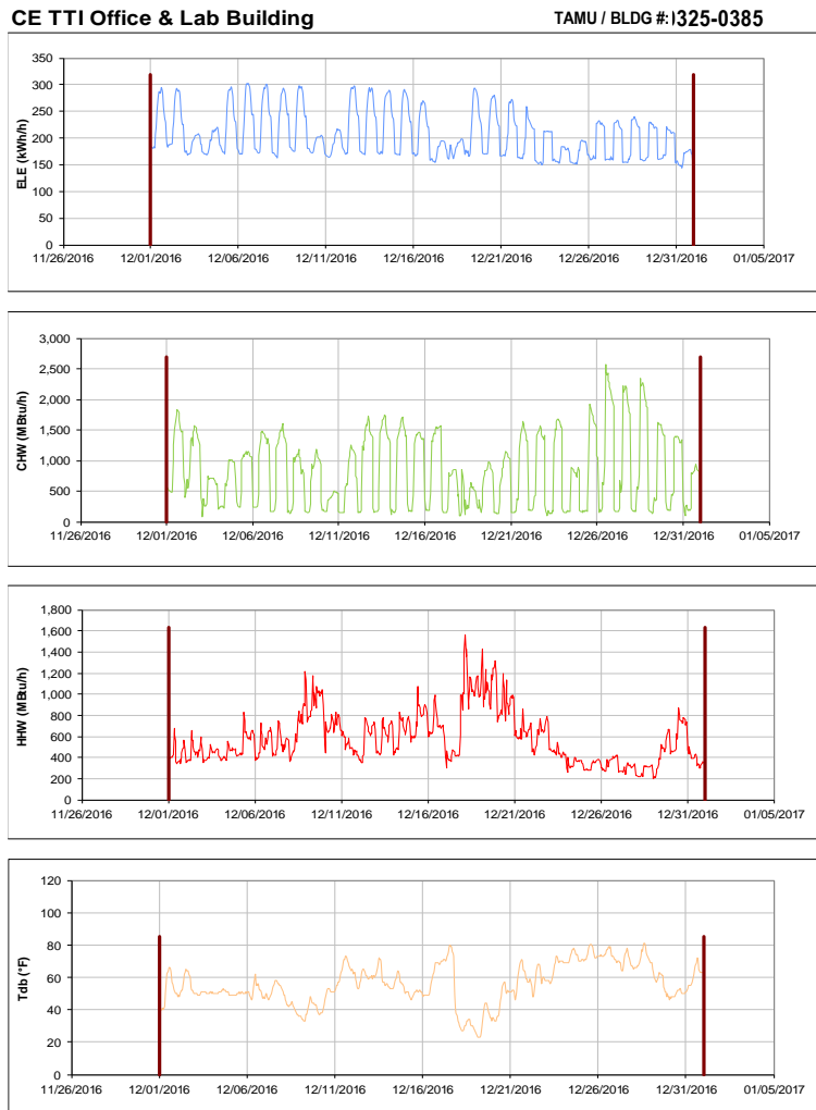
Figure III-9 Hourly Whole Building Electricity, Chilled Water, and Hot Water Consumption for CE TTI Office & Lab Building during the Month of December 2016 and the Corresponding Hourly Outdoor Dry Bulb Temperature for College Station, TX
