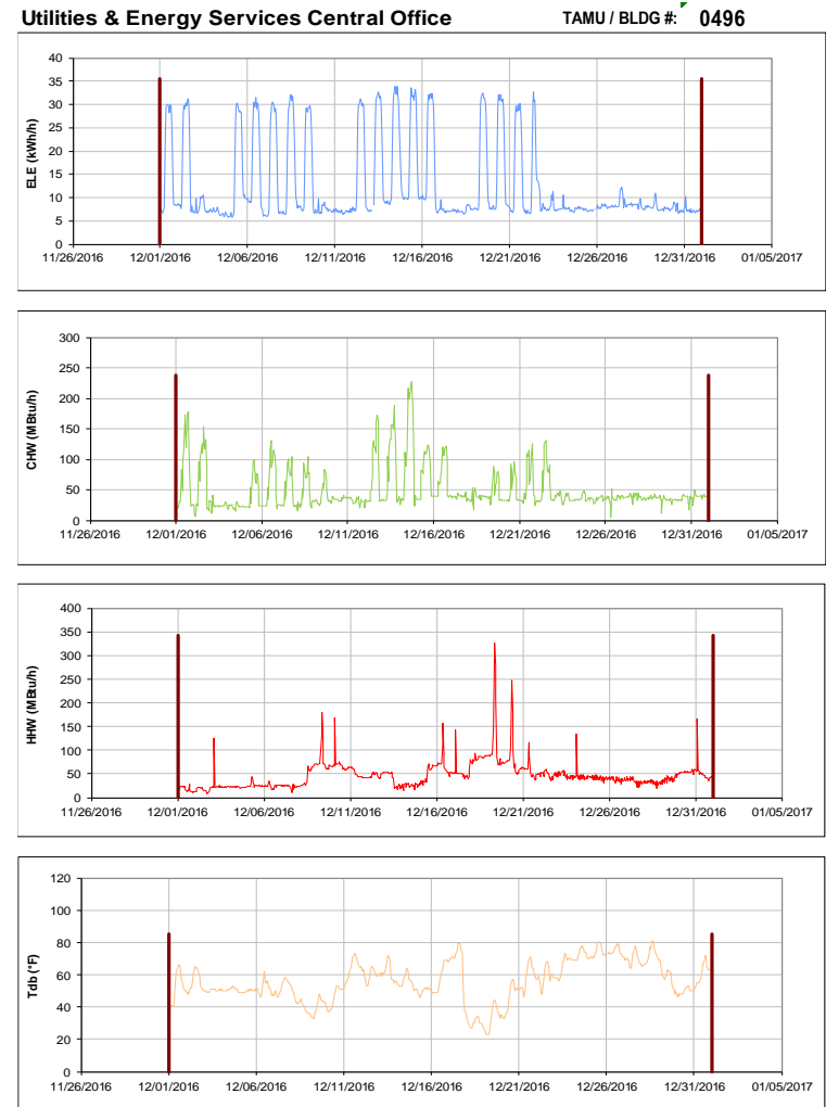
Figure III-100 Hourly Whole Building Electricity, Chilled Water, and Hot Water Consumption for Utilities & Energy Services Central Office during the Month of December 2016 and the Corresponding Hourly Outdoor Dry Bulb Temperature for College Station, TX
