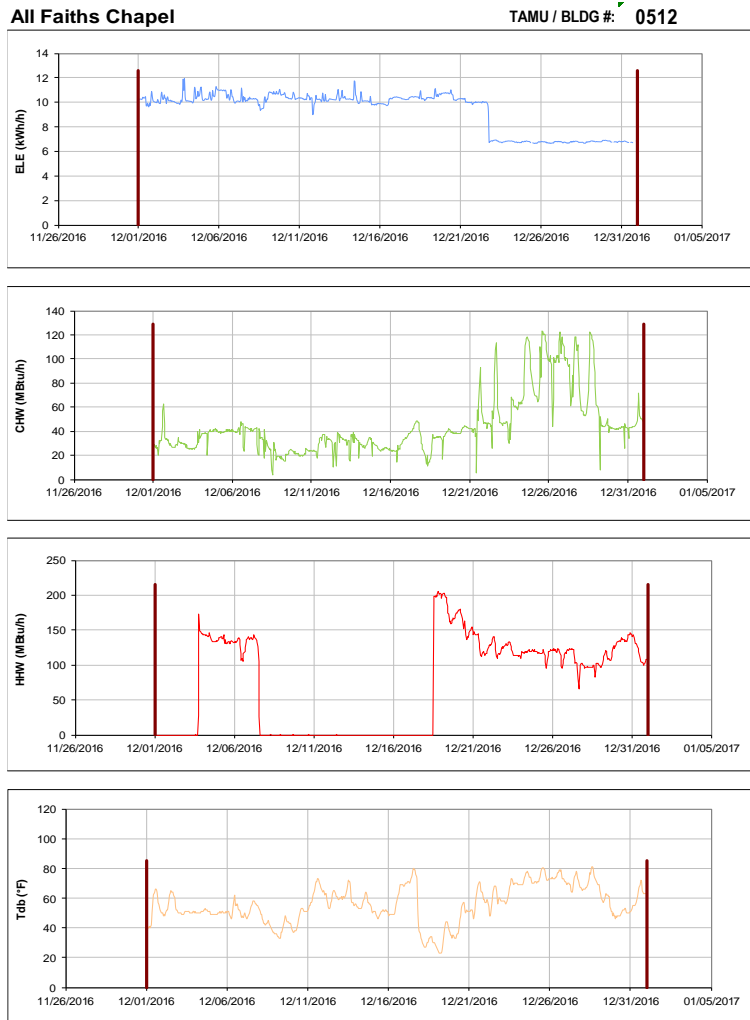
Figure III-107 Hourly Whole Building Electricity, Chilled Water, and Hot Water Consumption for All Faiths Chapel during the Month of December 2016 and the Corresponding Hourly Outdoor Dry Bulb Temperature for College Station, TX
