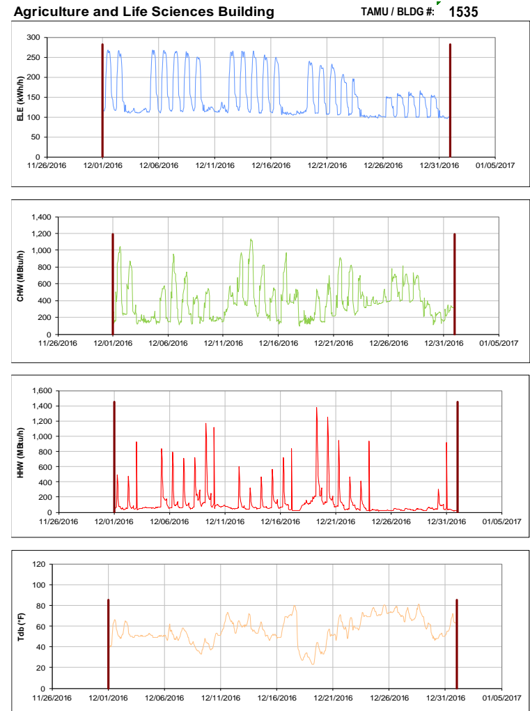
Figure III-164 Hourly Whole Building Electricity, Chilled Water, and Hot Water Consumption for Agriculture and Life Sciences Building during the Month of December 2016 and the Corresponding Hourly Outdoor Dry Bulb Temperature for College Station, TX
