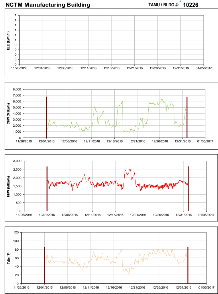
Figure III-196 Hourly Whole Building Electricity, Chilled Water, and Hot Water Consumption for NCTM Manufacturing Building during the Month of December 2016 and the Corresponding Hourly Outdoor Dry Bulb Temperature for College Station, TX
