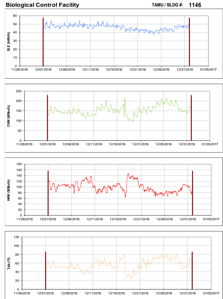
Figure III-130 Hourly Whole Building Electricity, Chilled Water, and Hot Water Consumption for Biological Control Facility during the Month of December 2016 and the Corresponding Hourly Outdoor Dry Bulb Temperature for College Station, TX
