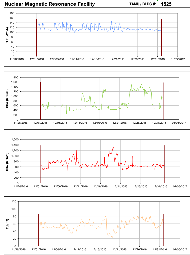
Figure III-162 Hourly Whole Building Electricity, Chilled Water, and Hot Water Consumption for Nuclear Magnetic Resonance Facility during the Month of December 2016 and the Corresponding Hourly Outdoor Dry Bulb Temperature for College Station, TX
