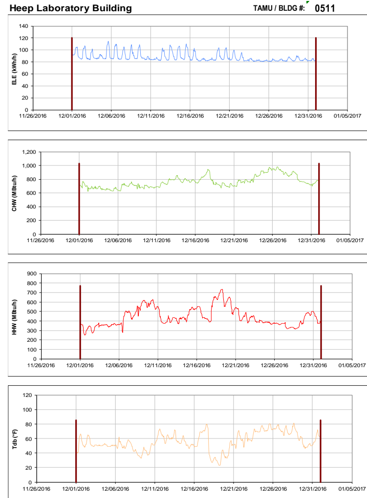
Figure III-106 Hourly Whole Building Electricity, Chilled Water, and Hot Water Consumption for Heep Laboratory Building during the Month of December 2016 and the Corresponding Hourly Outdoor Dry Bulb Temperature for College Station, TX
