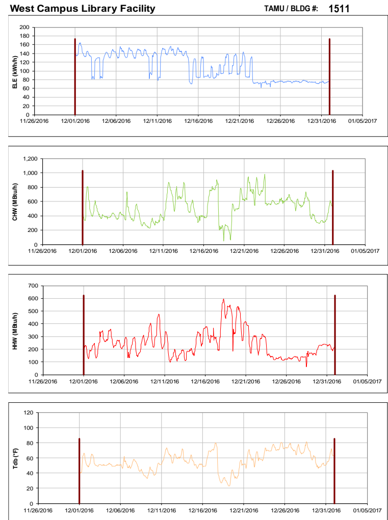
Figure III-158 Hourly Whole Building Electricity, Chilled Water, and Hot Water Consumption for West Campus Library Facility during the Month of December 2016 and the Corresponding Hourly Outdoor Dry Bulb Temperature for College Station, TX
