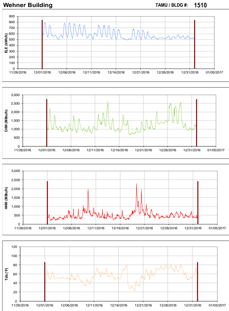
Figure III-157 Hourly Whole Building Electricity, Chilled Water, and Hot Water Consumption for Wehner Building during the Month of December 2016 and the Corresponding Hourly Outdoor Dry Bulb Temperature for College Station, TX
