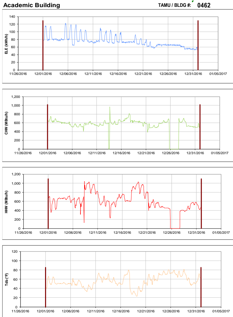
Figure III-77 Hourly Whole Building Electricity, Chilled Water, and Hot Water Consumption for Academic Building during the Month of December 2016 and the Corresponding Hourly Outdoor Dry Bulb Temperature for College Station, TX
