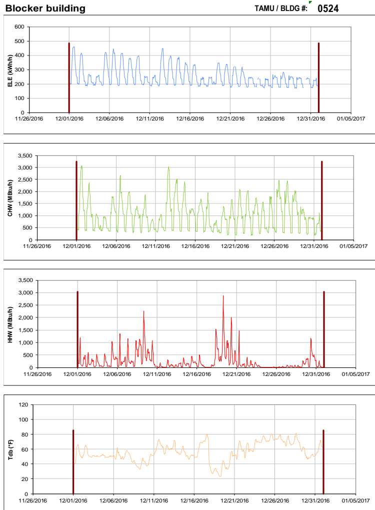
Figure III-113 Hourly Whole Building Electricity, Chilled Water, and Hot Water Consumption for Blocker building during the Month of December 2016 and the Corresponding Hourly Outdoor Dry Bulb Temperature for College Station, TX
