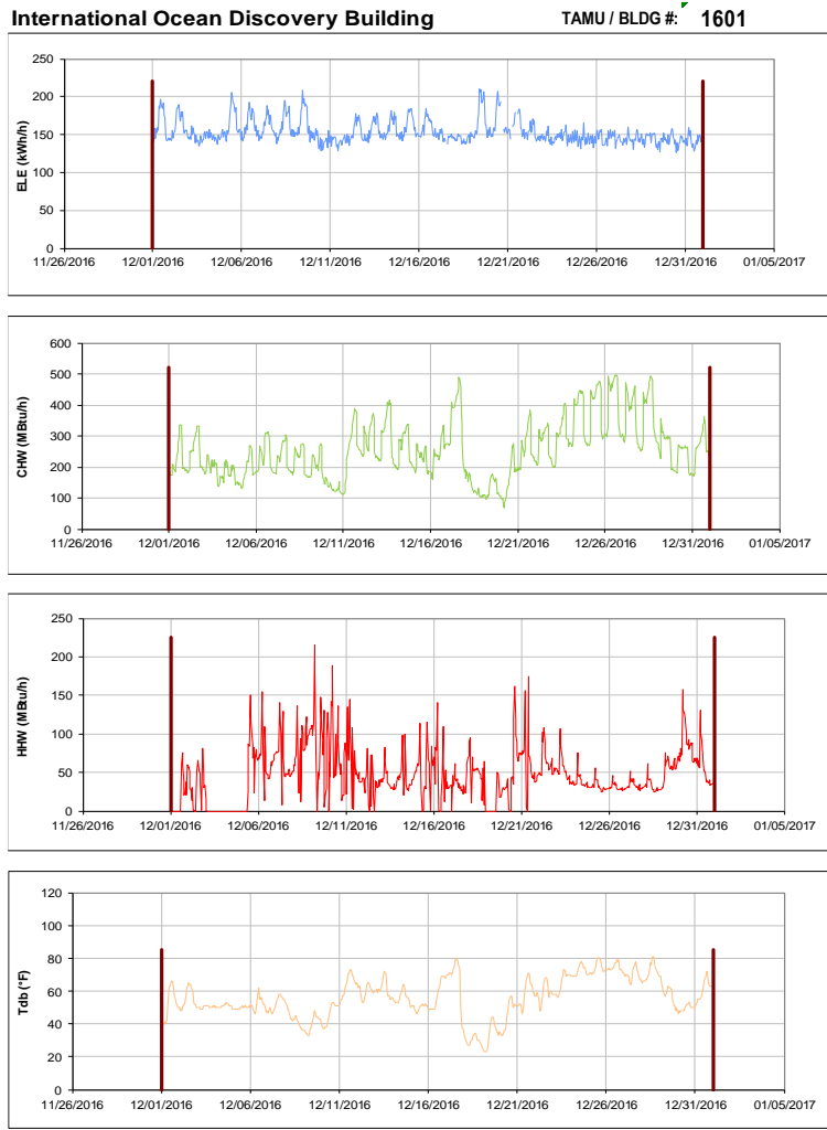
Figure III-179 Hourly Whole Building Electricity, Chilled Water, and Hot Water Consumption for International Ocean Discovery Building during the Month of December 2016 and the Corresponding Hourly Outdoor Dry Bulb Temperature for College Station, TX
