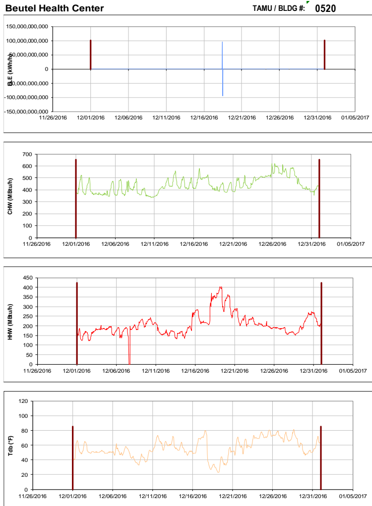
Figure III-111 Hourly Whole Building Electricity, Chilled Water, and Hot Water Consumption for Beutel Health Center during the Month of December 2016 and the Corresponding Hourly Outdoor Dry Bulb Temperature for College Station, TX
