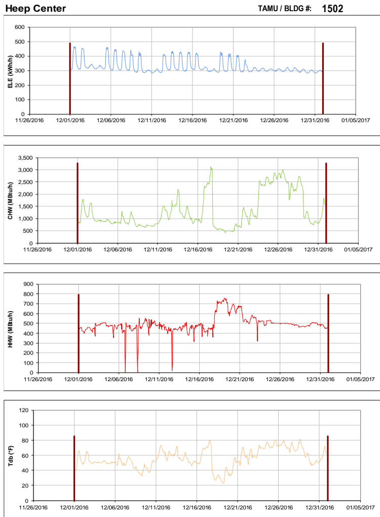
Figure III-149 Hourly Whole Building Electricity, Chilled Water, and Hot Water Consumption for Heep Center during the Month of December 2016 and the Corresponding Hourly Outdoor Dry Bulb Temperature for College Station, TX
