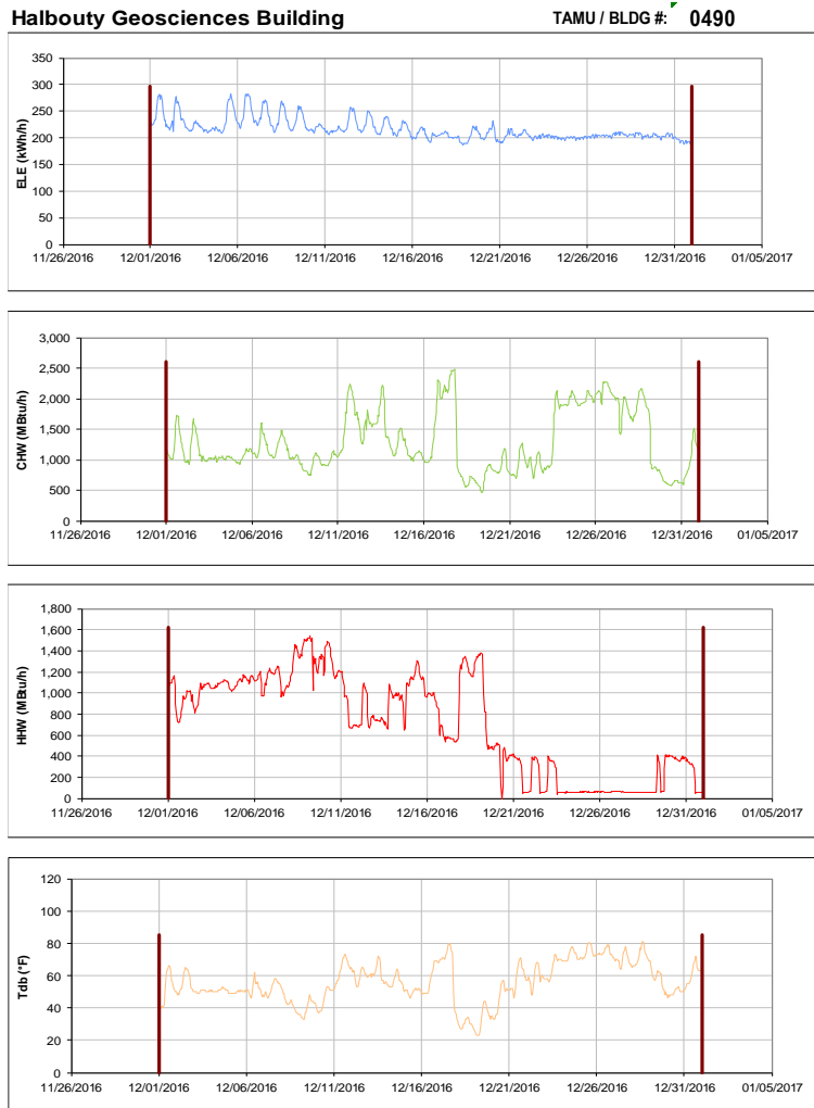
Figure III-97 Hourly Whole Building Electricity, Chilled Water, and Hot Water Consumption for Halbutoy Geosciences Building during the Month of December 2016 and the Corresponding Hourly Outdoor Dry Bulb Temperature for College Station, TX
