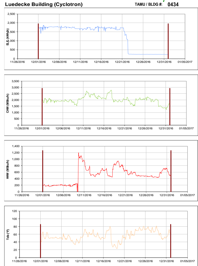
Figure III-56 Hourly Whole Building Electricity, Chilled Water, and Hot Water Consumption for Luedecke Building (Cyclotron) during the Month of December 2016 and the Corresponding Hourly Outdoor Dry Bulb Temperature for College Station, TX
