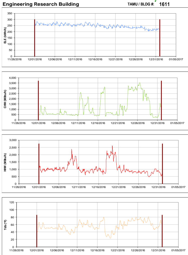
Figure III-185 Hourly Whole Building Electricity, Chilled Water, and Hot Water Consumption for Engineering Research Building during the Month of December 2016 and the Corresponding Hourly Outdoor Dry Bulb Temperature for College Station, TX
