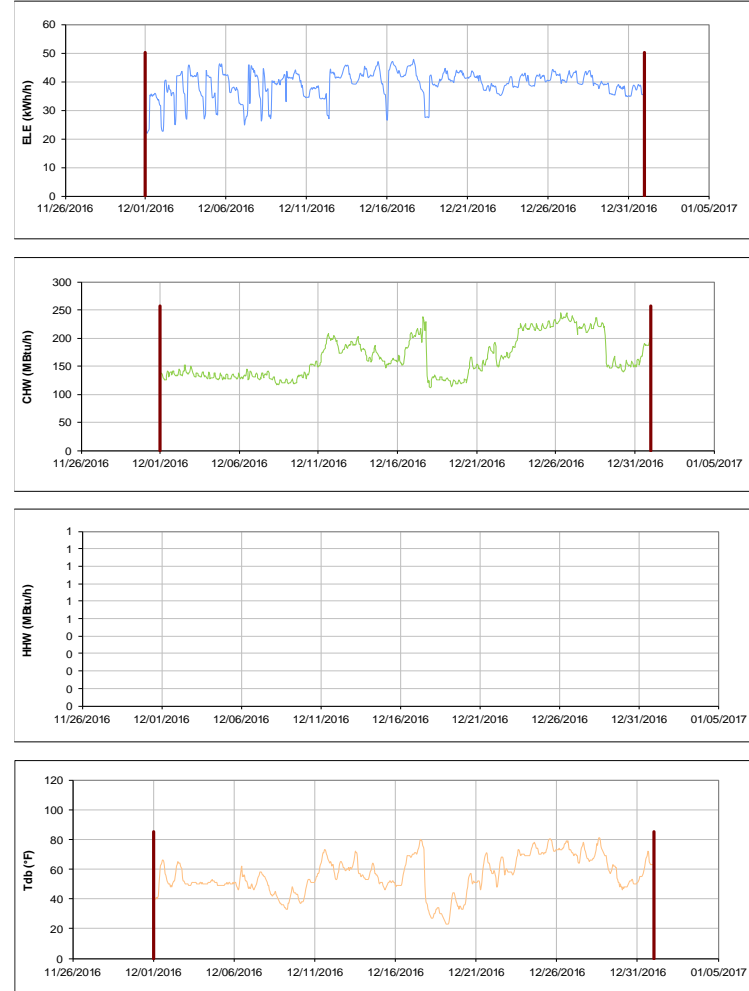
Figure III-122 Hourly Whole Building Electricity, Chilled Water, and Hot Water Consumption for Entomology Research Lab during the Month of December 2016 and the Corresponding Hourly Outdoor Dry Bulb Temperature for College Station, TX
