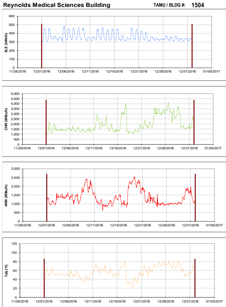
Figure III-151 Hourly Whole Building Electricity, Chilled Water, and Hot Water Consumption for Reynolds Medical Sciences Building during the Month of December 2016 and the Corresponding Hourly Outdoor Dry Bulb Temperature for College Station, TX
