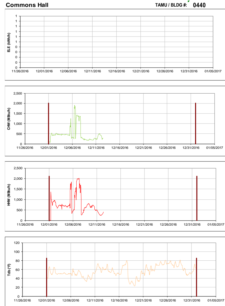
Figure III-52 Hourly Whole Building Electricity, Chilled Water, and Hot Water Consumption for Commons Hall during the Month of December 2016 and the Corresponding Hourly Outdoor Dry Bulb Temperature for College Station, TX
