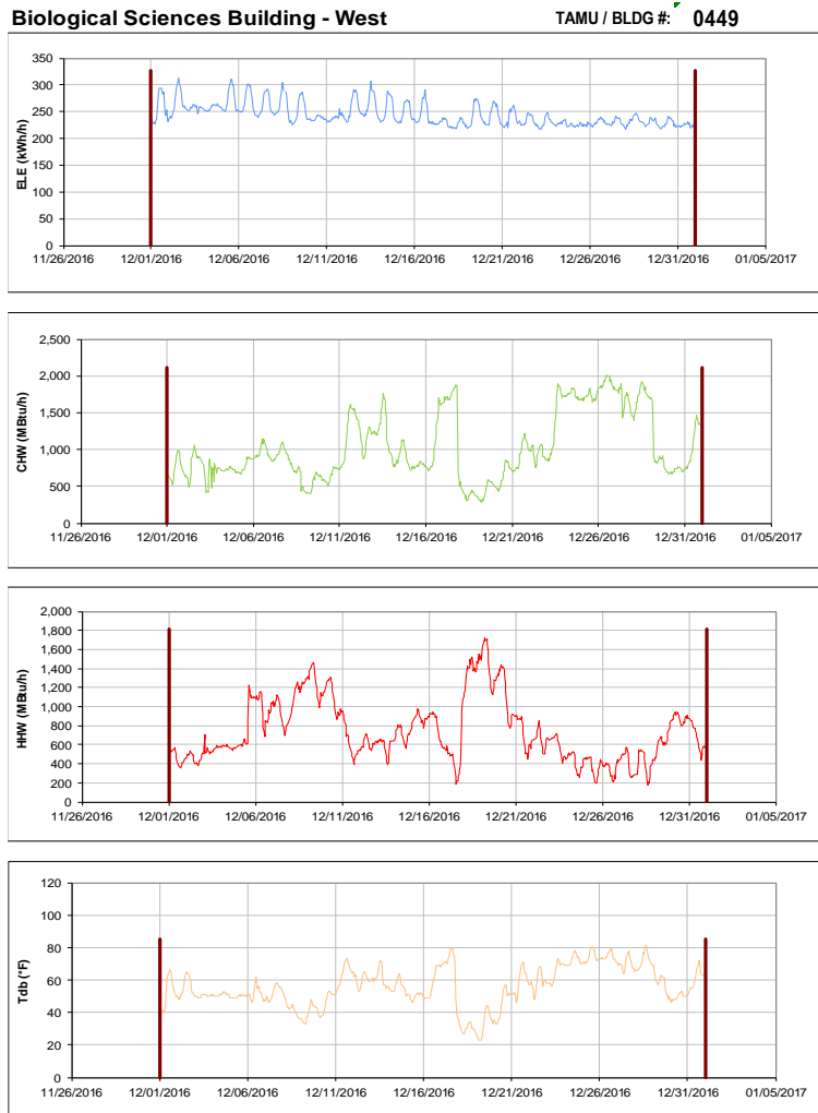
Figure III-71 Hourly Whole Building Electricity, Chilled Water, and Hot Water Consumption for Biological Sciences Building - West during the Month of December 2016 and the Corresponding Hourly Outdoor Dry Bulb Temperature for College Station, TX
