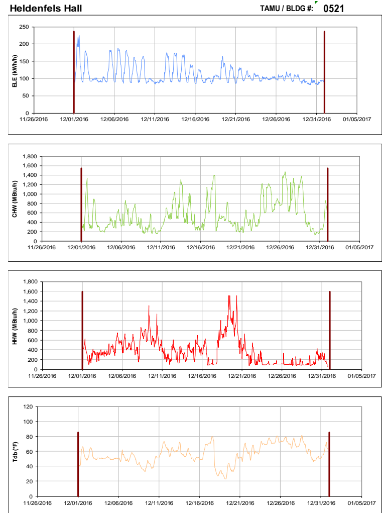
Figure III-112 Hourly Whole Building Electricity, Chilled Water, and Hot Water Consumption for Heldenfels Hall during the Month of December 2016 and the Corresponding Hourly Outdoor Dry Bulb Temperature for College Station, TX
