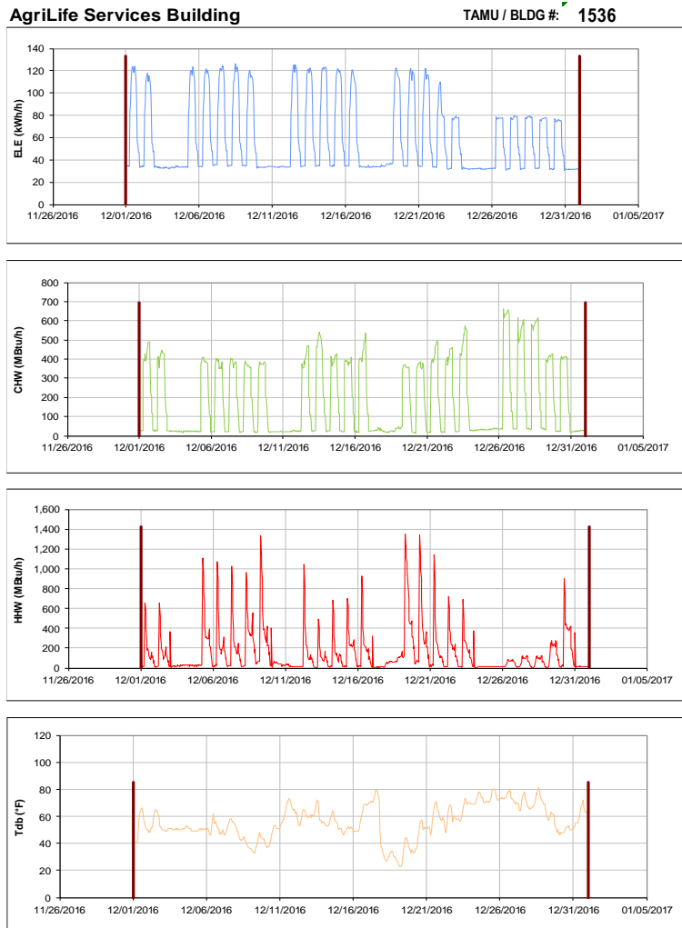
Figure III-165 Hourly Whole Building Electricity, Chilled Water, and Hot Water Consumption for AgriLife Services Building during the Month of December 2016 and the Corresponding Hourly Outdoor Dry Bulb Temperature for College Station, TX
