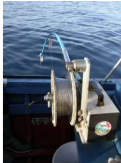
Electric reel lifting the handline
