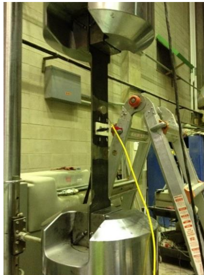
Figure 5. Fatigue load test setup
