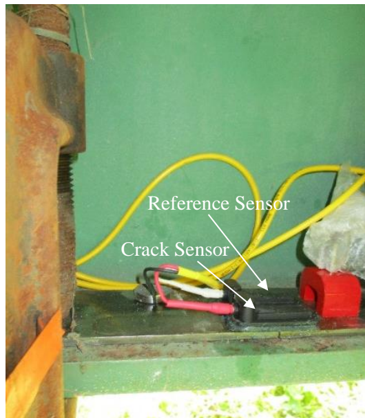
(b) Sensors on the sacrificial specimen
