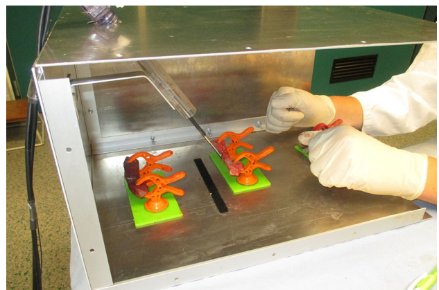
Fig. 1 Experimental setup of the box trainer. The participant stands on the left for holding the grasper, and the instructor on the right for placing the tissues in front of the grasper tip
