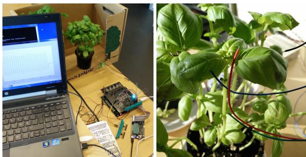
(a) Mecobo board connected to Basil plant setup. (b) Basil needle electrodes setup.
