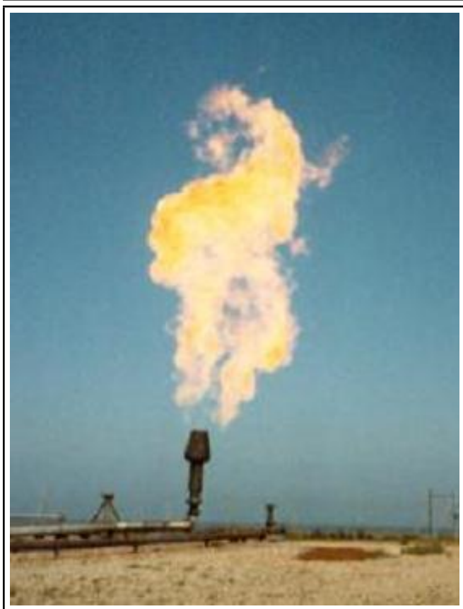
Figure 2. An operating Coanda flare.
