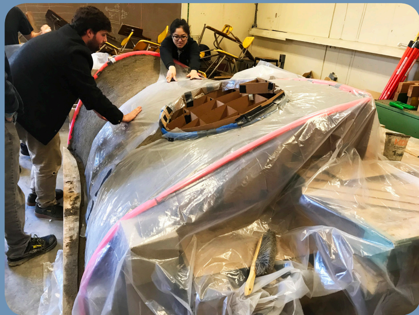
APPLICATION OF PLASTIC MEMBRANE
