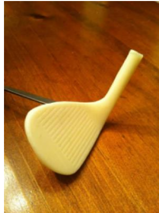
Figure 6: 3D Printed Model of Scanned Wedge
