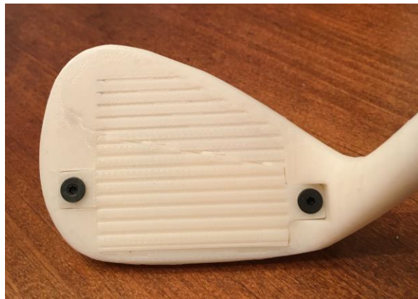
Figure 10: Plastic Assembly of Final Wedge and Insert
