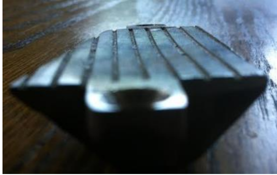
Figure 15: Prototype Insert Plastic Deformation
