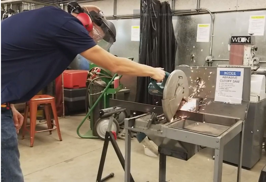
Figure 16: Oleg cutting the steel plates to length on the abrasive cutoff saw.
