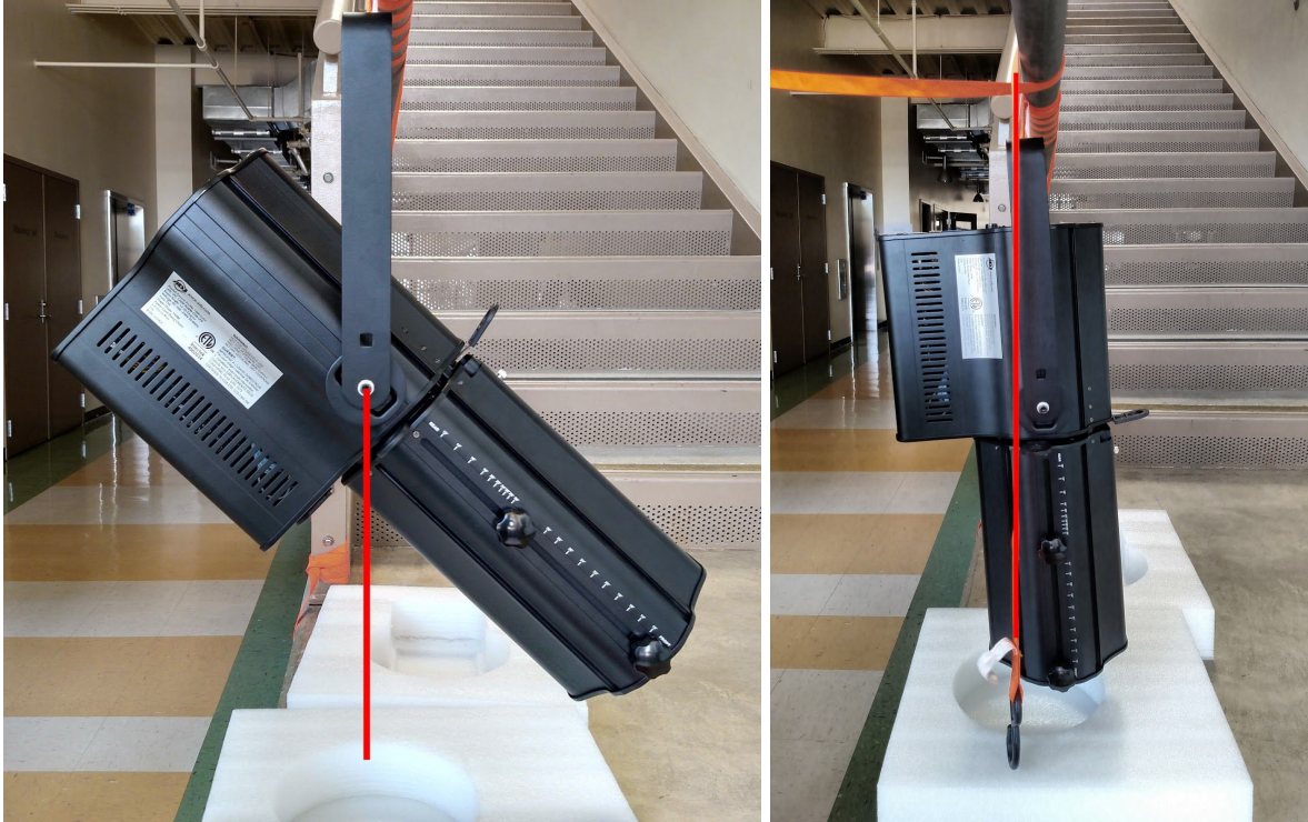
Figure 14: Suspended test to determine the location of the spotlight's center of gravity.
