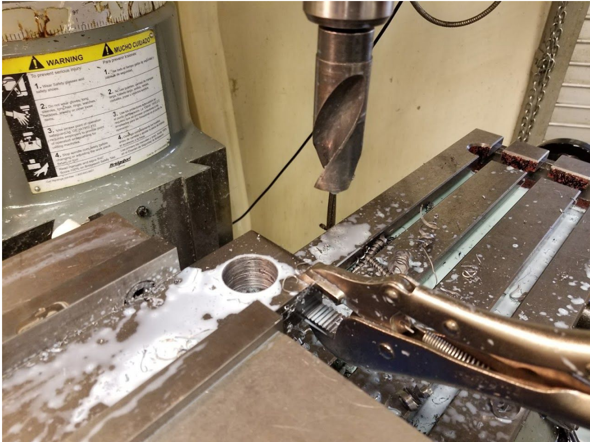
Figure 17: Boring through the steel plates with a large drill bit.
