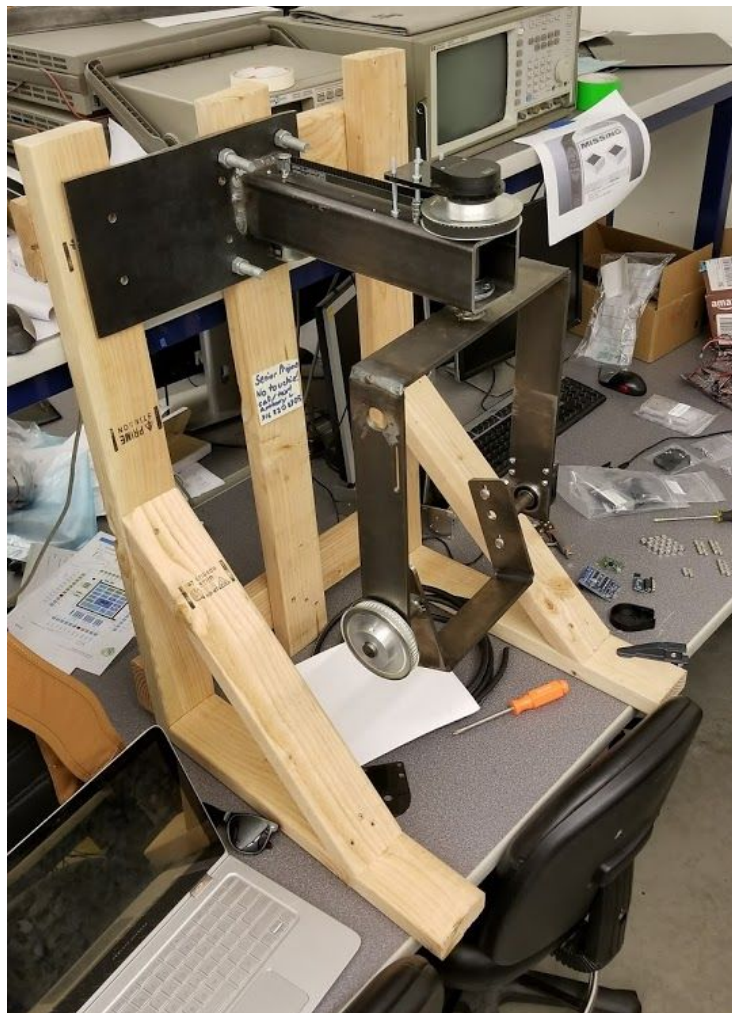
Figure 24: Temporary test setup during the coding and controller tuning phase of the project.
