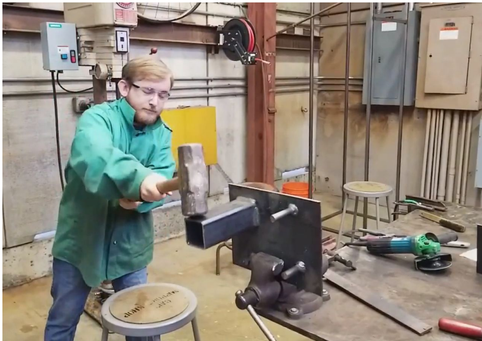
Figure 15: Anthony performing destructive testing on a sample weld joint.
