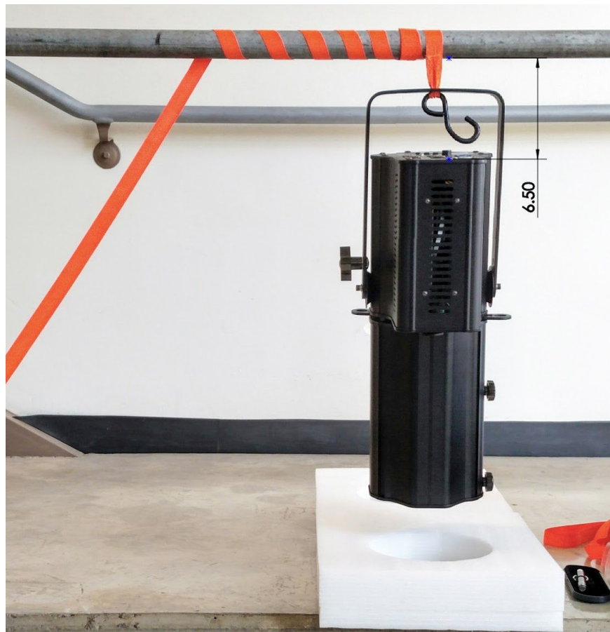
Figure 15: Suspended swinging test setup.
