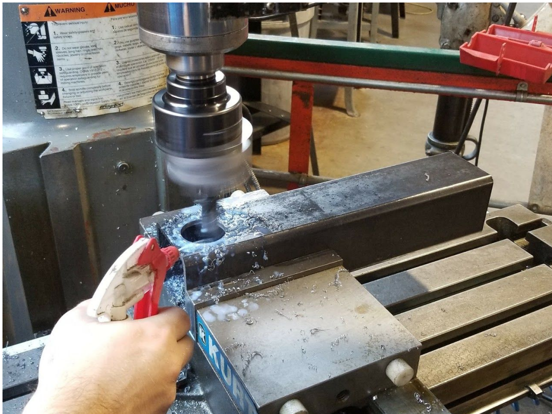
Figure 14: Using a fly cutter to widen the bearing holes.
