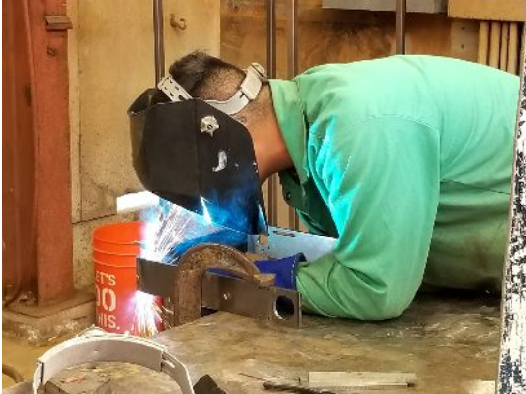
Figure 18: Welding the corner joints on the Y-bracket.
