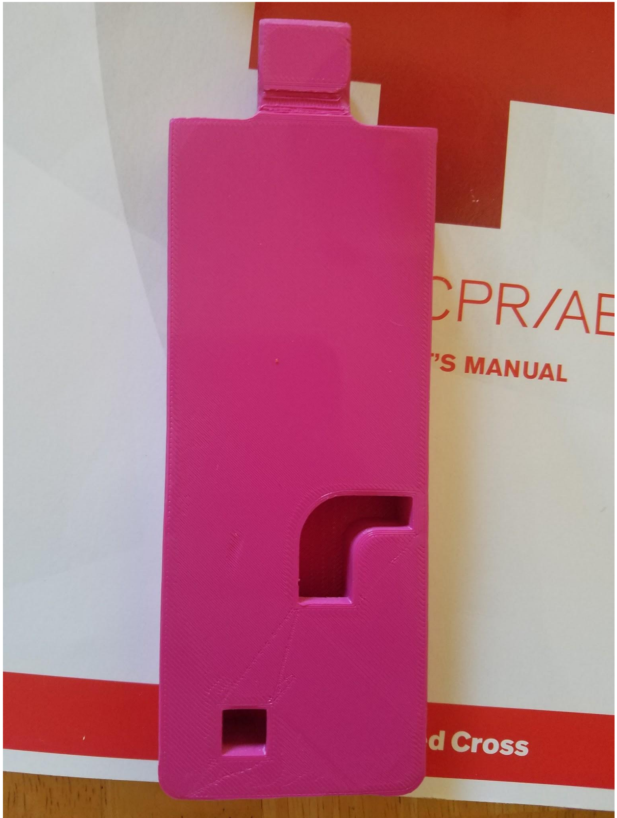
Figure 23: Photo of the completed printed slide valve.
