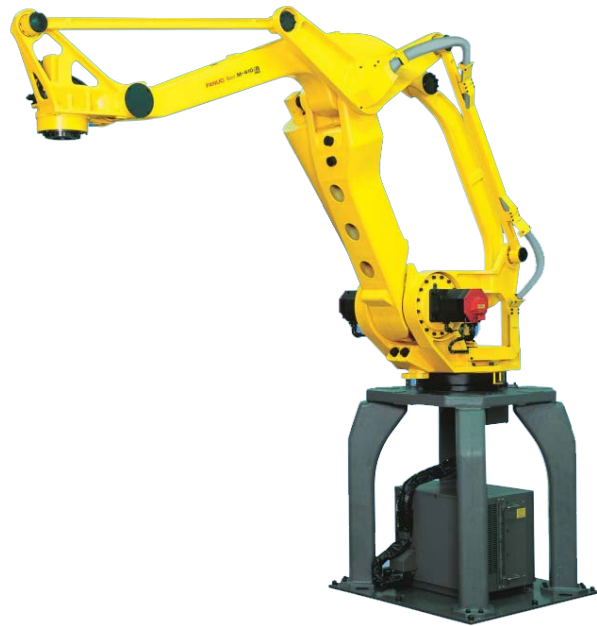
Figure 2-7 | A Fanuc arm using linkages to transfer rotational motion from motors fixed at the robot's base (FANUC America Corporation, 2017)
