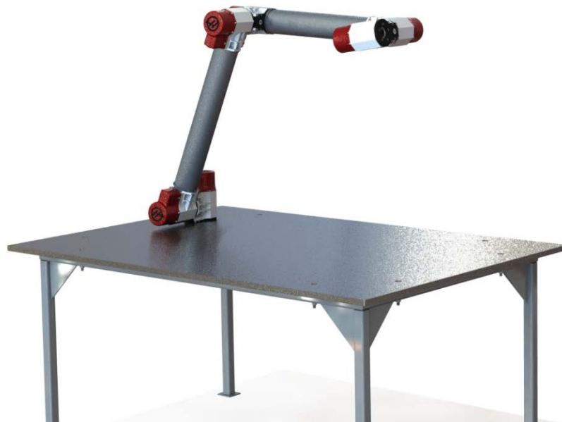
Figure 4-5 | Pictured here is a sample configuration of our rotary joint with arm tube segments to create a material handling robot.
