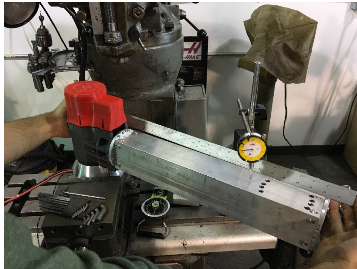
Figure 7-1 Spring Constant of Joint Testing
