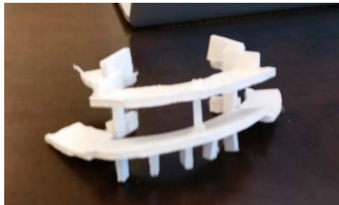
Figure 4.2b: Basic foam core model of the Rim Seal Mounted Clamping Tool.
