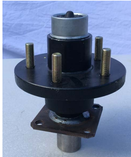
Figure 6.3.1. Trailer Hub in as-ordered condition.
