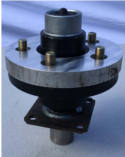
Figure 6.3.2. Hub Spacer on top of the Trailer Hub (longer studs not shown).
