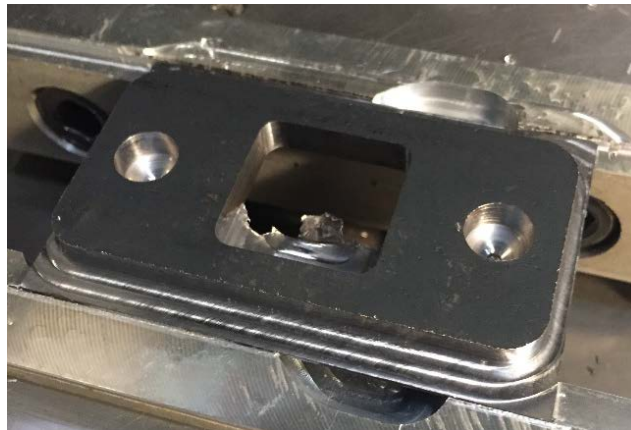
Figure 6.2.1. Base Plate after Op. 1 of machining.
