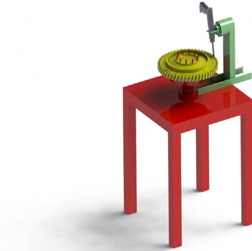
Figure 4.6b: A preliminary rendering of the table based tool with rotating disk mount.
