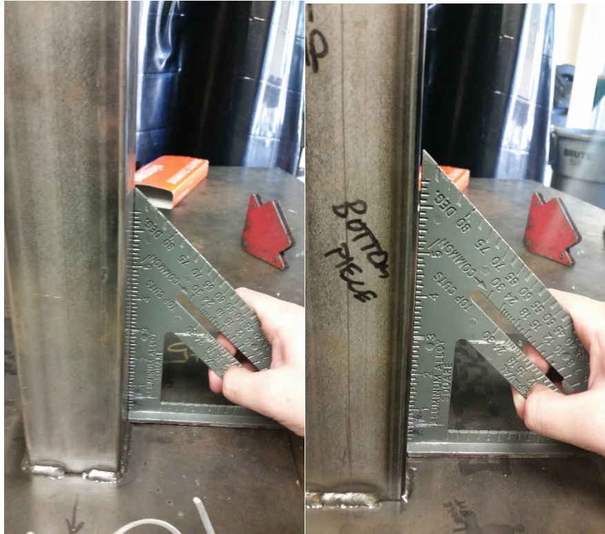
Figure 6.1.4. Perpendicularity measurements on the vertical tube.
