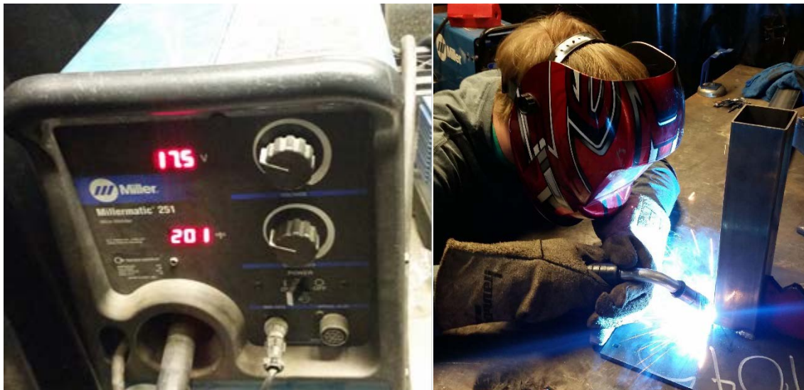
Figure 6.1.3. Performing stitch welds
