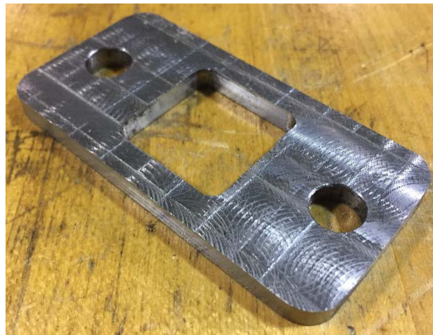
Figure 6.2.2. Finished Locking Mechanism Base Plate.
