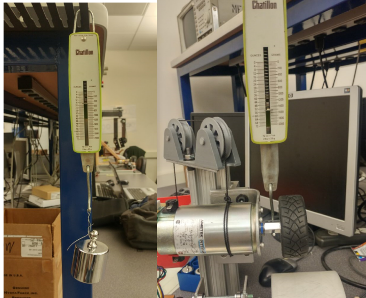
Figure 6.4 Fish scale calibration with 500g weight (left) and radial load measurement (right)
