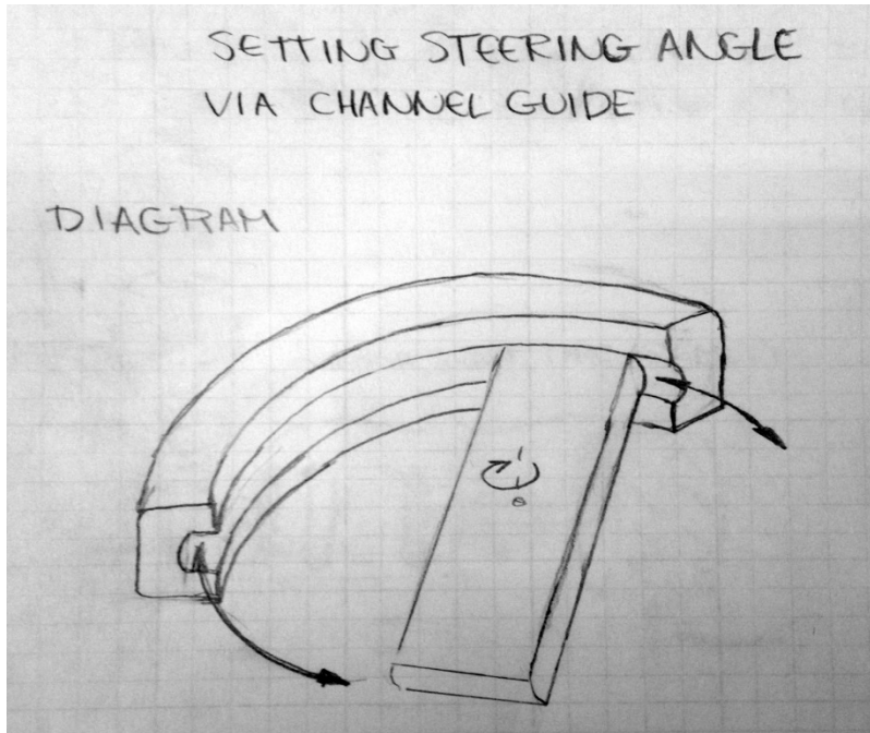
Figure F.5 Hand sketch diagram illustrating the slot guide concept for applying the steering angle
