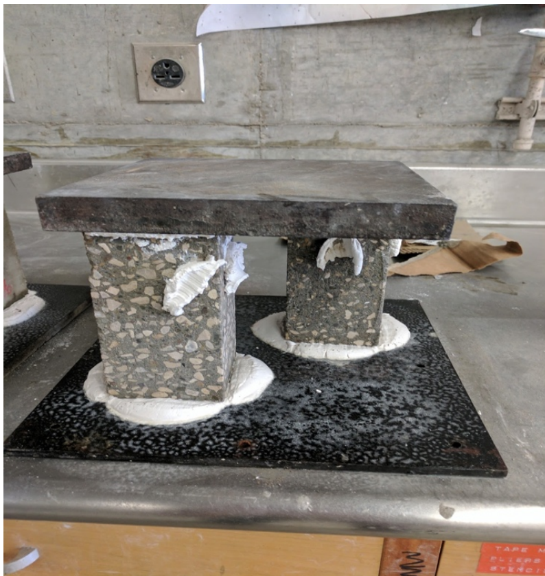
Figure 6: Filled then Cut CMU Test Specimen
