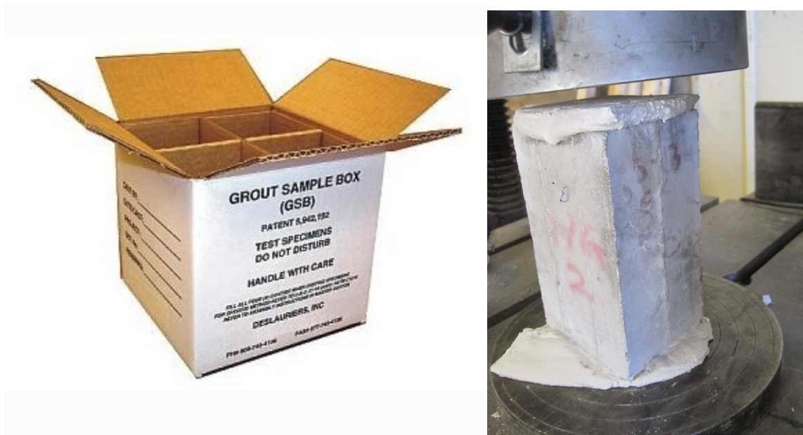
Figure 7: Masonry Grout Sample Box and Test Specimen
