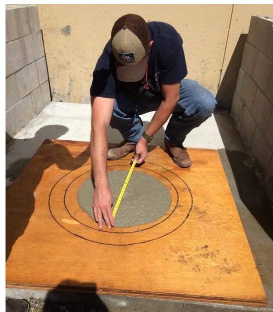
Figure 4B: Slump Flow Test
